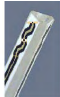
Figure 3.3 Probe Thick-Film Technique
