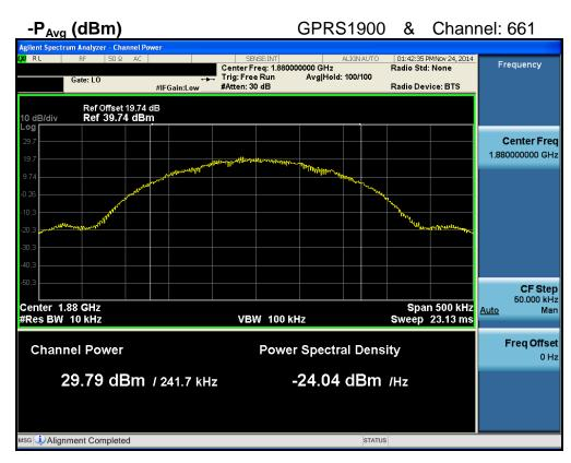
PAPR (dB) =  $P_{Pk}$  (dBm) -  $P_{Avg}$  (dBm) = 30.16dBm - 29.79dBm = 0.37 dB
