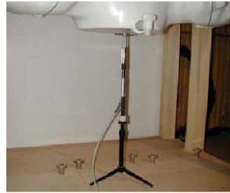
Figure 11.1 Dipole Verification Test Setup Diagram & Photo
