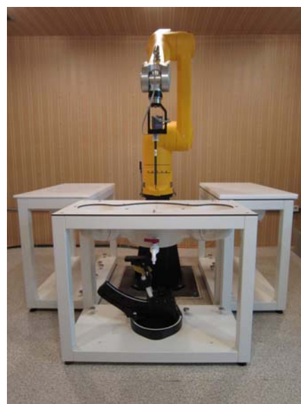
Figure 2.2 DASY5 Test System
