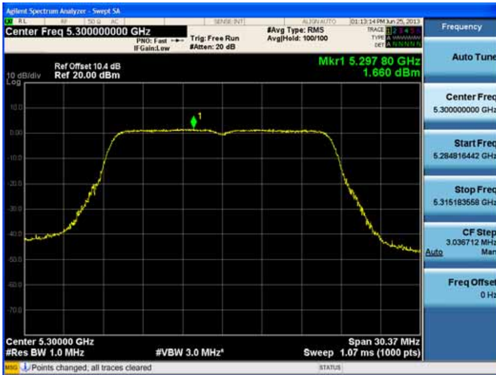
Power Spectral Density (802.11a-CH 60)
