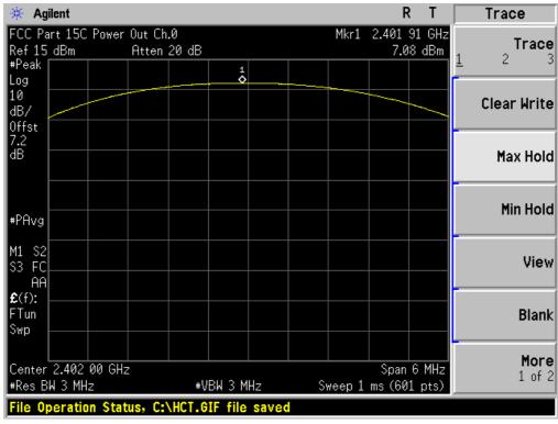
Test Plots ( $\pi/4DQPSK$ ) Peak Power (Mid-CH)
