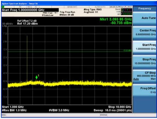
Test Plots ( $\pi$ /4DQPSK) - 1 GHz - 10 GHz (RBW:1 MHz, VBW: 3 MHz) Spurious Emission (Mid-CH)
