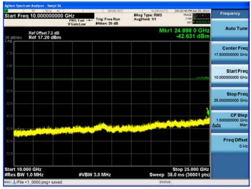
Test Plots (GFSK) - 10 GHz - 25 GHz (RBW:1 MHz, VBW: 3 MHz) Spurious Emission (Mid-CH)
