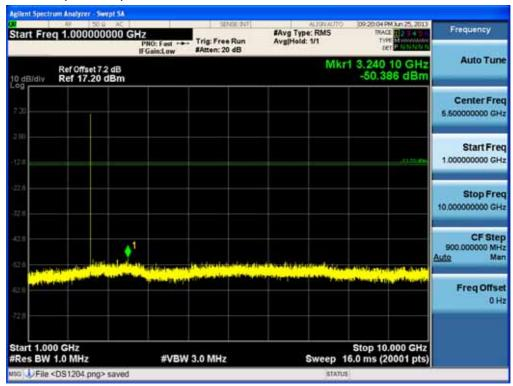
Test Plots (GFSK) - 1 GHz - 10 GHz (RBW:1 MHz, VBW: 3 MHz) Spurious Emission (Mid-CH)
