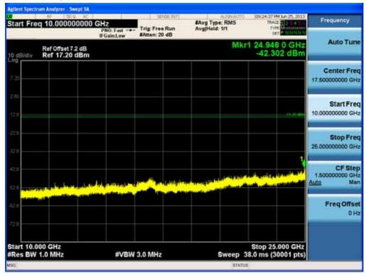
Test Plots (8DPSK) - 10 GHz - 25 GHz (RBW:1 MHz, VBW: 3 MHz) Spurious Emission (Low-CH)
