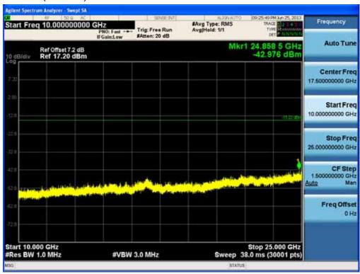
Test Plots ( $\pi$ /4DQPSK) - 10 GHz - 25 GHz (RBW:1 MHz, VBW: 3 MHz) Spurious Emission (Mid-CH)
