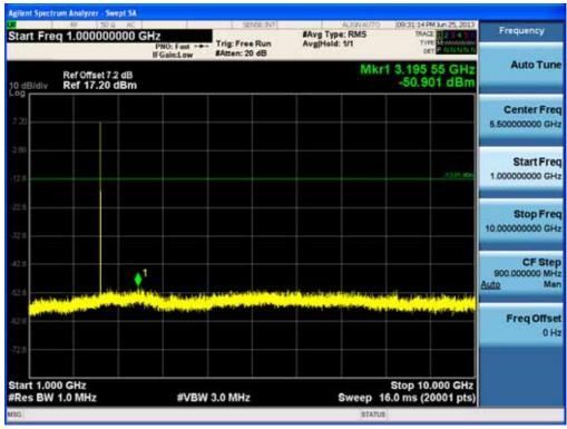
Test Plots (8DPSK) - 1 GHz - 10 GHz (RBW:1 MHz, VBW: 3 MHz) Spurious Emission (High-CH)
