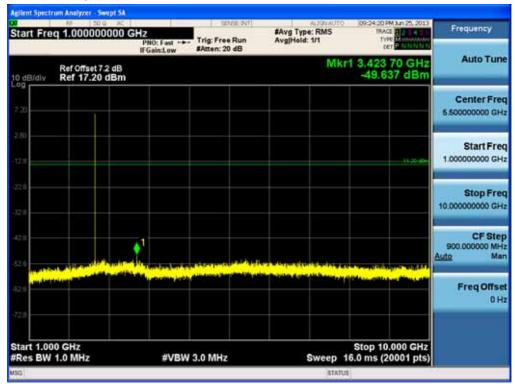
Test Plots (8DPSK) - 1 GHz - 10 GHz (RBW:1 MHz, VBW: 3 MHz) Spurious Emission (Low-CH)
