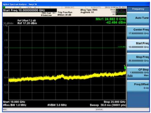
Test Plots (8DPSK) - 10 GHz - 25 GHz (RBW:1 MHz, VBW: 3 MHz) Spurious Emission (High-CH)
