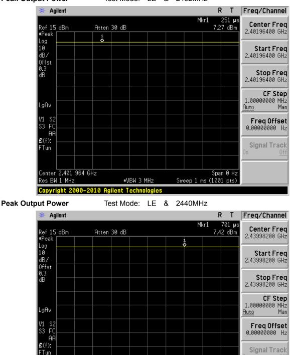
Peak Output Power Test Mode: LE & 2402MHz
