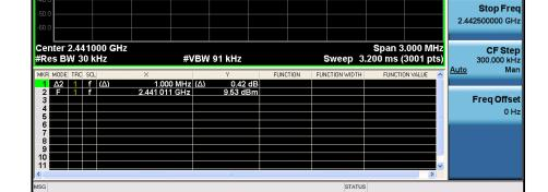
Carrier Frequency Separation (FH) <u>Hopping mode : Enable & π/4DQPSK</u>
