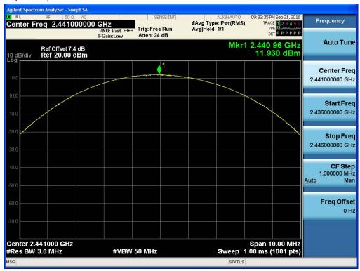
Test Plots (8DPSK) Peak Power (CH.78)
