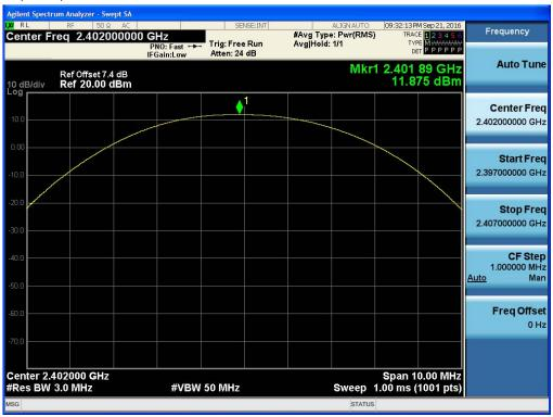
Test Plots (GFSK) Peak Power (CH.39)
