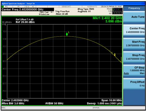
Test Plots (GFSK) Peak Power (Mid-CH)
