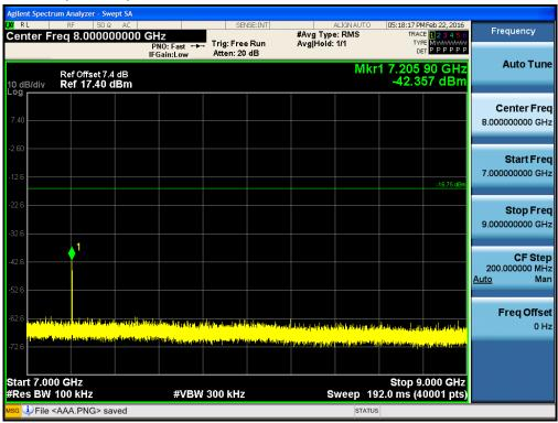
Test Plots (GFSK)- 9 GHz - 11 GHz Spurious Emission (Low-CH)
