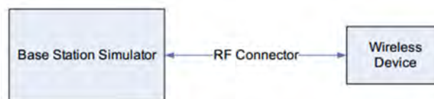
Figure 9.1 Power Measurement Setup
