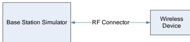
Figure 9-3 Power Measurement Setup
