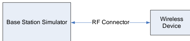
Figure 9-2 Power Measurement Setup
