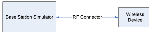
Figure 9-1 Power Measurement Setup
