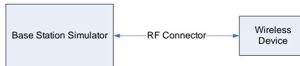
Figure 9-4 Power Measurement Setup
