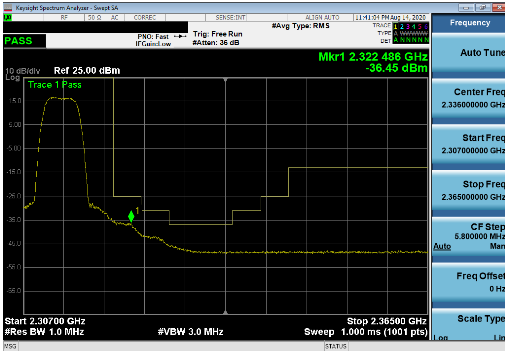
Plot 7-417. Extended Upper Band Edge Plot (LTE Band 30 - 5MHz QPSK – Full RB Configuration)
