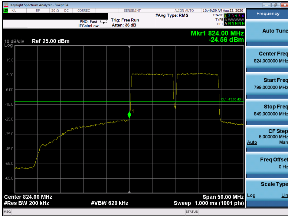
Plot 7-430. Lower Band Edge Plot (LTE Band 5 – 10MHz BW QPSK – Full RB Configuration)
