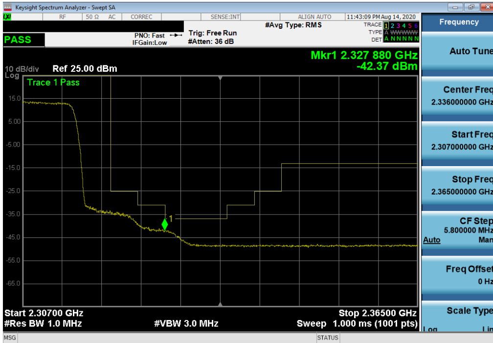
Plot 7-421. Extended Upper Band Edge Plot (LTE Band 30 - 10MHz QPSK – Full RB Configuration)
