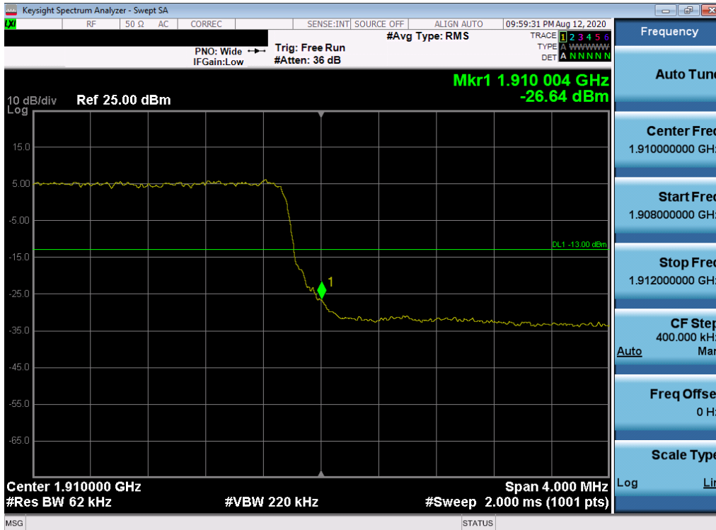
Plot 7-392. Upper Band Edge Plot (LTE Band 2 - 5MHz QPSK – Full RB Configuration)
