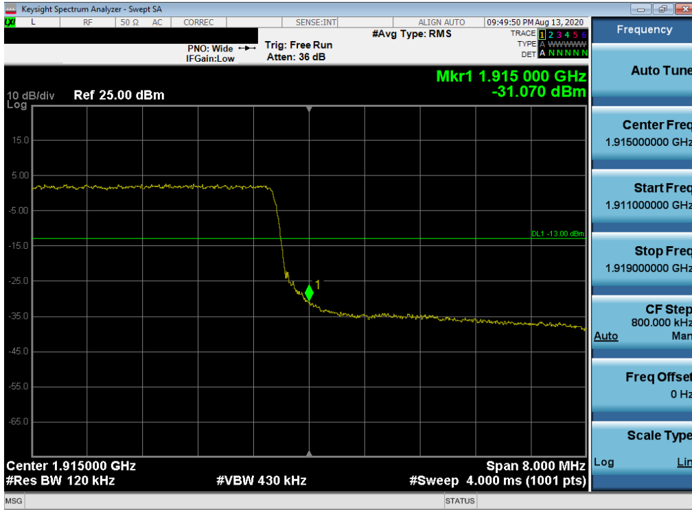
Plot 7-400. Upper Band Edge Plot (LTE Band 25 - 10MHz QPSK – Full RB Configuration)
