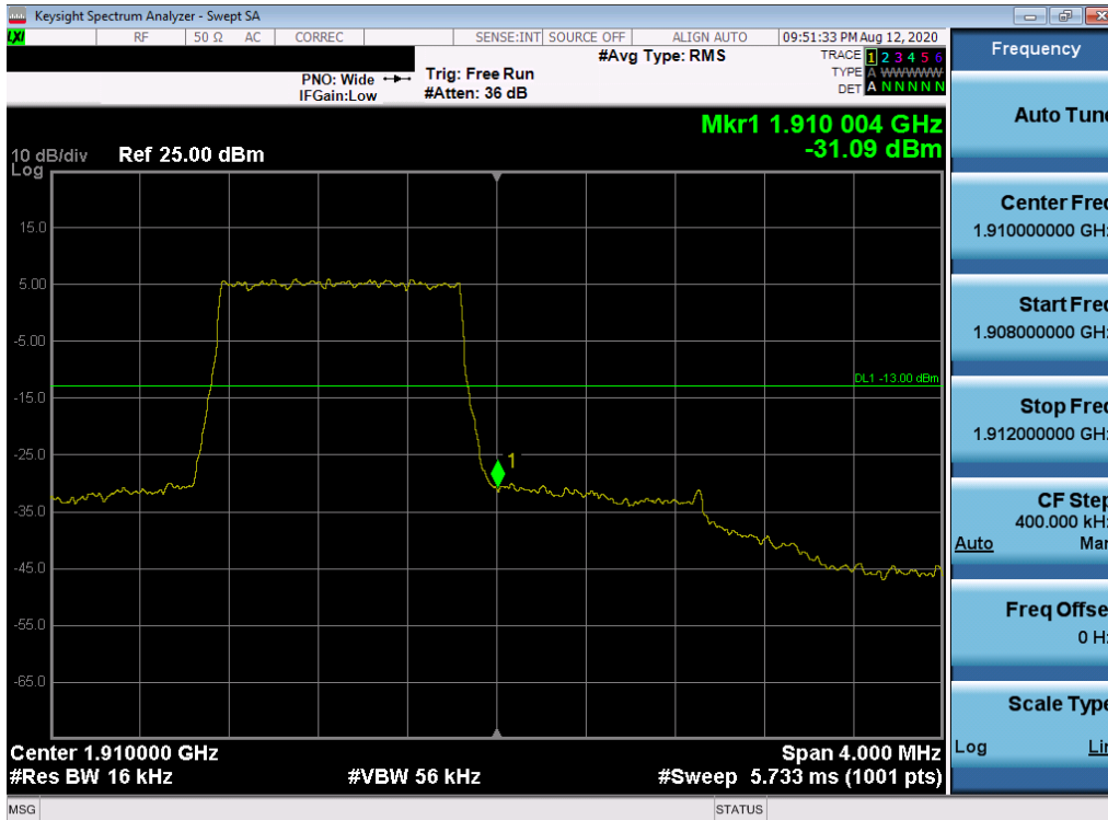
Plot 7-380. Upper Band Edge Plot (LTE Band 2 – 1.4MHz QPSK – Full RB Configuration)
