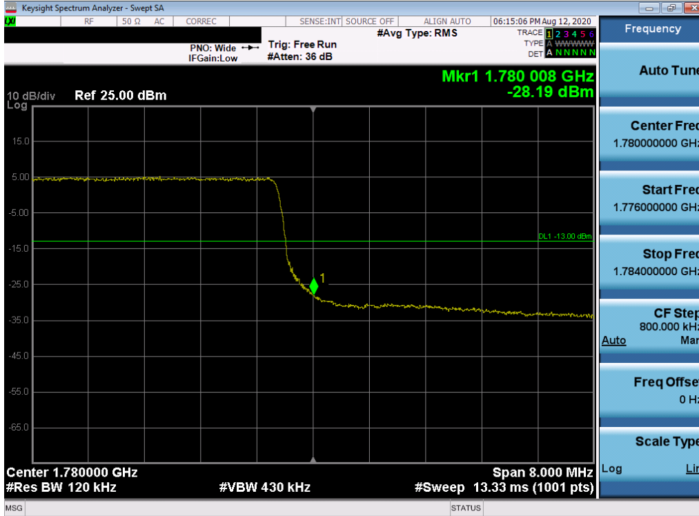
Plot 7-364. Upper Band Edge Plot (LTE Band 66 - 10MHz QPSK – Full RB Configuration)
