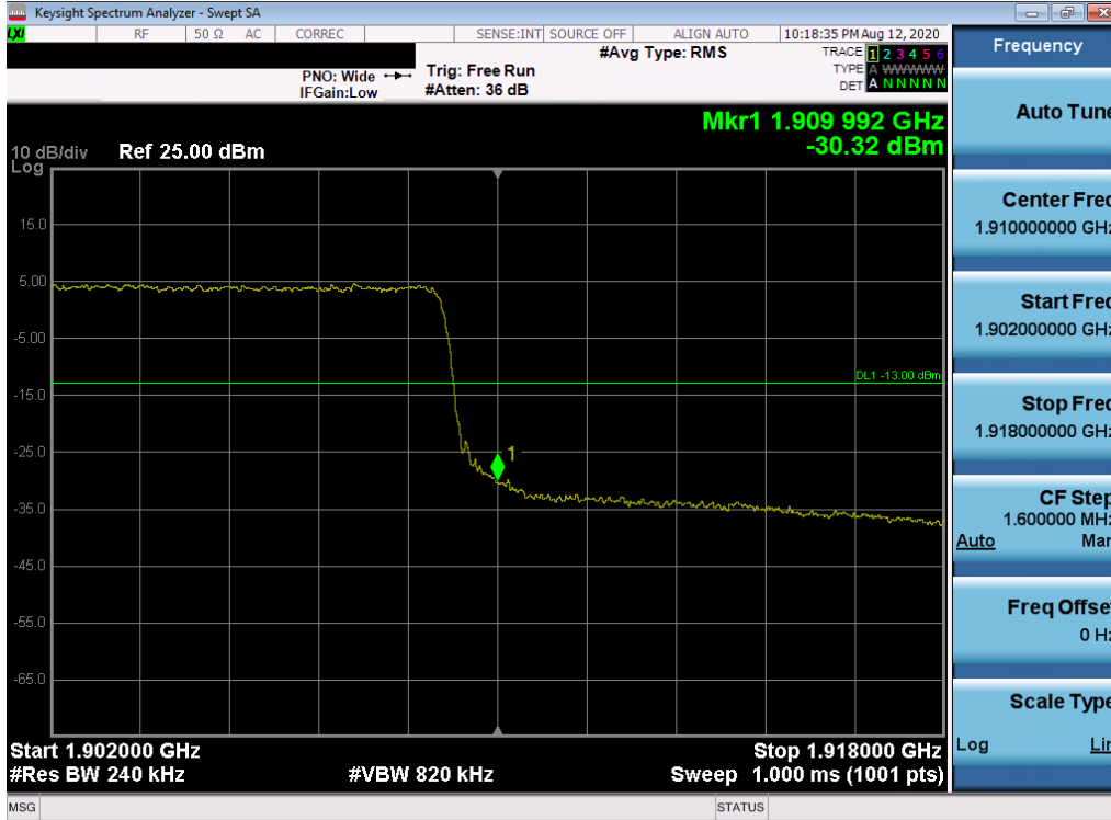
Plot 7-410. Upper Band Edge Plot (LTE Band 2 - 20MHz QPSK – Full RB Configuration)
