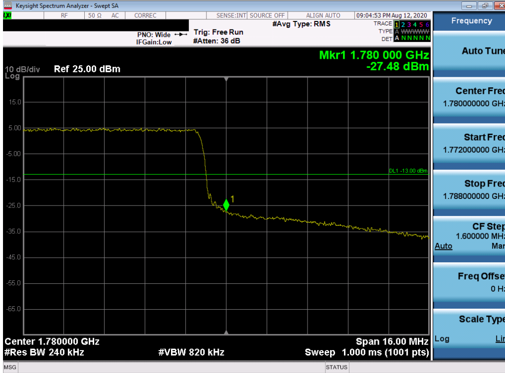
Plot 7-376. Upper Band Edge Plot (LTE Band 66 - 20MHz QPSK – Full RB Configuration)
