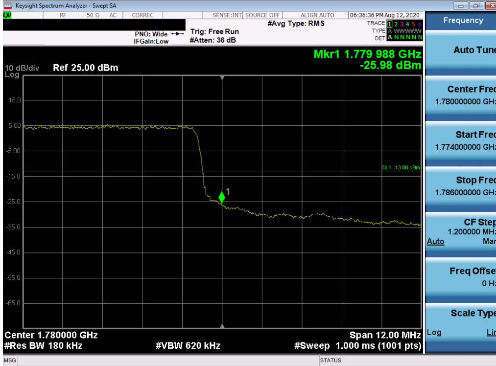
Plot 7-370. Upper Band Edge Plot (LTE Band 66 - 15MHz QPSK – Full RB Configuration)
