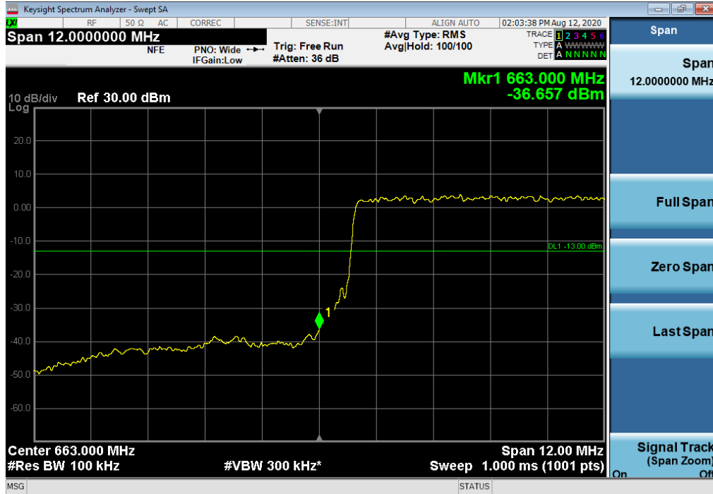
Plot 7-328. Lower Band Edge Plot (LTE Band 71 - 15MHz QPSK – Full RB Configuration)
