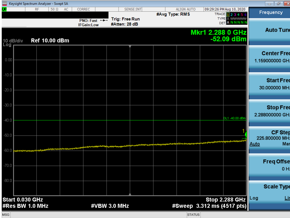
Plot 7-246. Conducted Spurious Plot (LTE Band 30 - 5MHz QPSK - RB Size 1, RB Offset 0 - High Channel)
