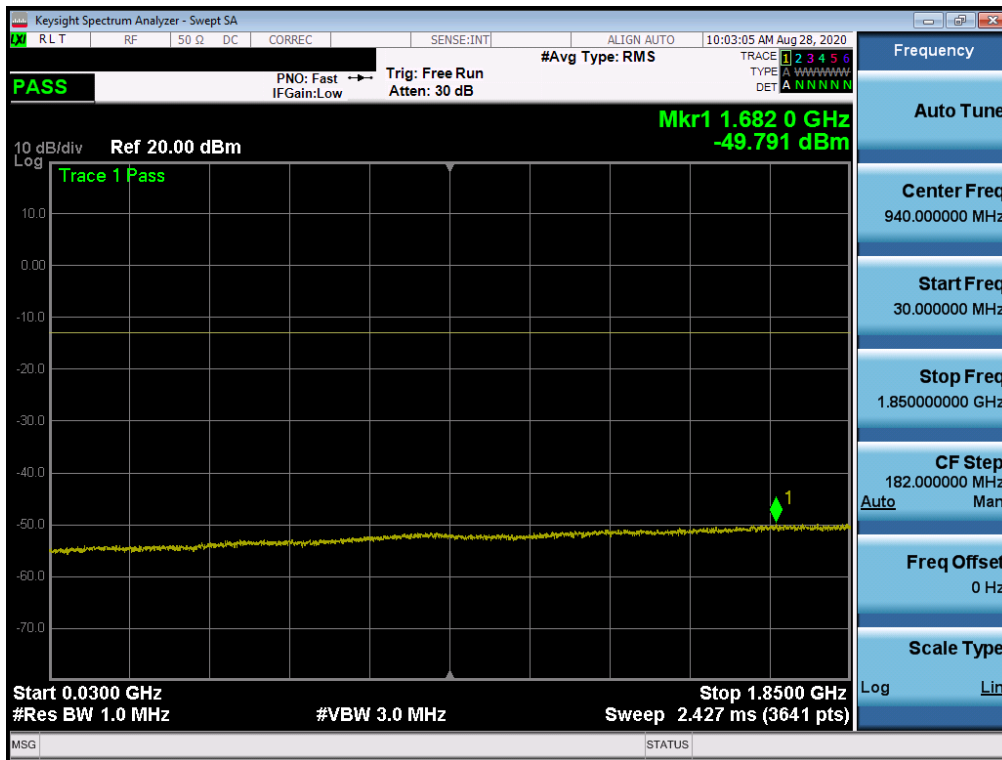
Plot 7-300. Conducted Spurious Plot (NR Band n2 - 20.0MHz - RB Size 1, RB Offset 0 - Mid Channel)
