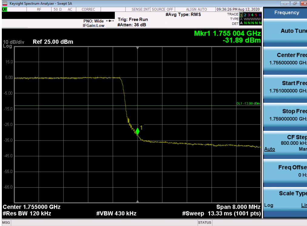
Plot 7-362. Upper Band Edge Plot (LTE Band 4 - 10MHz QPSK – Full RB Configuration)
