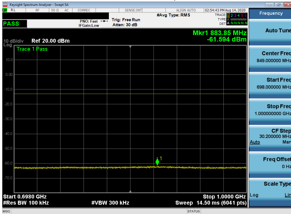
Plot 7-271. Conducted Spurious Plot (NR Band n71 - 20.0MHz - RB Size 1, RB Offset 0 - Low Channel)
