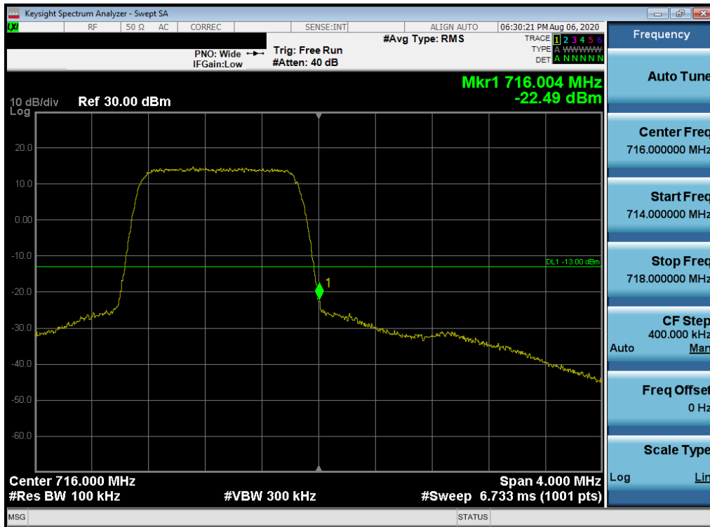
Plot 7-307. Upper Band Edge Plot (LTE Band 12 – 1.4MHz QPSK – Full RB Configuration)
