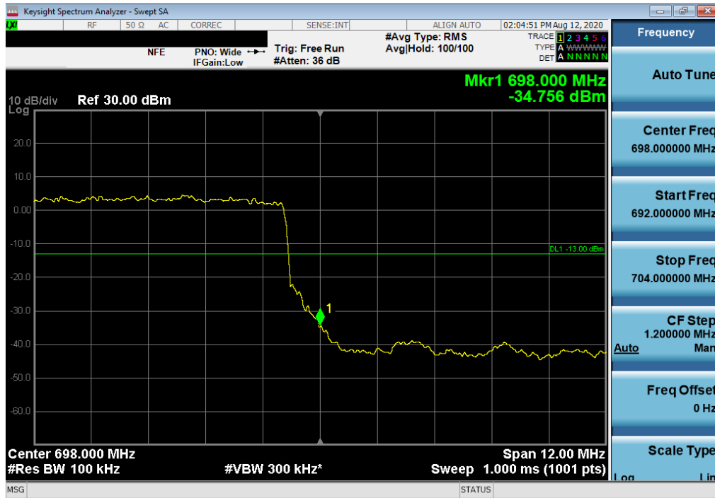
Plot 7-329. Upper Band Edge Plot (LTE Band 71 - 15MHz QPSK – Full RB Configuration)
