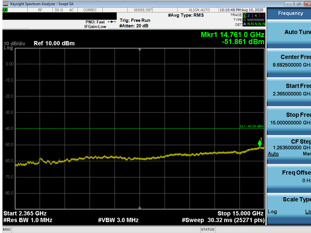
Plot 7-244. Conducted Spurious Plot (LTE Band 30 - 5MHz QPSK - RB Size 1, RB Offset 0 - Mid Channel)
