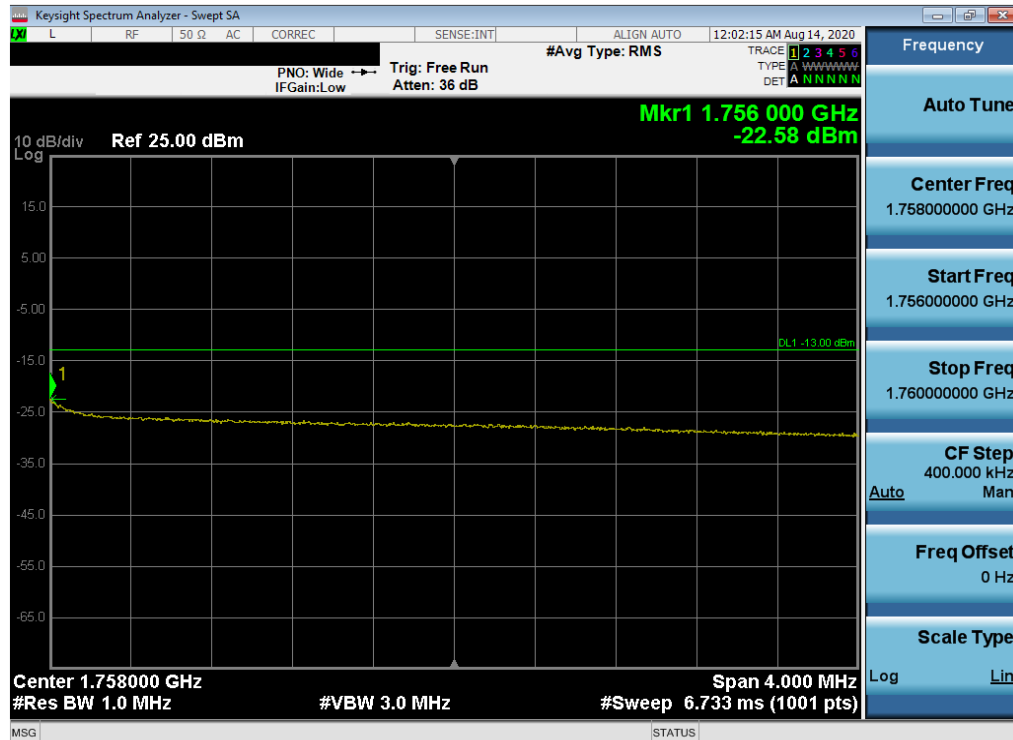
Plot 7-363. Upper Extended Band Edge Plot (LTE Band 4 - 10MHz QPSK – Full RB Configuration)
