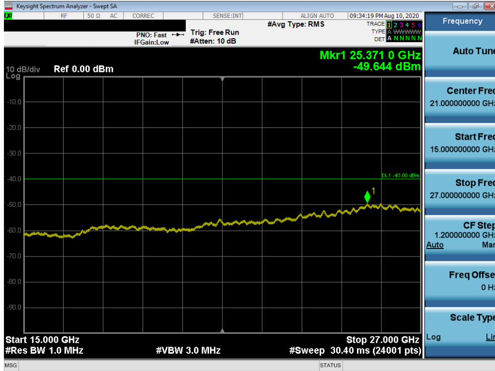
Plot 7-248. Conducted Spurious Plot (LTE Band 30 - 5MHz QPSK - RB Size 1, RB Offset 0 - High Channel)
