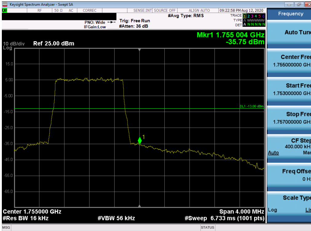
Plot 7-344. Upper Band Edge Plot (LTE Band 4 – 1.4MHz QPSK – Full RB Configuration)
