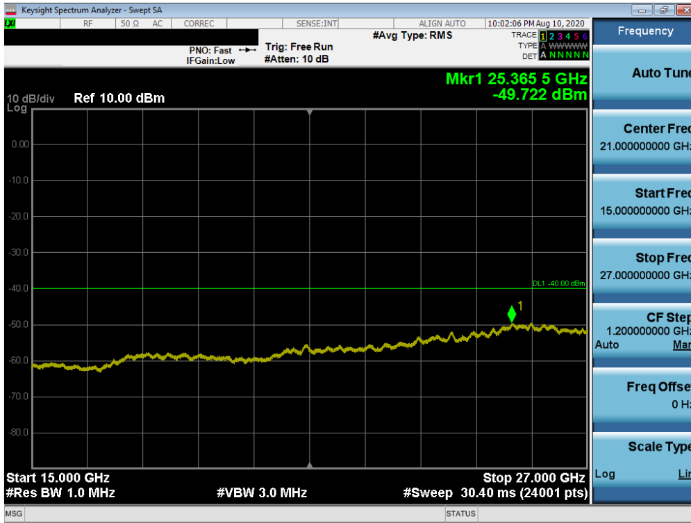
Plot 7-242. Conducted Spurious Plot (LTE Band 30 - 5MHz QPSK - RB Size 1, RB Offset 0 - Low Channel)
