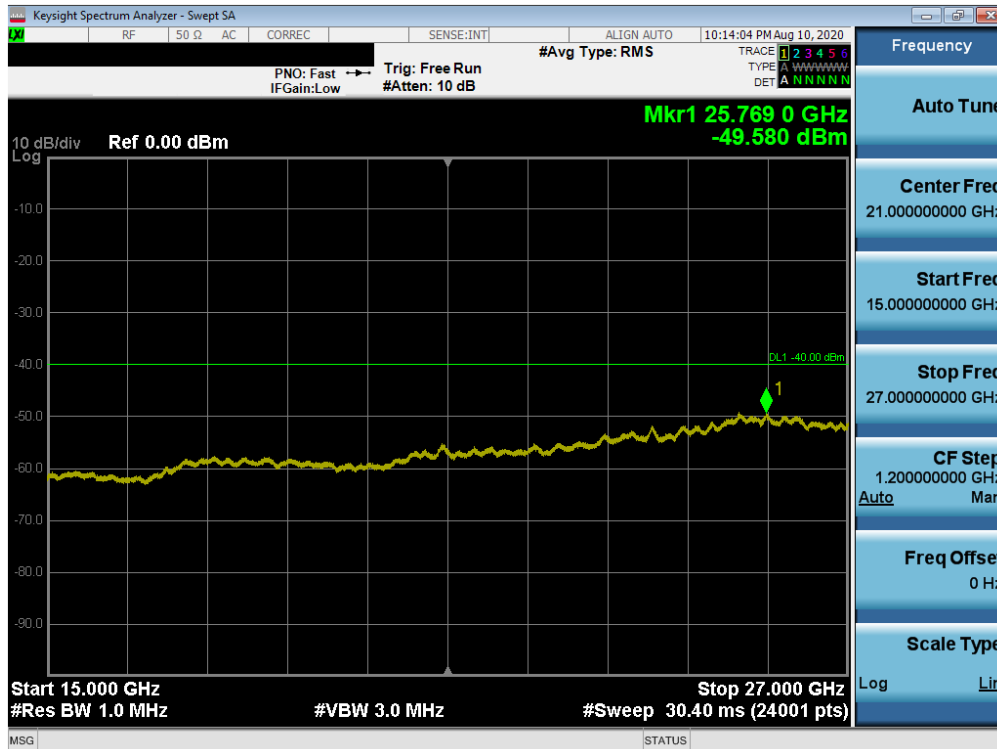
Plot 7-245. Conducted Spurious Plot (LTE Band 30 - 5MHz QPSK - RB Size 1, RB Offset 0 - Mid Channel)
