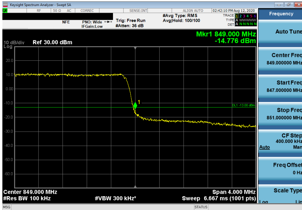
Plot 7-335. Upper Band Edge Plot (LTE Band 26/5 - 3MHz QPSK – Full RB Configuration)
