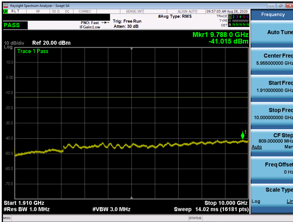
Plot 7-304. Conducted Spurious Plot (NR Band n2 - 20.0MHz - RB Size 1, RB Offset 0 - High Channel)
