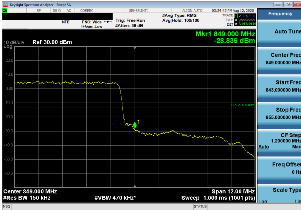
Plot 7-341. Upper Band Edge Plot (LTE Band 26 - 15MHz QPSK – Full RB Configuration)
