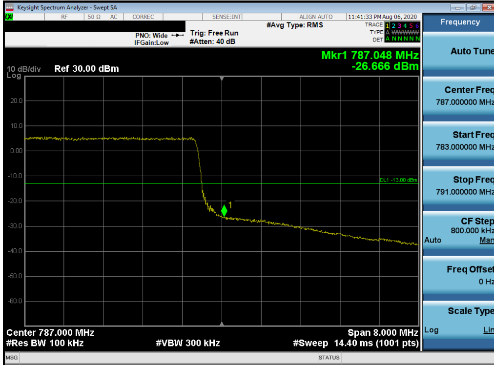
Plot 7-322. Upper Band Edge Plot (LTE Band 13 - 10MHz QPSK – Full RB Configuration)
