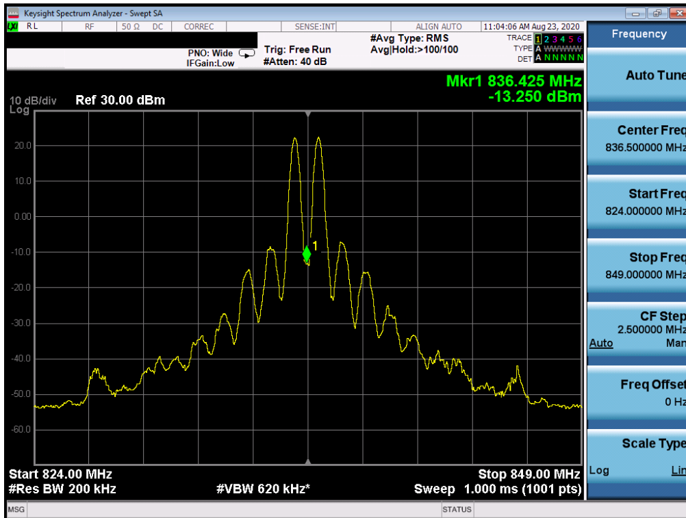
Plot 7-215. Conducted Spurious Plot (ULCA LTE Band 5 – (10 + 10)MHz QPSK – PCC 1/49 SCC 1/0 - Mid Channel)
