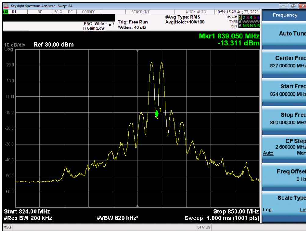
Plot 7-219. Conducted Spurious Plot (ULCA LTE Band 5 – (10 + 10)MHz QPSK – PCC 1/0 SCC 1/49 - High Channel)
