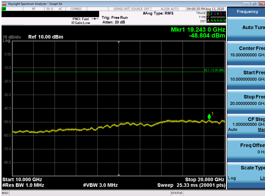
Plot 7-224. Conducted Spurious Plot (LTE Band 66/4 - 20MHz QPSK - RB Size 1, RB Offset 0 - Low Channel)
