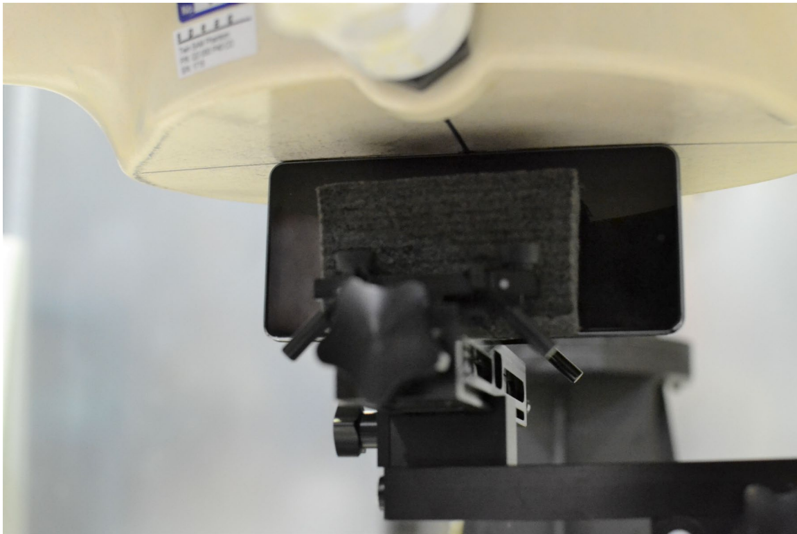
SAR Test Setup Photo 19 – Left Edge at 0 mm
