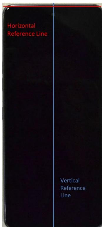
SAR Test Setup Photo 20 – Horizontal and Vertical Lines
