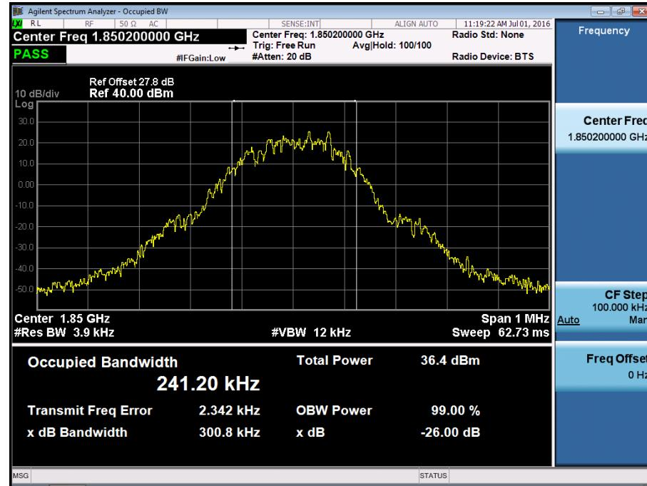
■ GSM1900 MODE (661 CH.) Occupied Bandwidth
