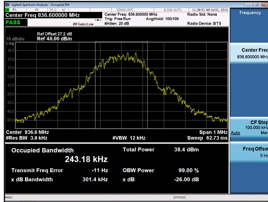
■ GSM850 MODE (251 CH.) Occupied Bandwidth
