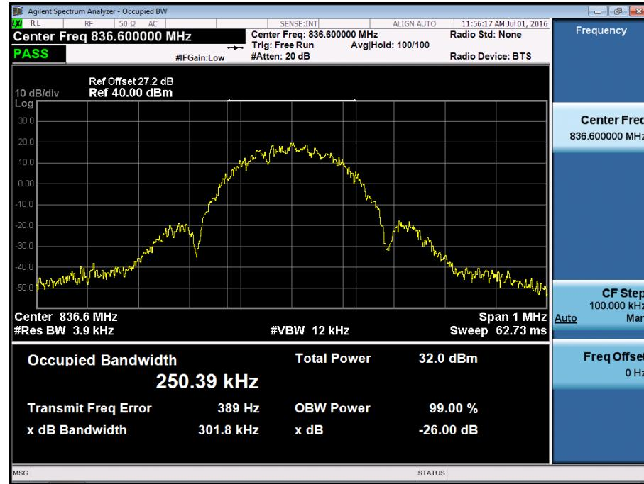
■ GSM1900 MODE (512 CH.) Occupied Bandwidth
