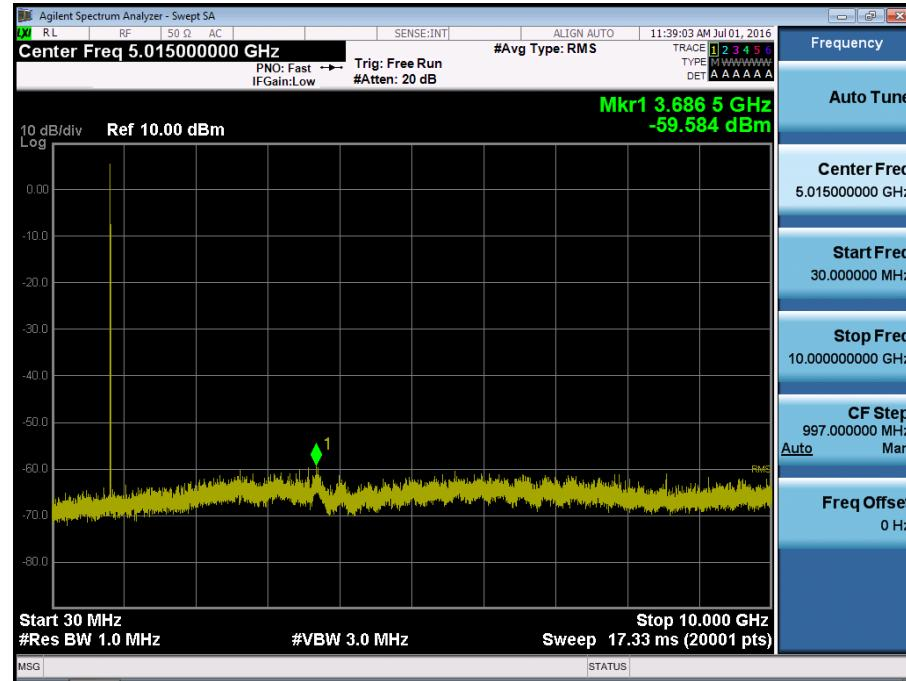
■ GSM850 MODE (251 CH.) Conducted Spurious Emissions
