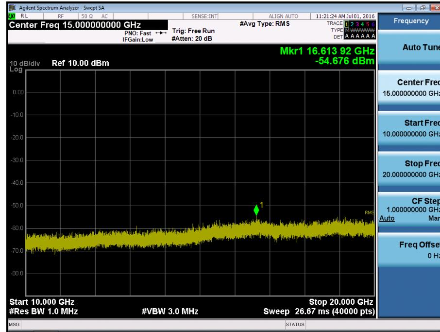
■ GSM1900 MODE (810 CH.) Conducted Spurious Emissions1
