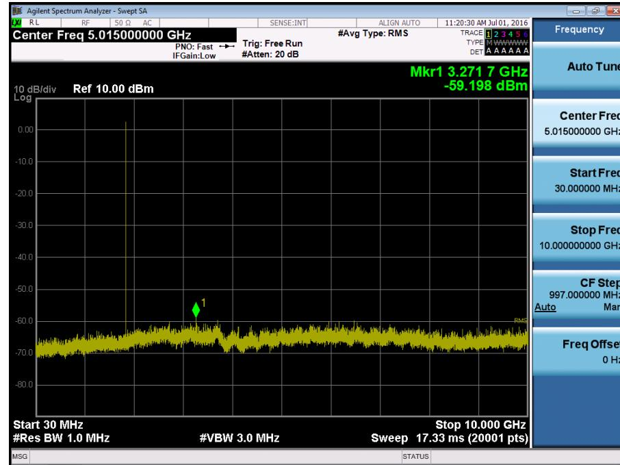
■ GSM1900 MODE (512 CH.) Conducted Spurious Emissions2
