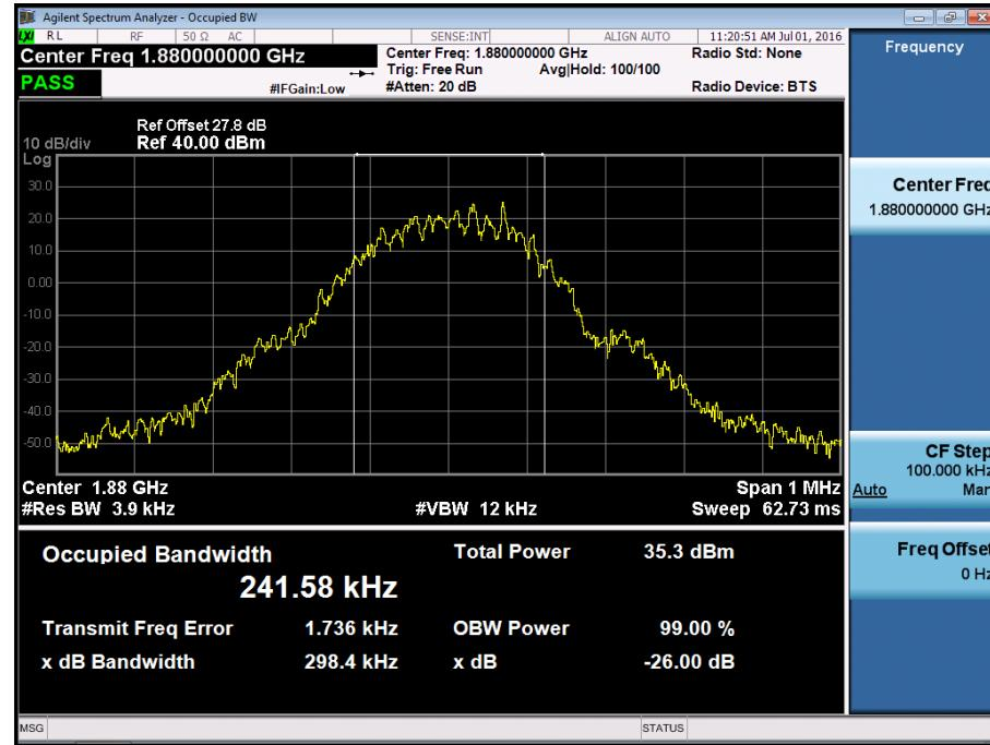
■ GSM1900 MODE (810 CH.) Occupied Bandwidth
