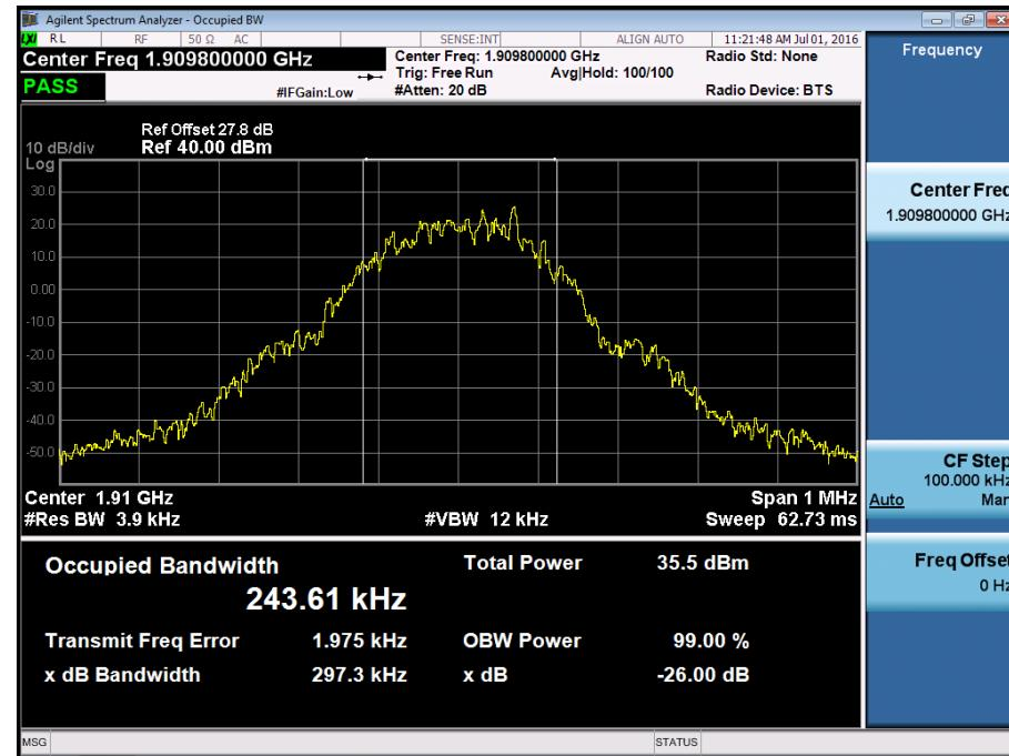
■ GSM1900 EDGE (810 CH.) Occupied Bandwidth
