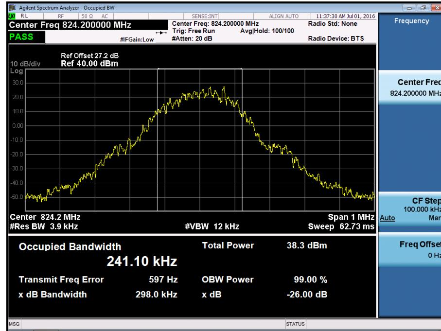
■ GSM850 MODE (190 CH.) Occupied Bandwidth
