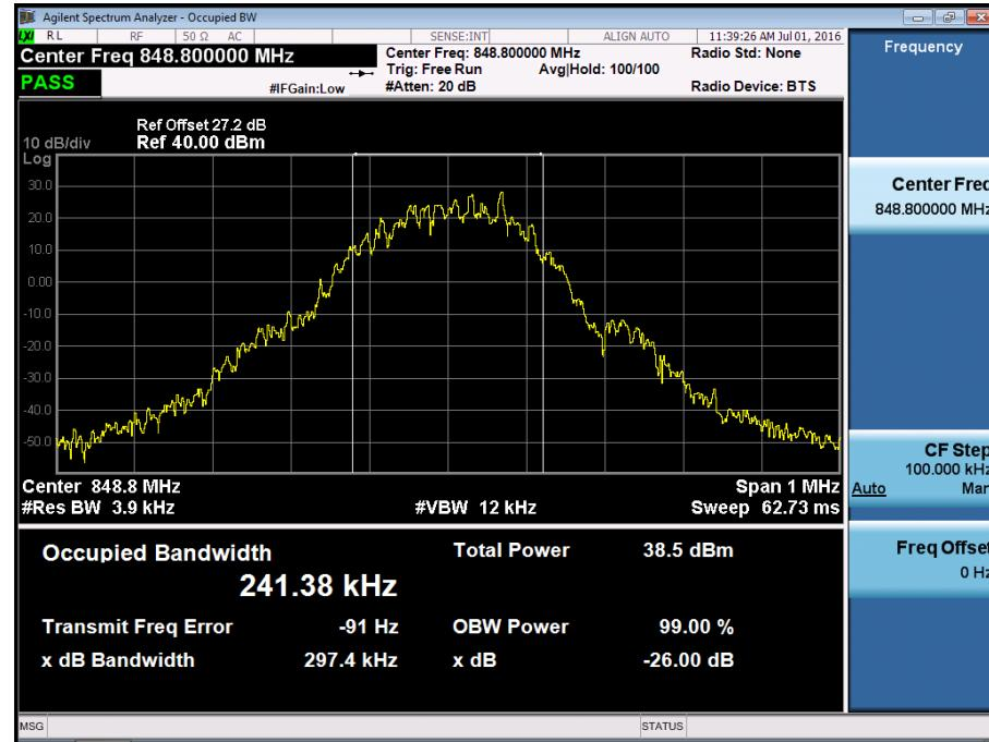
■ GSM850 EDGE (190 CH.) Occupied Bandwidth
