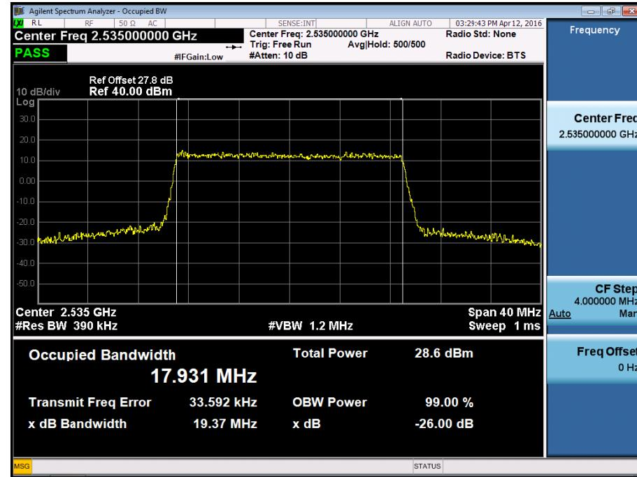
BAND7. Low Channel Edge Plot (5MHz Ch.20775 QPSK RB 25)-1
