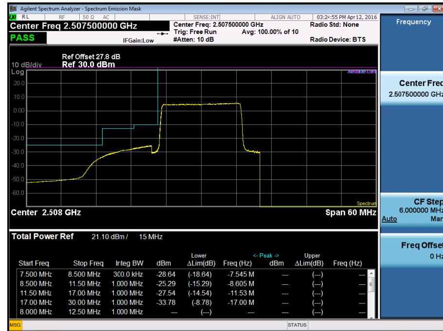
BAND7. Low Channel Edge Plot (15MHz Ch.20825 QPSK RB 75)-2
