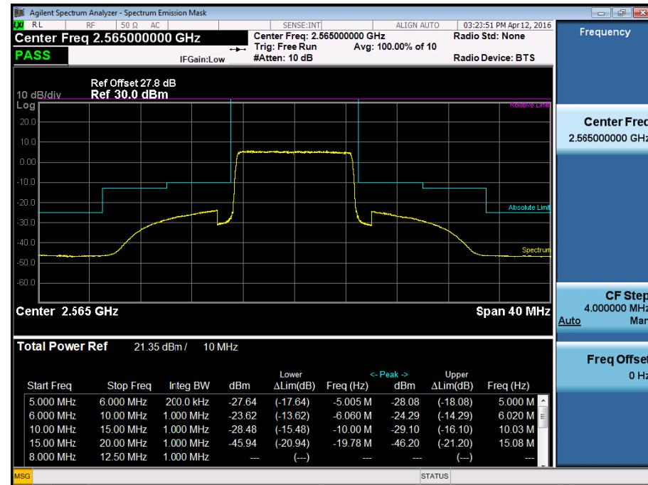
BAND7. Low Channel Edge Plot (15MHz Ch.20825 QPSK RB 75)-1
