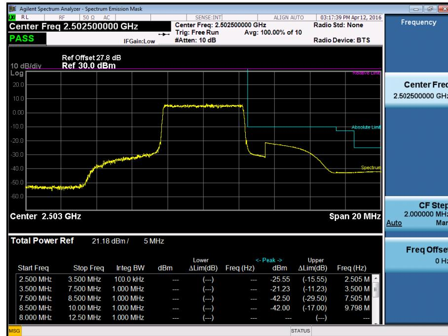
BAND7. Mid Channel Edge Plot (5MHz Ch.21100 QPSK RB 25)
