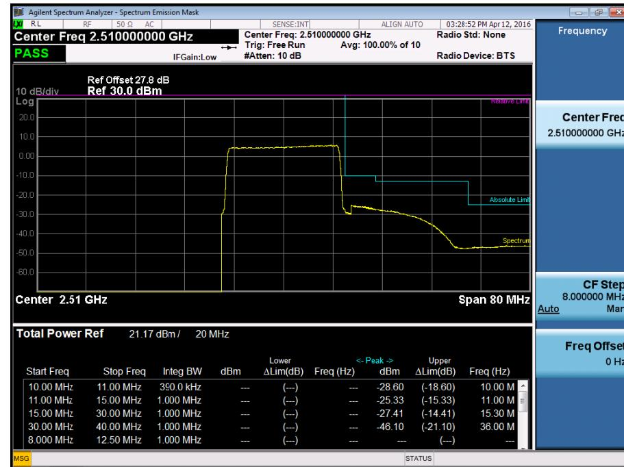
BAND7. Mid Channel Edge Plot (20MHz Ch.21100 QPSK RB 100)
