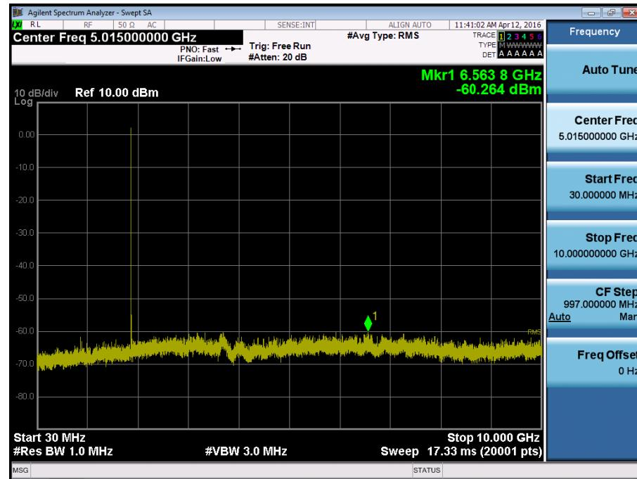
■ GSM1900 MODE (661 CH.) Conducted Spurious Emissions2
