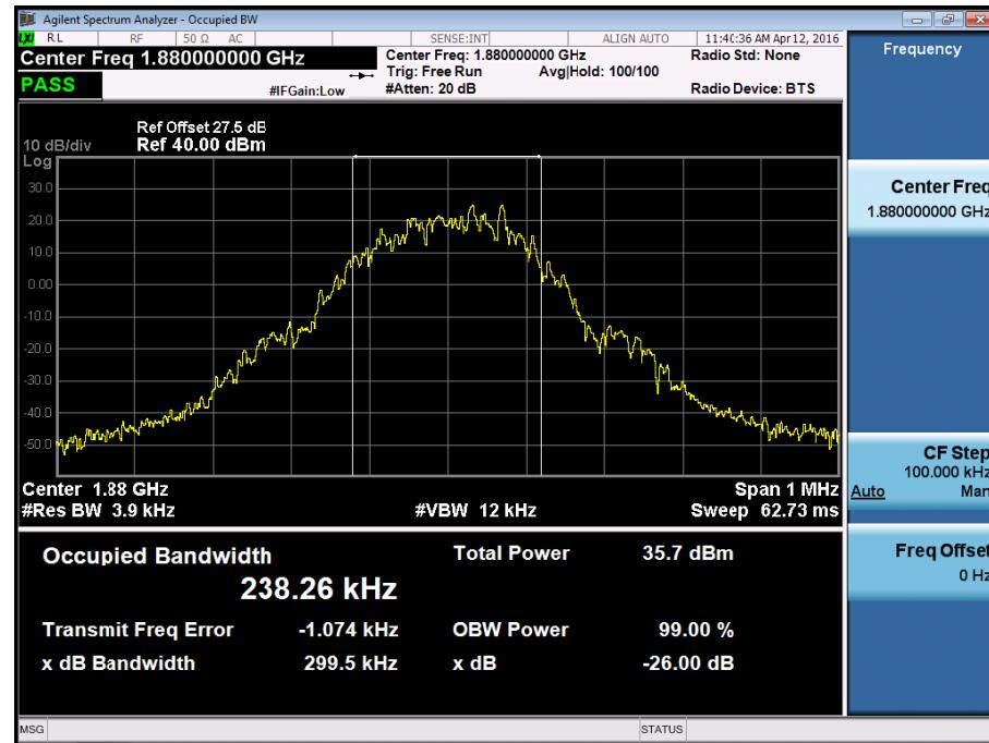
■ GSM1900 MODE (810 CH.) Occupied Bandwidth
