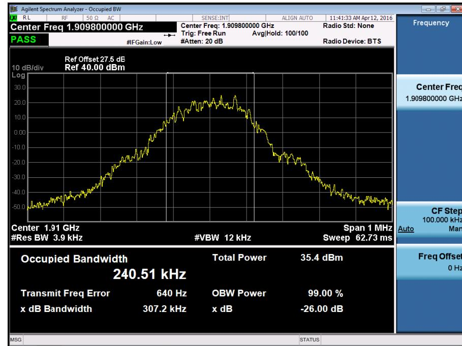
■ GSM1900 EDGE (512 CH.) Occupied Bandwidth
