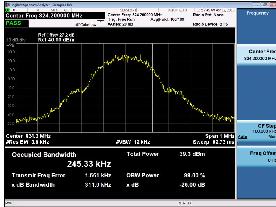
■ GSM850 MODE (190 CH.) Occupied Bandwidth
