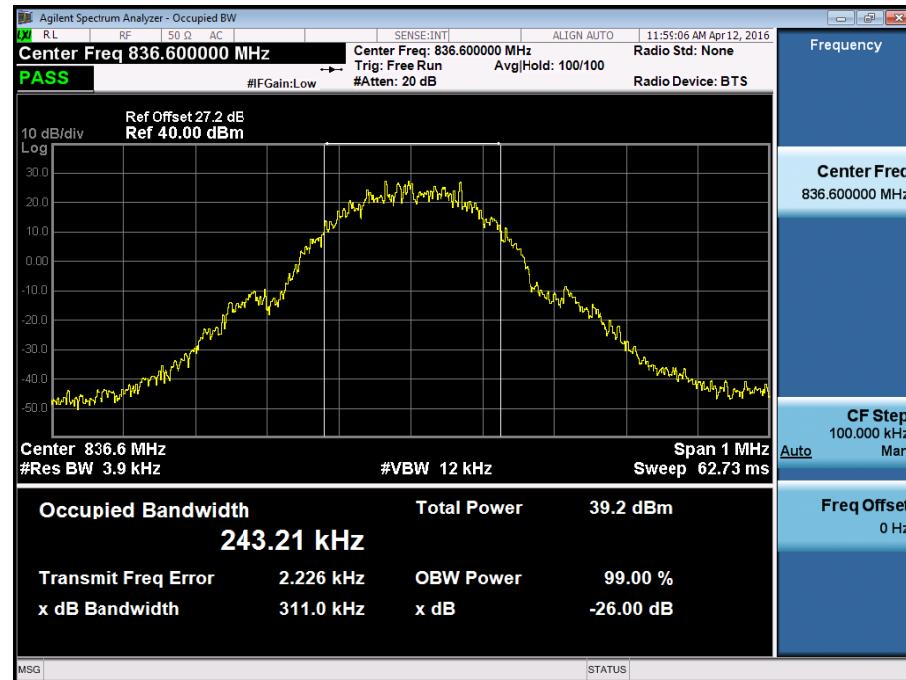
■ GSM850 MODE (251 CH.) Occupied Bandwidth
