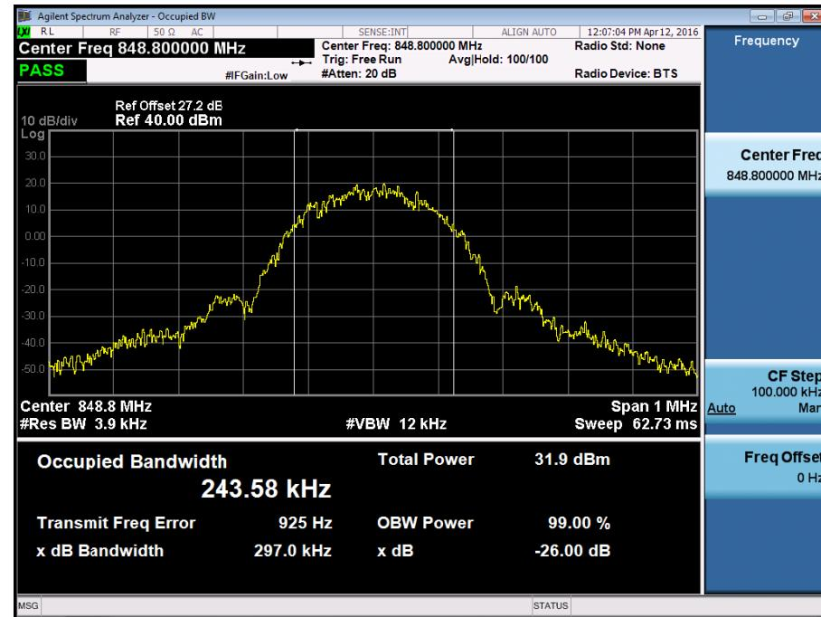
■ GSM1900 MODE (512 CH.) Occupied Bandwidth
