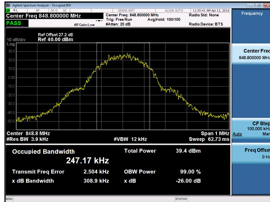
■ GSM850 EDGE (251 CH.) Occupied Bandwidth
