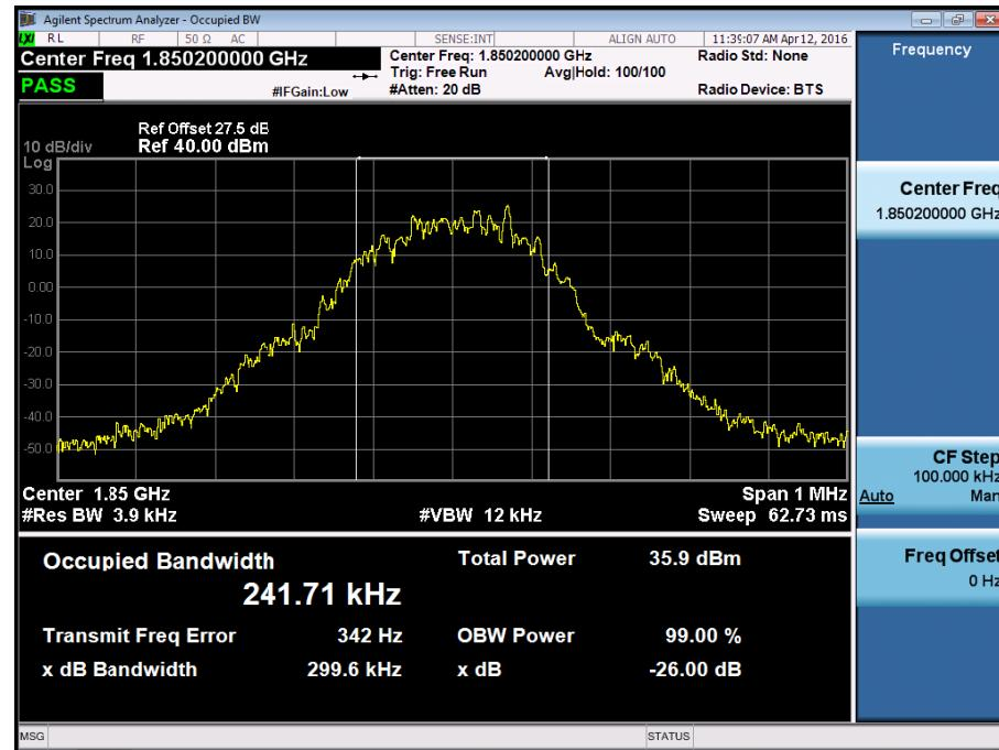
■ GSM1900 MODE (661 CH.) Occupied Bandwidth
