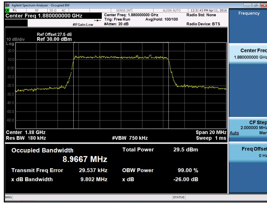
BAND 2. Occupied Bandwidth Plot (15M BW Ch.18900 QPSK RB 75\_0)
