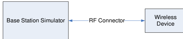
Figure 9-2 Power Measurement Setup
