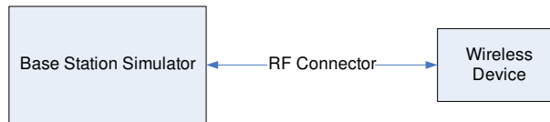
Figure 9-3 Power Measurement Setup
