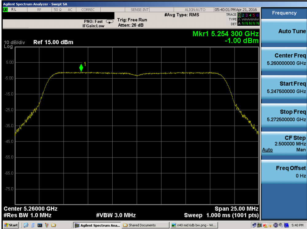
Plot 7-50. Power Spectral Density Plot (20MHz BW 802.11n (UNII Band 2A) – Ch. 52)
