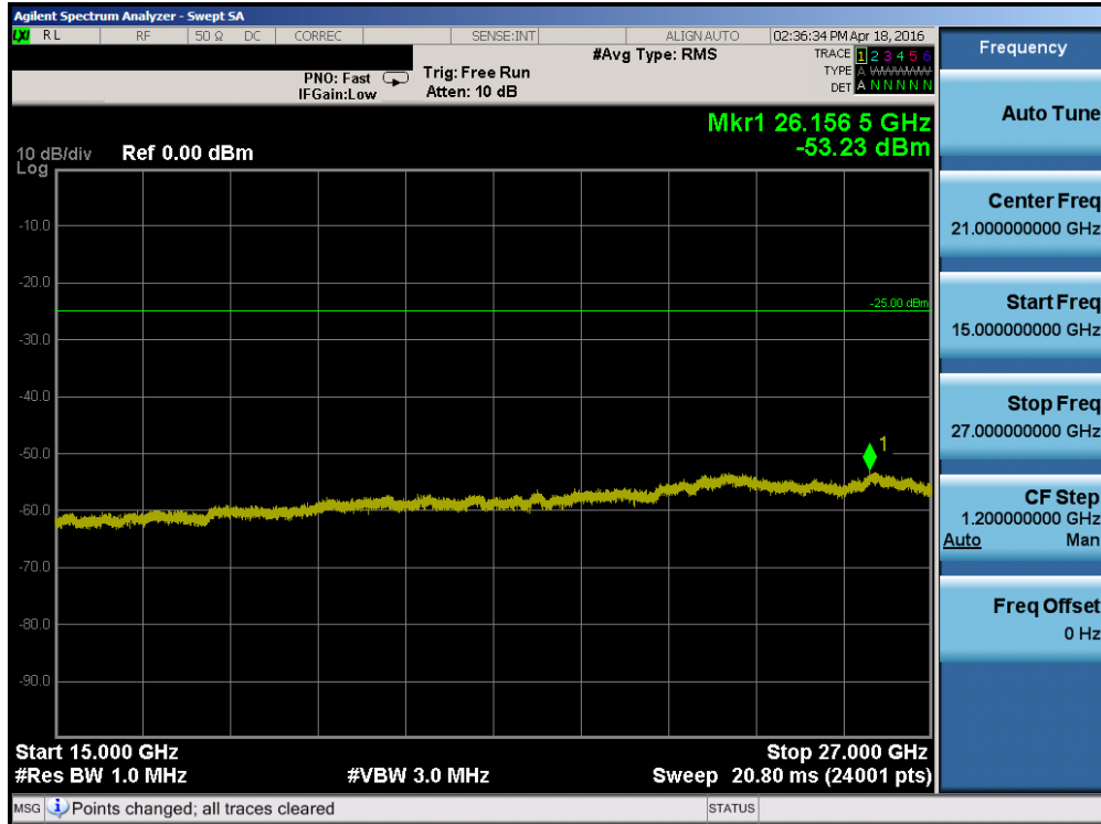
Plot 7-87. Conducted Spurious Plot (Band 7 – 20.0MHz QPSK – RB Size 1, RB Offset 0 – Low Channel)
