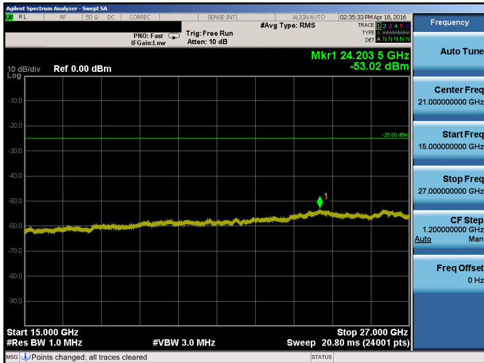
Plot 7-90. Conducted Spurious Plot (Band 7 – 20.0MHz QPSK – RB Size 1, RB Offset 0 – Mid Channel)
