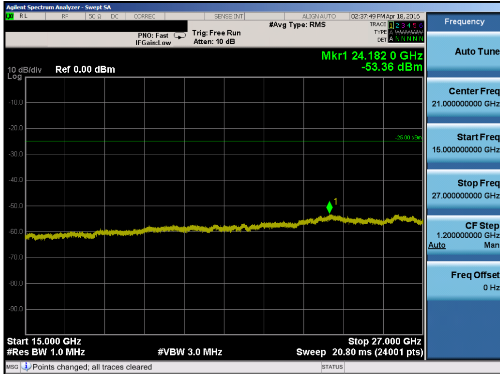
Plot 7-93. Conducted Spurious Plot (Band 7 – 20.0MHz QPSK – RB Size 1, RB Offset 0 – High Channel)
