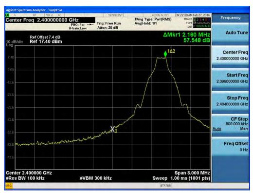
Test Plots without hopping (GFSK) Band Edges (High-CH)
