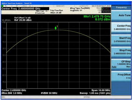
Test Plots (8DPSK) Peak Power (Low-CH)
