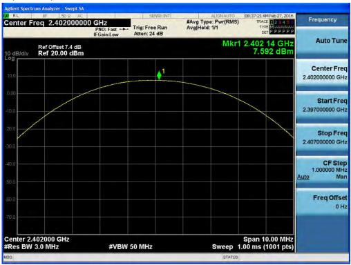
Test Plots (π/4DQPSK) Peak Power (Mid-CH)
