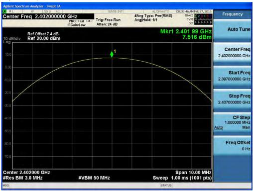
Test Plots (GFSK) Peak Power (Mid-CH)
