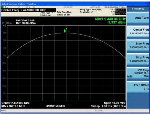
Test Plots (8DPSK) Peak Power (High-CH)
