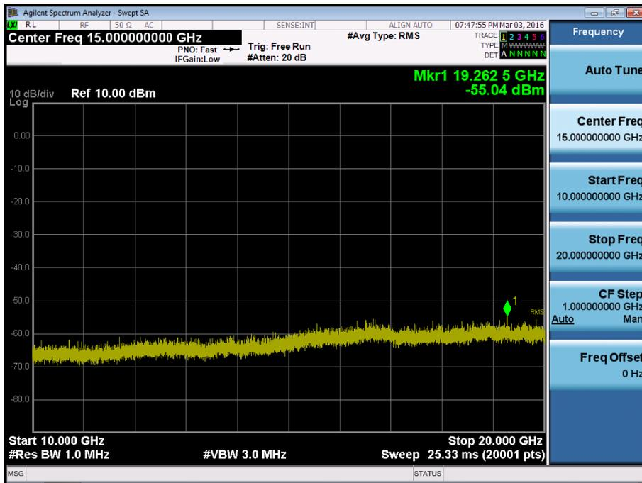
BAND 2. Conducted Spurious\_1 (19185ch\_3MHz\_QPSK\_RB 1\_0)
