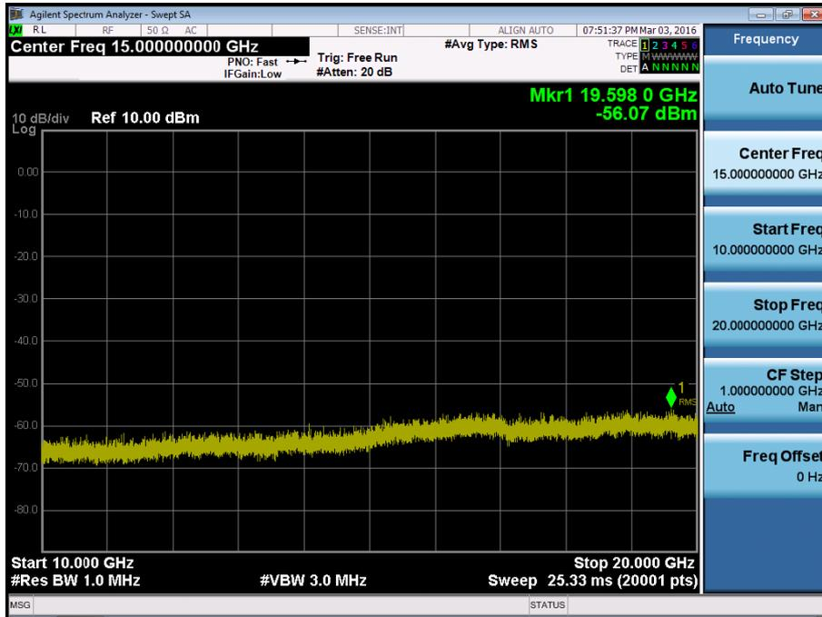
BAND 2. Conducted Spurious\_1 (19175ch\_5MHz\_QPSK\_RB 1\_0)
