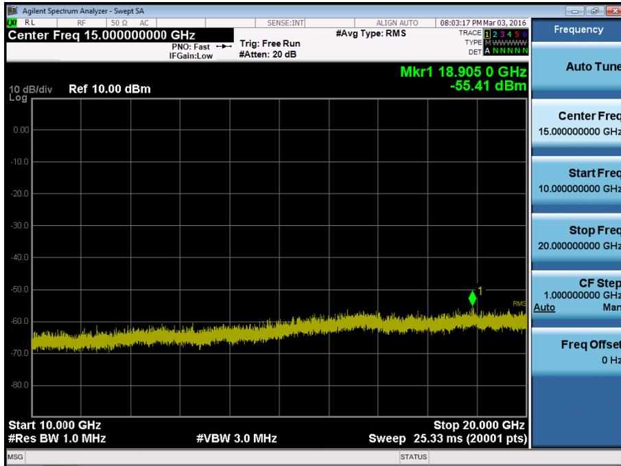
BAND 2. Conducted Spurious\_1 (19100ch\_20MHz\_QPSK\_RB 1\_0)
