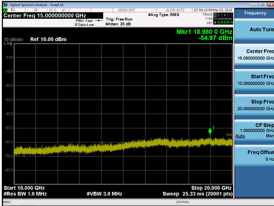
BAND 2. Conducted Spurious\_1 (19125ch\_15MHz\_QPSK\_RB 1\_0)
