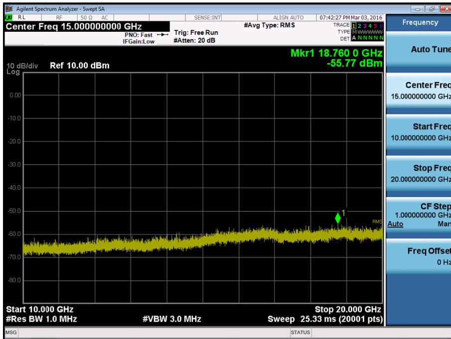
BAND 2. Conducted Spurious\_1 (18900ch\_1.4MHz\_QPSK\_RB 1\_0)
