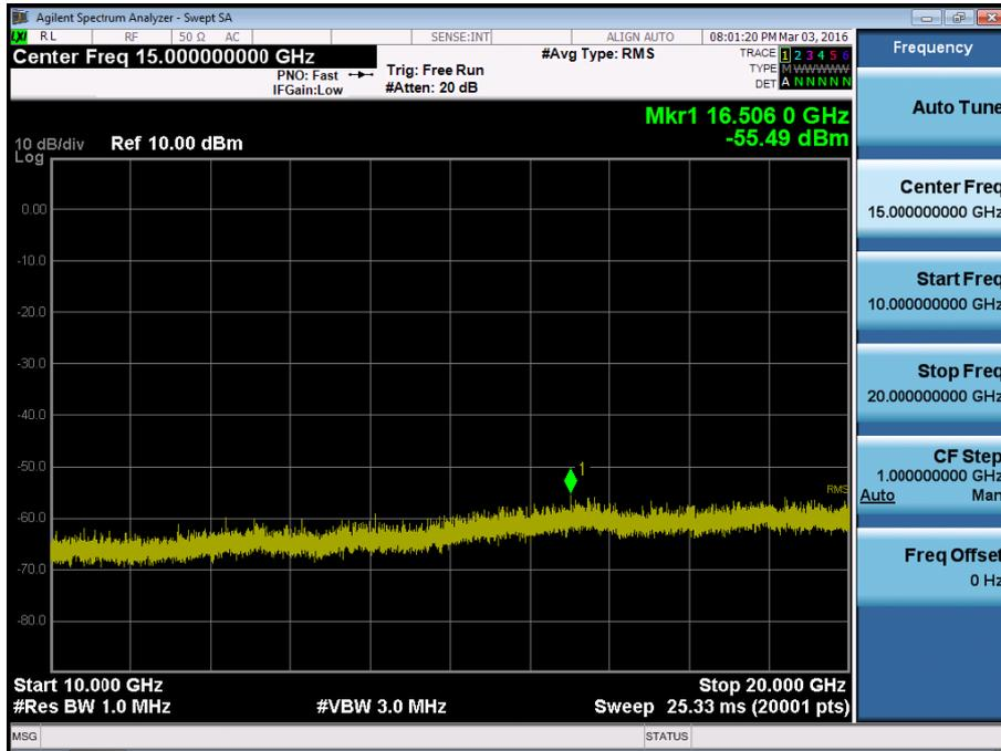
BAND 2. Conducted Spurious\_1 (18900ch\_20MHz\_QPSK\_RB 1\_0)
