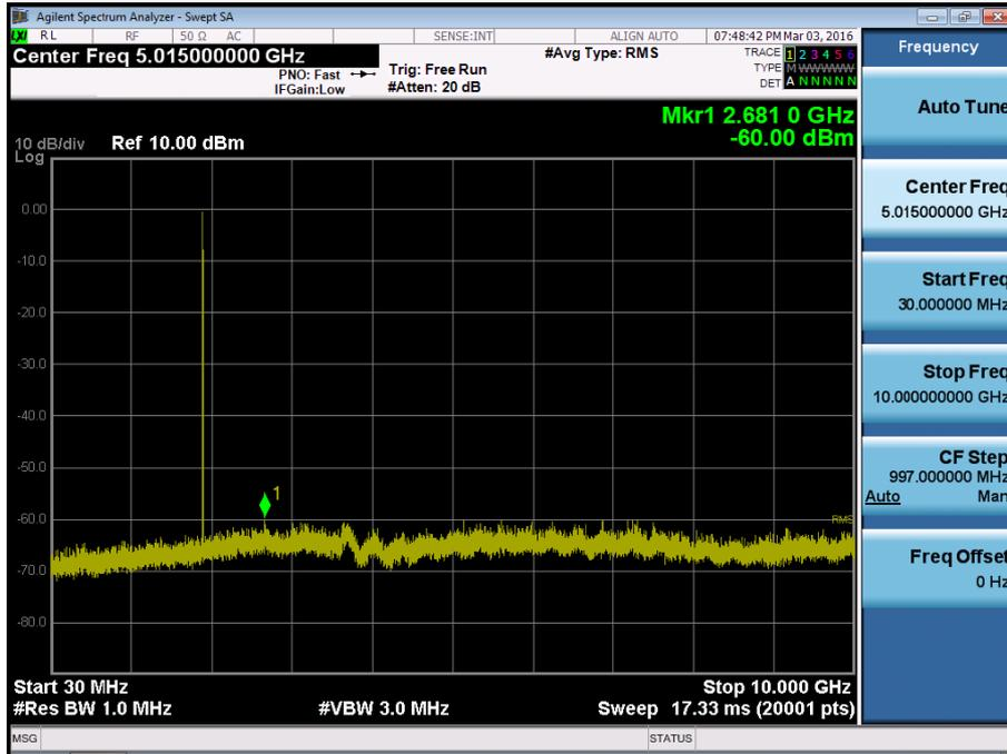
BAND 2. Conducted Spurious\_2 (19185ch\_3MHz\_QPSK\_RB 1\_0)
