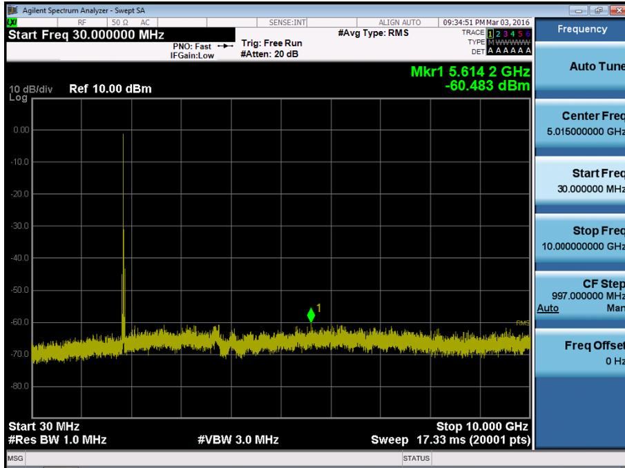
BAND 2. Conducted Spurious\_2 (18700ch\_20MHz\_QPSK\_RB 1\_0)
