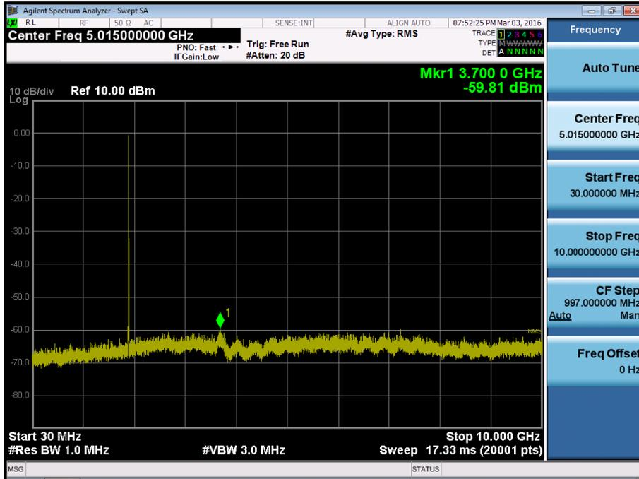
BAND 2. Conducted Spurious\_2 (19175ch\_5MHz\_QPSK\_RB 1\_0)
