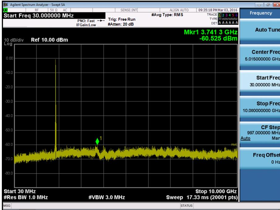
BAND 2. Conducted Spurious\_2 (18900ch\_20MHz\_QPSK\_RB 1\_0)
