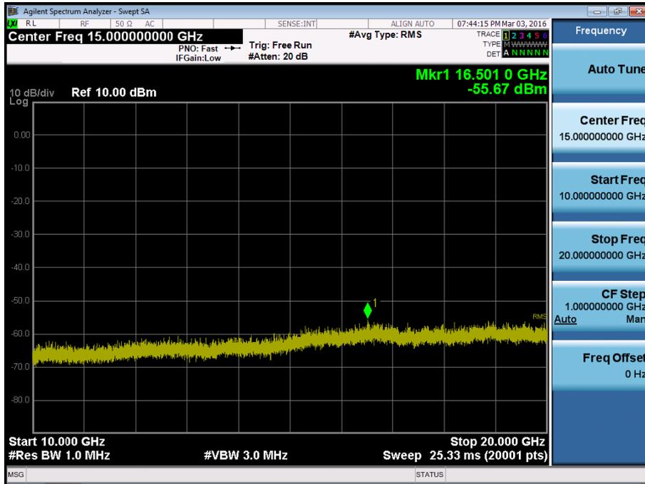
BAND 2. Conducted Spurious\_1 (19193ch\_1.4MHz\_QPSK\_RB 1\_0)
