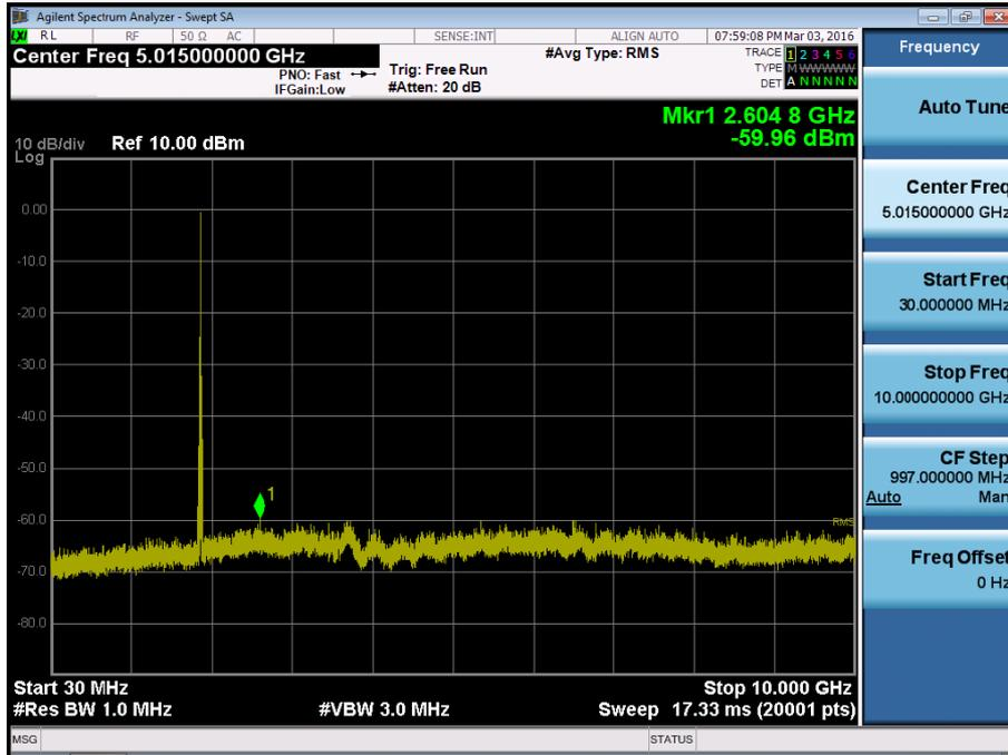
BAND 2. Conducted Spurious\_2 (18900ch\_15MHz\_QPSK\_RB 1\_0)
