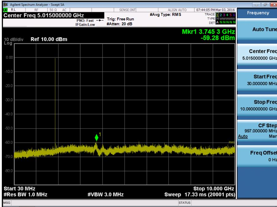
BAND 2. Conducted Spurious\_2 (18900ch\_1.4MHz\_QPSK\_RB 1\_0)
