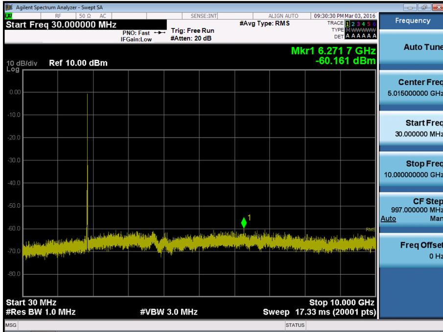
BAND 2. Conducted Spurious\_2 (18650ch\_10MHz\_QPSK\_RB 1\_0)
