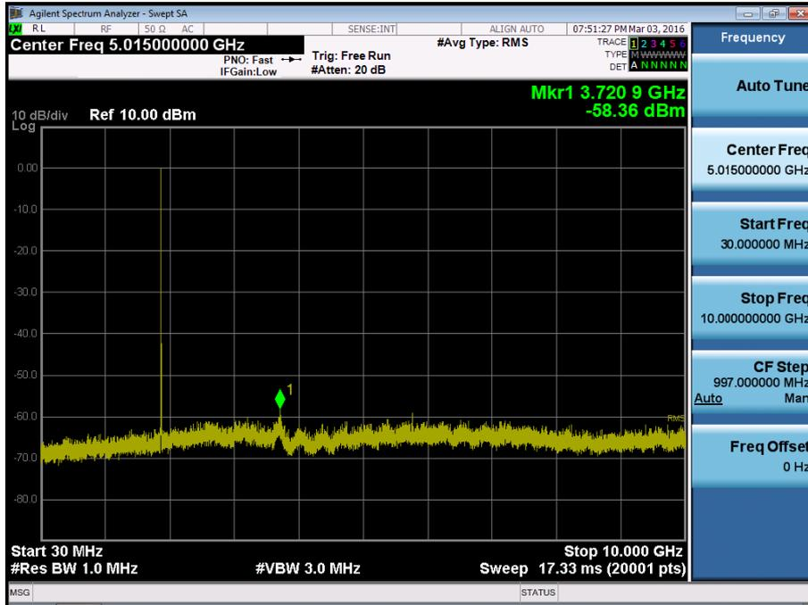
BAND 2. Conducted Spurious\_2 (18900ch\_5MHz\_QPSK\_RB 1\_0)
