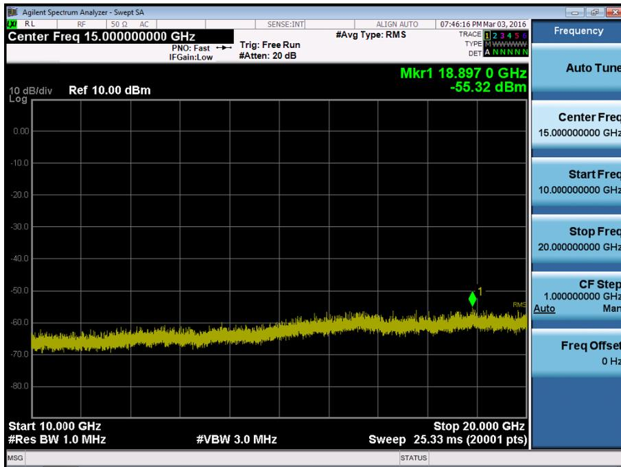
BAND 2. Conducted Spurious\_1 (18900ch\_3MHz\_QPSK\_RB 1\_0)
