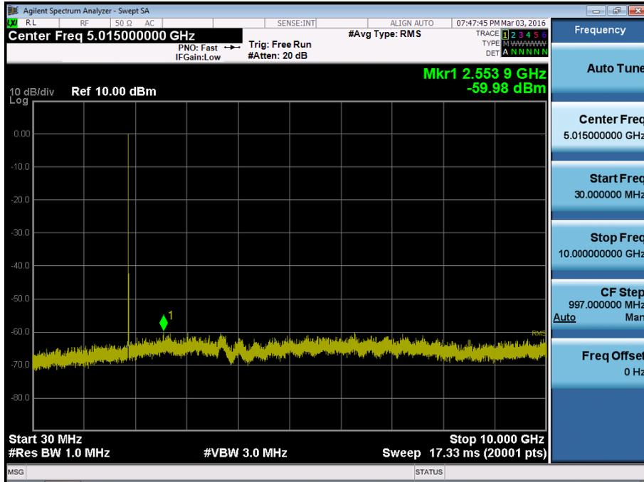
BAND 2. Conducted Spurious\_2 (18900ch\_3MHz\_QPSK\_RB 1\_0)
