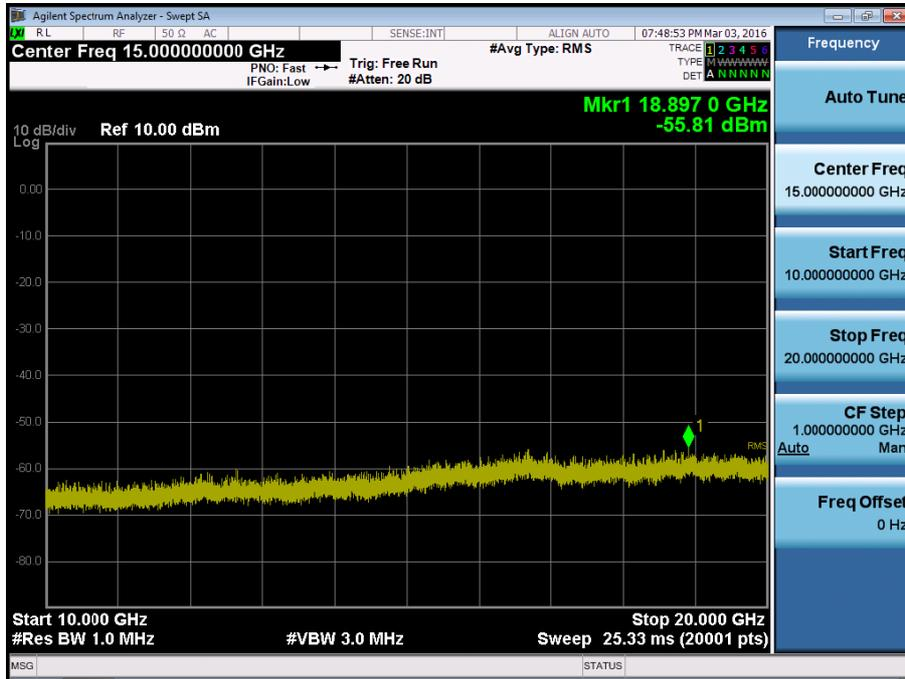
BAND 2. Conducted Spurious\_1 (18625ch\_5MHz\_QPSK\_RB 1\_0)
