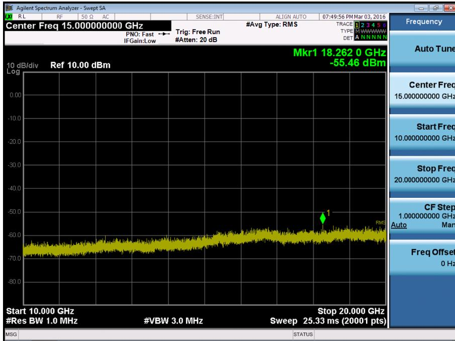
BAND 2. Conducted Spurious\_1 (18900ch\_5MHz\_QPSK\_RB 1\_0)
