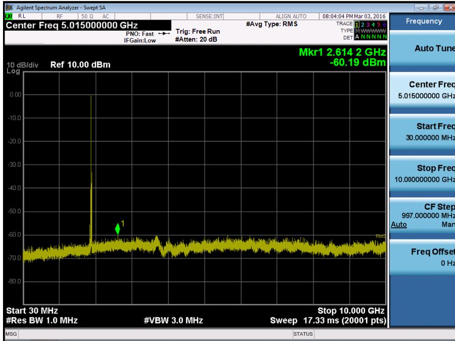
BAND 2. Conducted Spurious\_2 (19100ch\_20MHz\_QPSK\_RB 1\_0)
