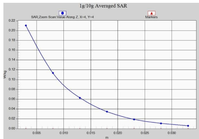
Fig. 1-15 Z-Scan at power reference point (LTE Band7)
