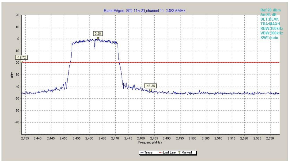
Fig.A.5.10 Band Edges (802.11n-HT20, Ch 11)
