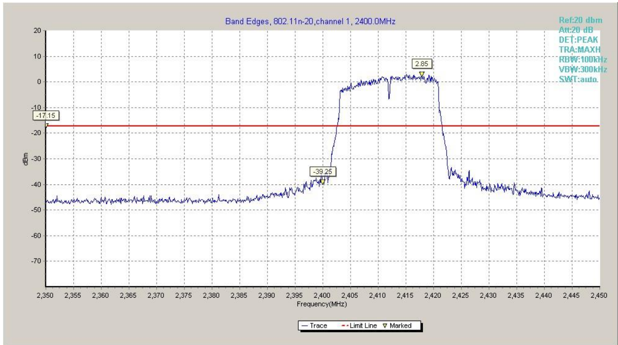
Fig.A.5.9 Band Edges (802.11n-HT20, Ch 1)
