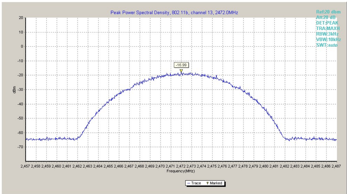
Fig.A.3.5 Power Spectral Density (802.11b, Ch 13)
