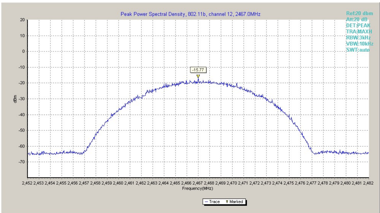
Fig.A.3.4 Power Spectral Density (802.11b, Ch 12)
