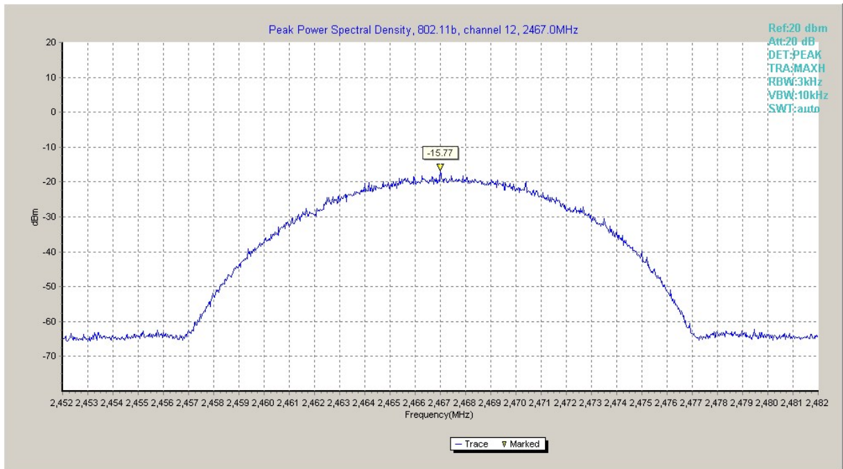
Fig.A.3.4 Power Spectral Density (802.11b, Ch 12)
