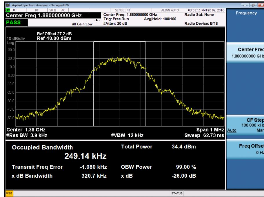
■ GSM1900 MODE (810 CH.) Occupied Bandwidth
