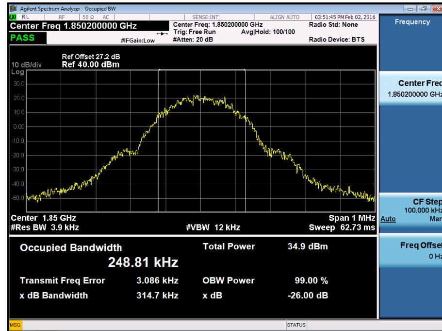
■ GSM1900 MODE (661 CH.) Occupied Bandwidth
