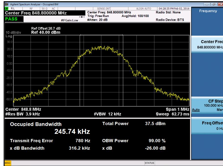
■ GSM850 EDGE (251 CH.) Occupied Bandwidth
