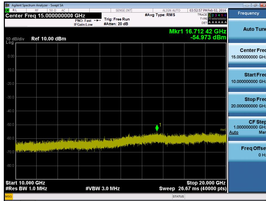
■ GSM1900 MODE (661 CH) Conducted Spurious Emissions1
