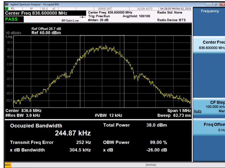
■ GSM850 MODE (251 CH.) Occupied Bandwidth
