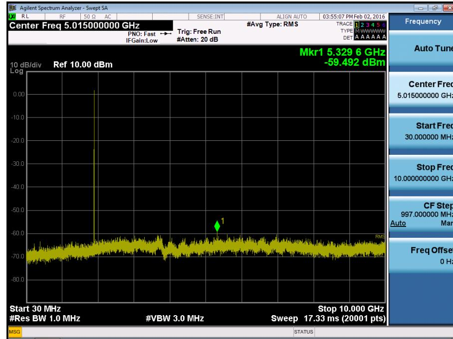
■ GSM1900 MODE (810 CH.) Conducted Spurious Emissions2
