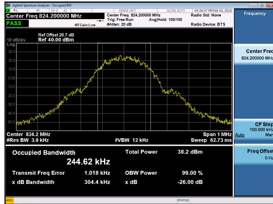
■ GSM850 MODE (190 CH.) Occupied Bandwidth
