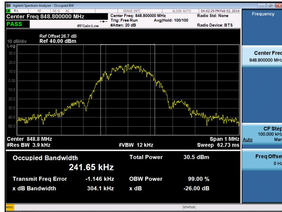
■ GSM1900 MODE (512 CH.) Occupied Bandwidth
