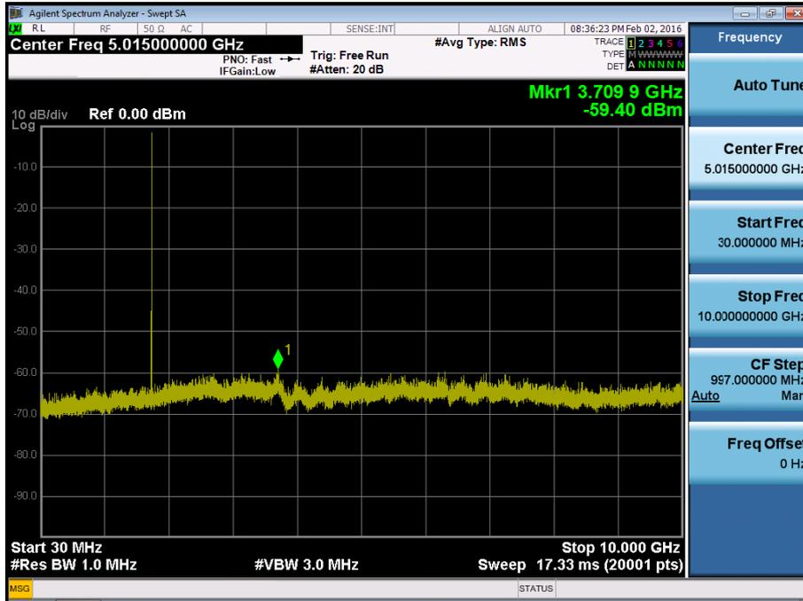
BAND 4. Conducted Spurious Plot\_2 (20385ch\_3MHz\_QPSK\_RB 1\_0)
