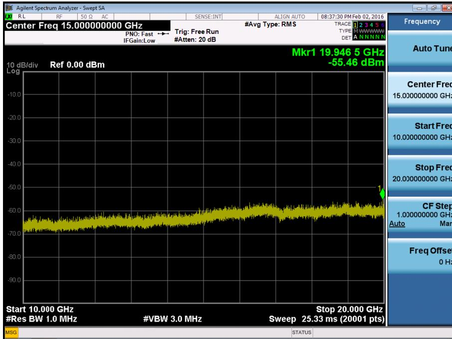
BAND 4. Conducted Spurious Plot\_1 (20375ch\_5MHz\_QPSK\_RB 1\_0)
