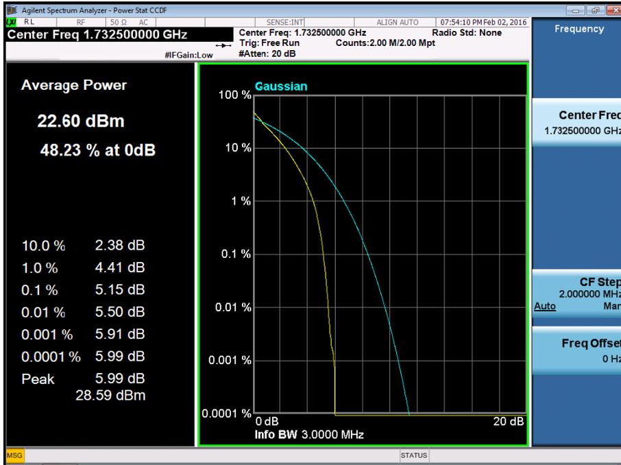
BAND 4. PAR Plot (3M BW\_Ch.20175\_16QAM\_RB15\_0)
