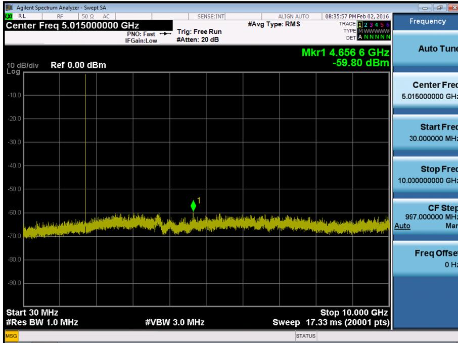
BAND 4. Conducted Spurious Plot\_2 (20175ch\_3MHz\_QPSK\_RB 1\_0)
