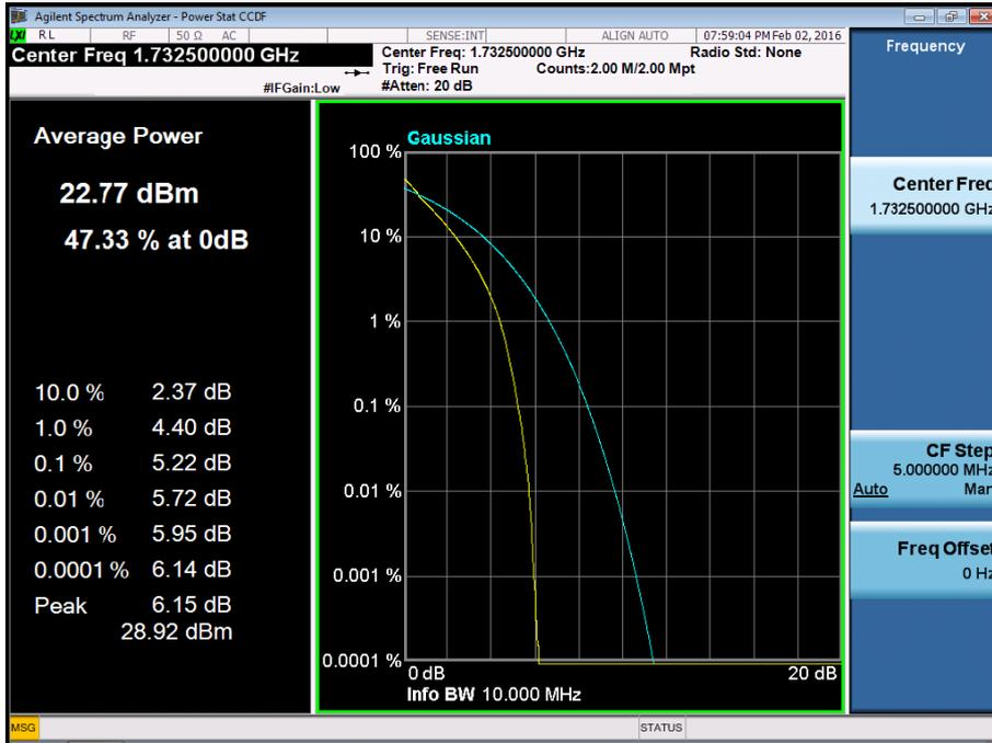
BAND 4. PAR Plot (10M BW\_Ch.20175\_16QAM\_RB50\_0)
