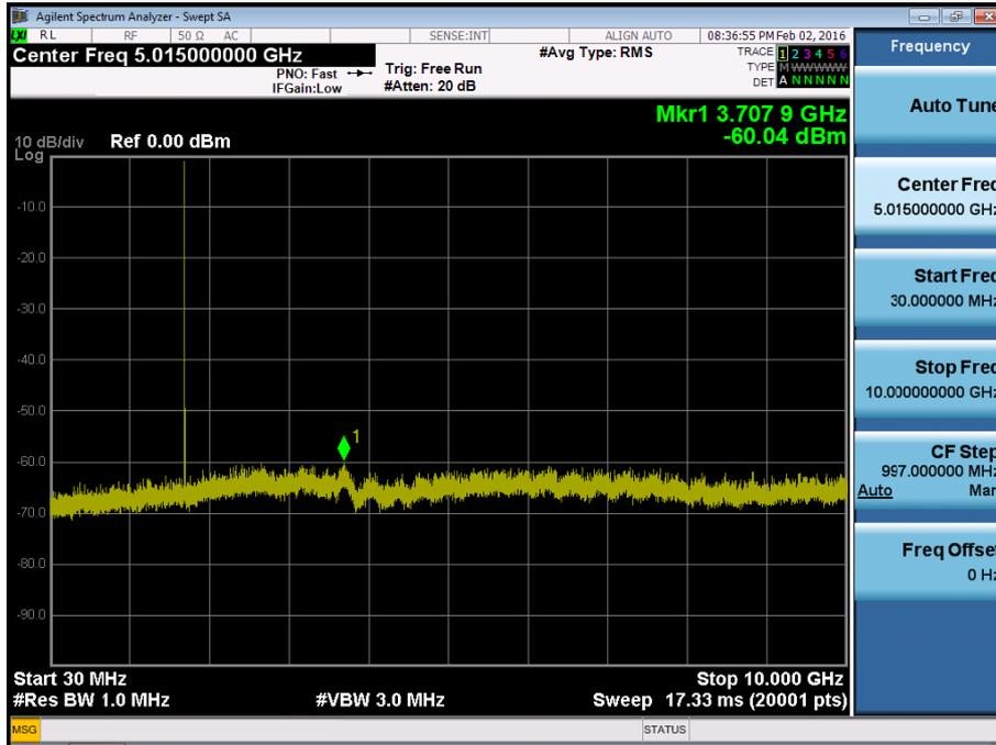
BAND 4. Conducted Spurious Plot\_2 (19975ch\_5MHz\_QPSK\_RB 1\_0)
