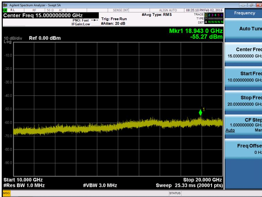
BAND 4. Conducted Spurious Plot\_1 (19965ch\_3MHz\_QPSK\_RB 1\_0)
