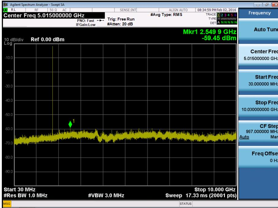
BAND 4. Conducted Spurious Plot\_2 (20393ch\_1.4MHz\_QPSK\_RB 1\_0)
