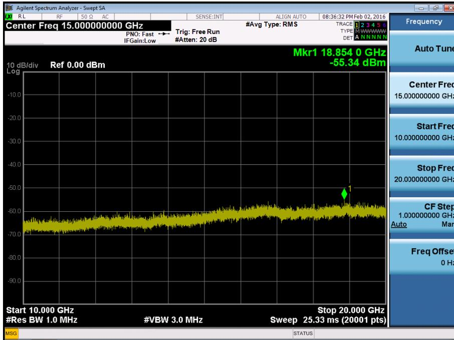
BAND 4. Conducted Spurious Plot\_1 (19975ch\_5MHz\_QPSK\_RB 1\_0)
