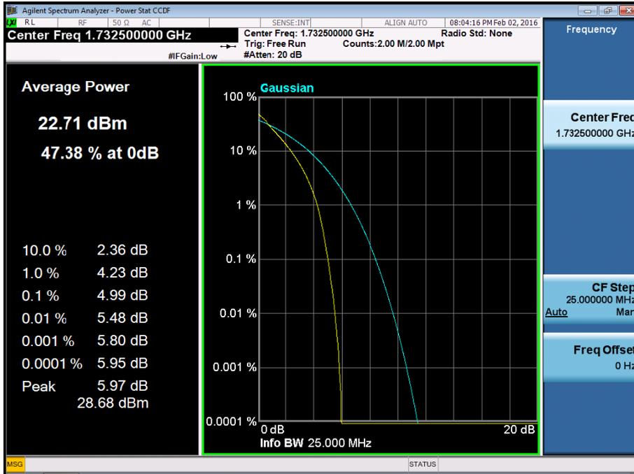
BAND 4. PAR Plot (20M BW\_Ch.20175\_16QAM\_RB100\_0)
