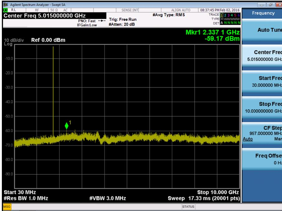
BAND 4. Conducted Spurious Plot\_2 (20375ch\_5MHz\_QPSK\_RB 1\_0)
