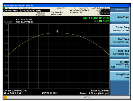
Test Plots (GFSK) Peak Power (Mid-CH)
