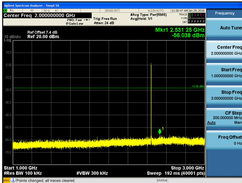
**Note : Fundamental maximum level(average mode) is 1.54 dBm. Limit line is 20 dBc down from the fundamental. So, limit is -18.46 dBm.**
