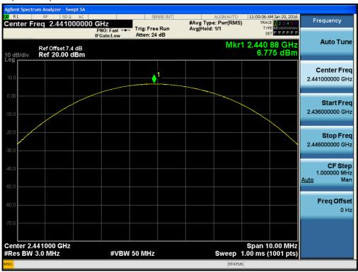
Test Plots (8DPSK) Peak Power (High-CH)
