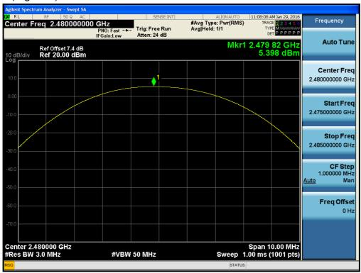
Test Plots (8DPSK) Peak Power (Low-CH)
