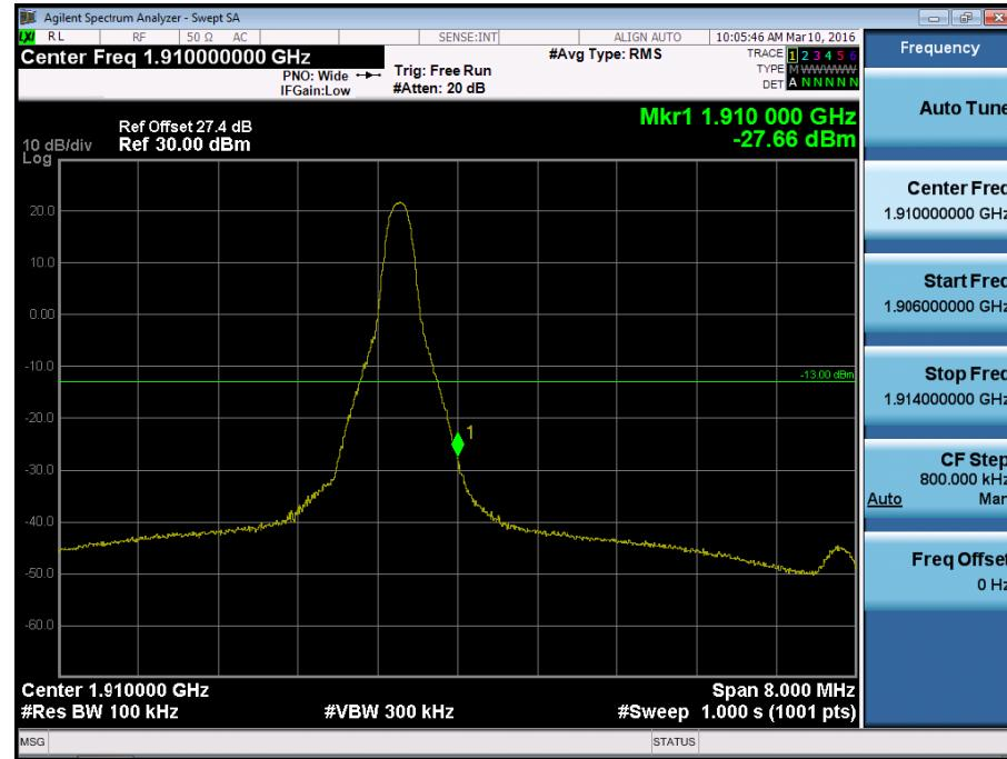
BAND 2. Upper Band Edge Plot (10M BW Ch.19150 QPSK\_RB50\_Offset 0) -2
