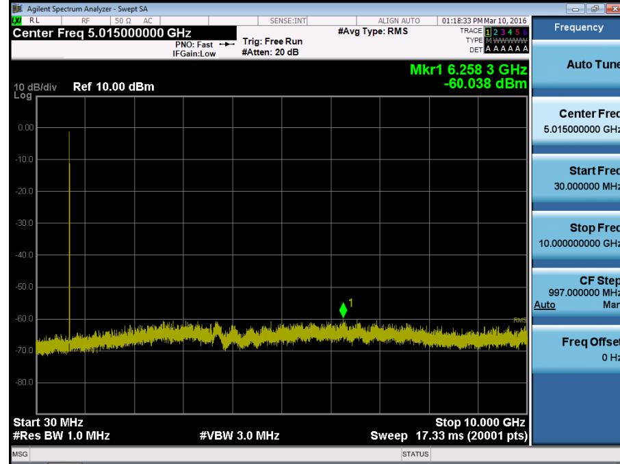
BAND 17. Conducted Spurious Plot\_ (23780ch\_10MHz\_QPSK\_RB 1\_0)
