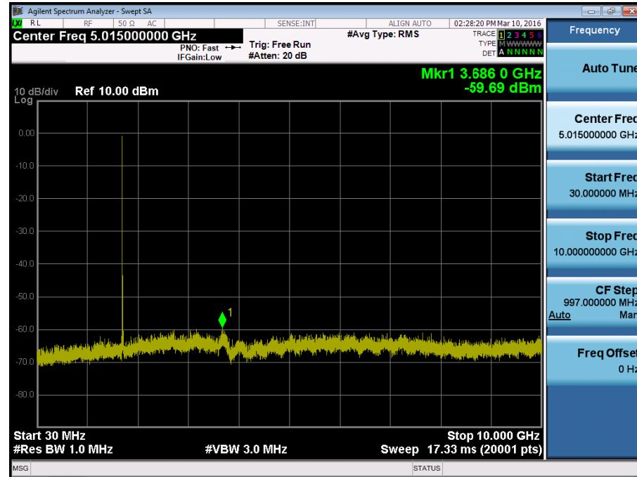
BAND 4. Conducted Spurious Plot\_2 (20025ch\_15MHz\_QPSK\_RB 1\_0)
