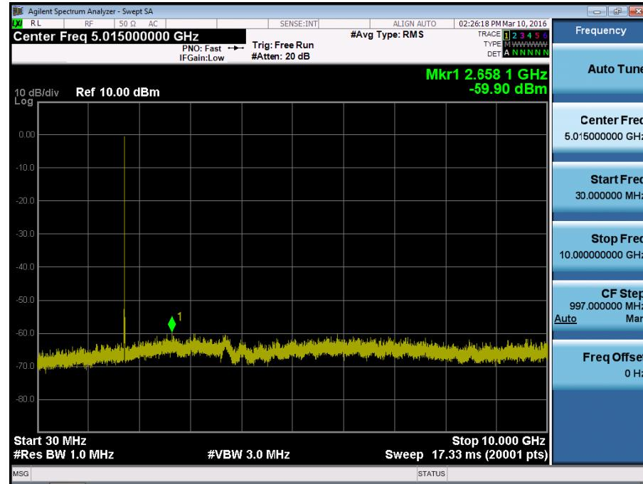
BAND 4. Conducted Spurious Plot\_2 (20175ch\_10MHz\_QPSK\_RB 1\_0)
