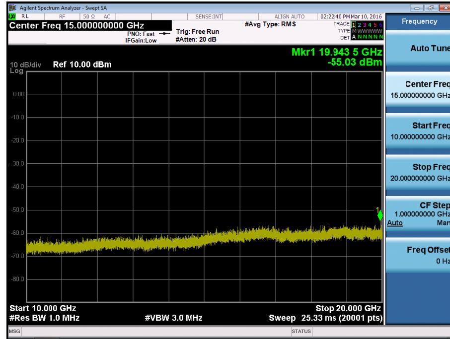
BAND 4. Conducted Spurious Plot\_1 (20375ch\_5MHz\_QPSK\_RB 1\_0)
