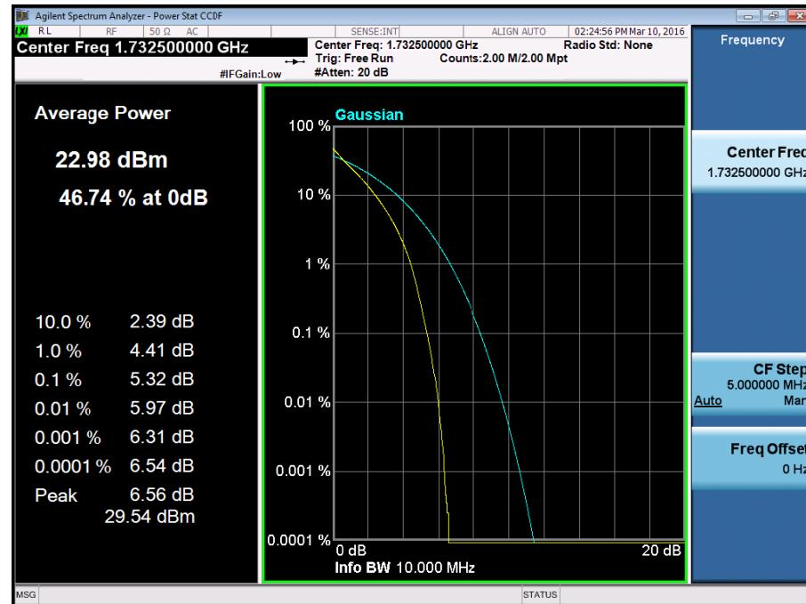
BAND 4. PAR Plot (10M BW\_Ch.20175\_16QAM\_RB50\_0)
