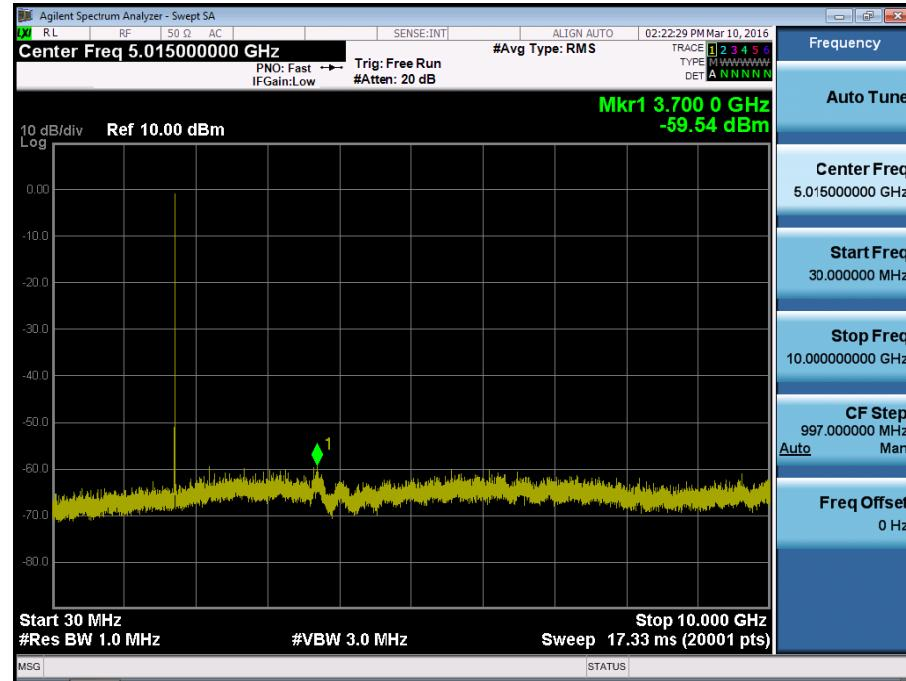
BAND 4. Conducted Spurious Plot\_2 (20175ch\_5MHz\_QPSK\_RB 1\_0)
