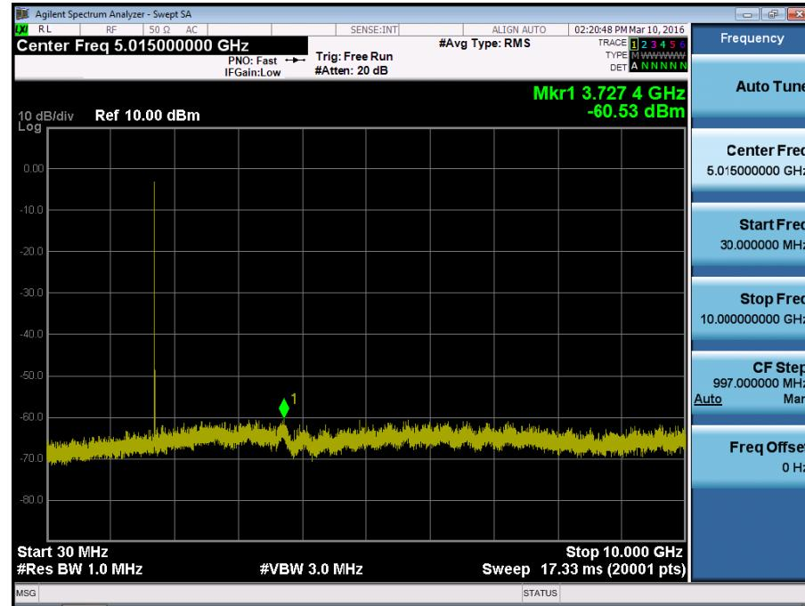
BAND 4. Conducted Spurious Plot\_2 (19975ch\_5MHz\_QPSK\_RB 1\_0)
