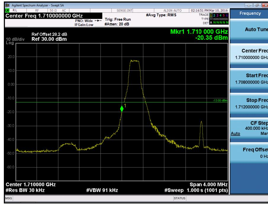
BAND 4.Lower Band Edge Plot (3M BW Ch.19965 QPSK RB 15) -2
