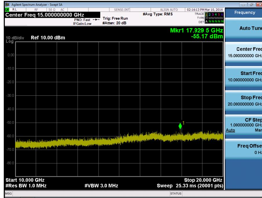
BAND 4. Conducted Spurious Plot\_1 (19965ch\_3MHz\_QPSK\_RB 1\_0)
