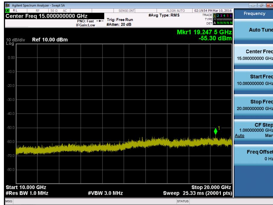
BAND 4. Conducted Spurious Plot\_1 (19975ch\_5MHz\_QPSK\_RB 1\_0)
