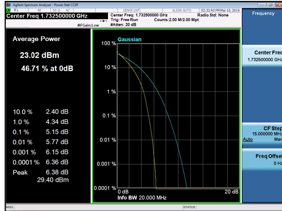
BAND 4. PAR Plot (20M BW\_Ch.20175\_16QAM\_RB100\_0)
