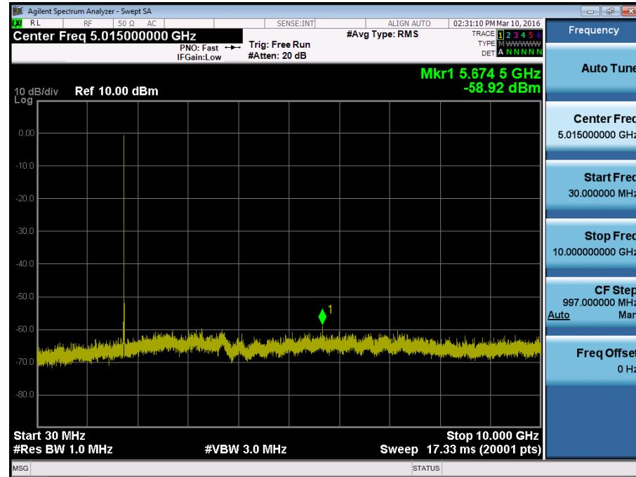
BAND 4. Conducted Spurious Plot\_2 (20325ch\_15MHz\_QPSK\_RB 1\_0)
