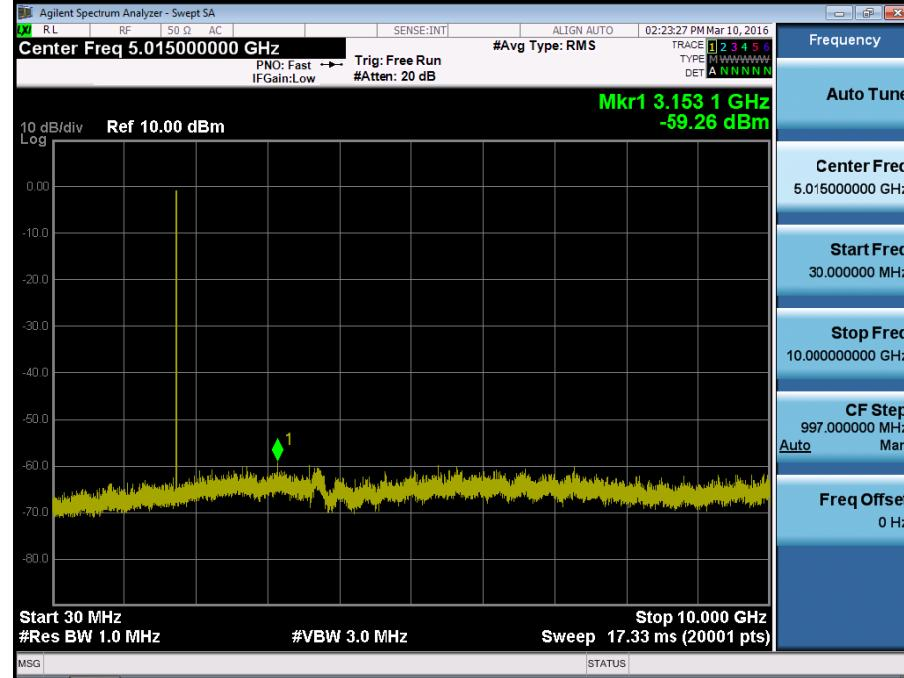
BAND 4. Conducted Spurious Plot\_2 (20375ch\_5MHz\_QPSK\_RB 1\_0)
