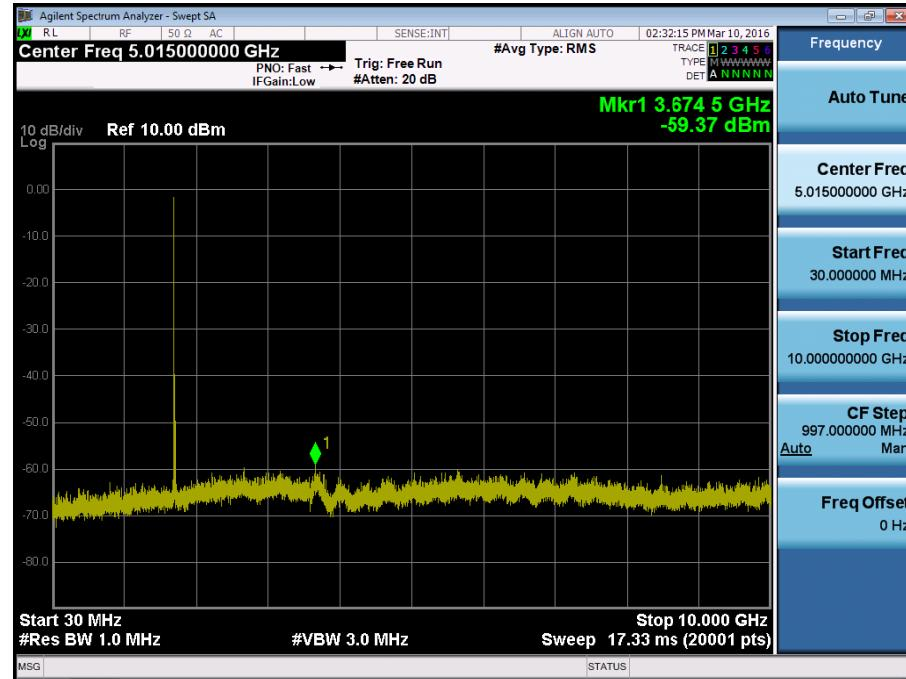
BAND 4. Conducted Spurious Plot\_2 (20050ch\_20MHz\_QPSK\_RB 1\_0)
