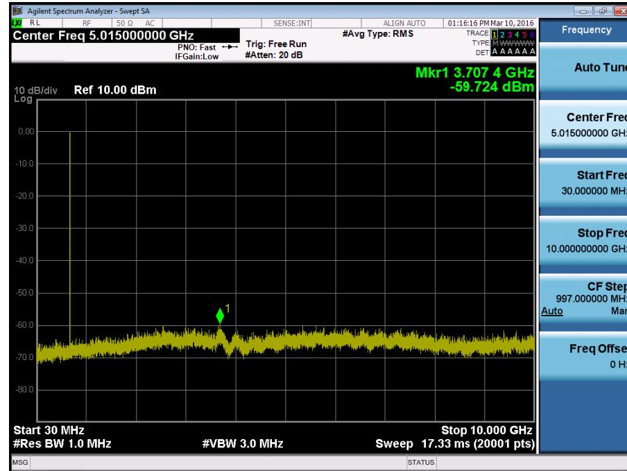
BAND 17. Conducted Spurious Plot\_ (23790ch\_5MHz\_QPSK\_RB 1\_0)
