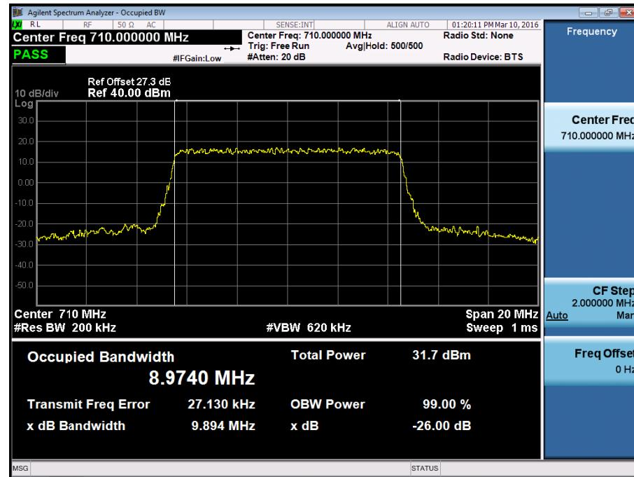
BAND 17. Occupied Bandwidth Plot (10M BW Ch.23790 16QAMRB 50)
