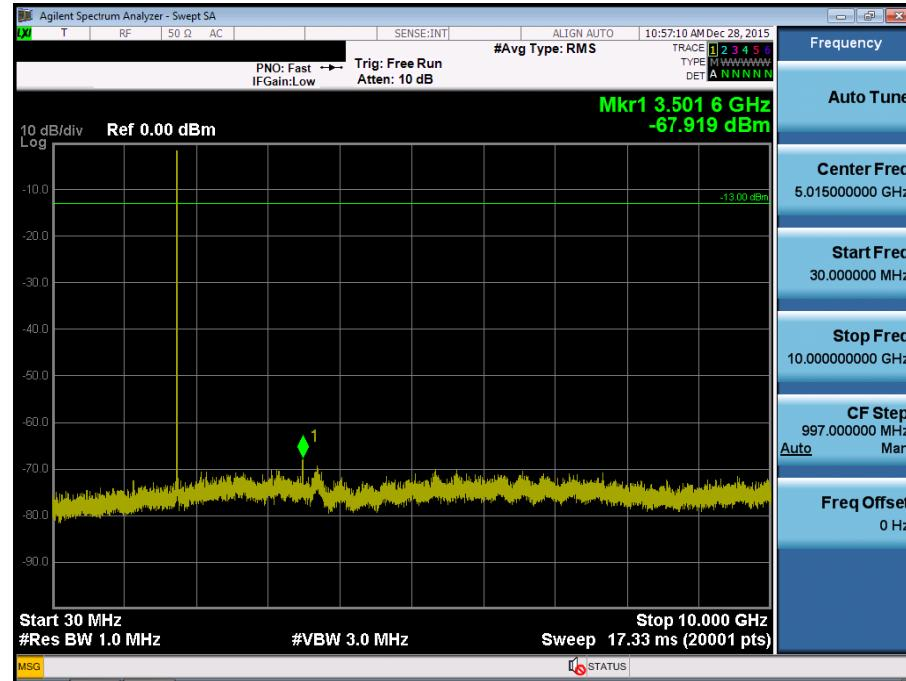
BAND 4. Conducted Spurious Plot\_2 (20375ch\_5MHz\_QPSK\_RB 1\_0)
