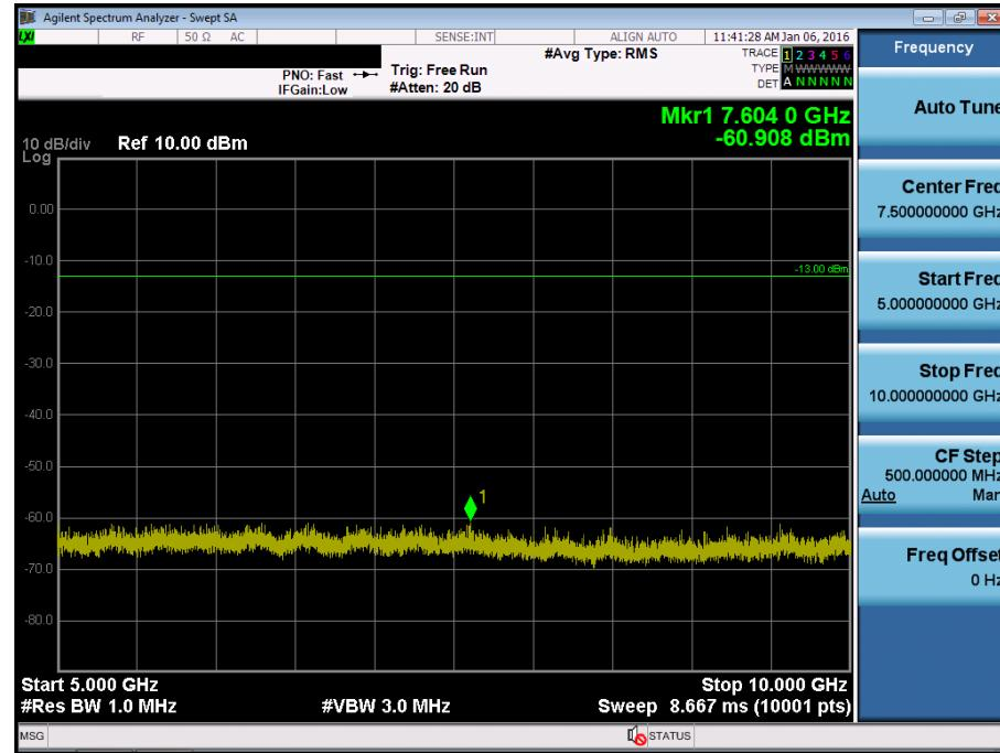
BAND 17. Conducted Spurious Plot\_1 (23825ch\_5MHz\_QPSK\_RB 1\_0)
