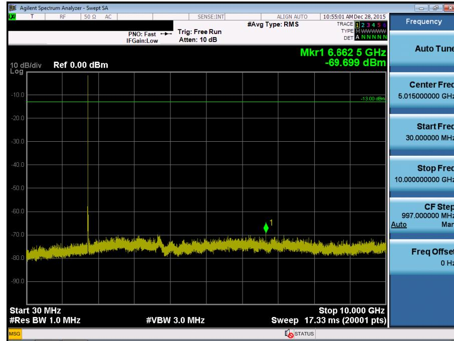
BAND 4. Conducted Spurious Plot\_2 (20175ch\_3MHz\_QPSK\_RB 1\_0)
