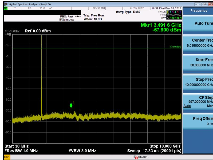
BAND 4. Conducted Spurious Plot\_2 (20350ch\_10MHz\_QPSK\_RB 1\_0)
