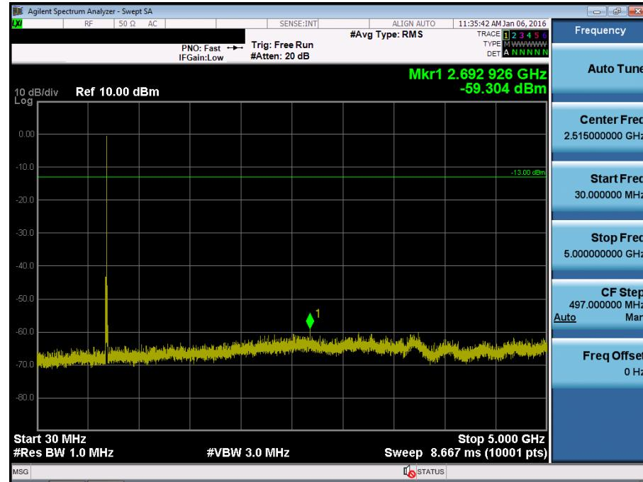
BAND 17. Conducted Spurious Plot\_2 (23790ch\_5MHz\_QPSK\_RB 1\_0)
