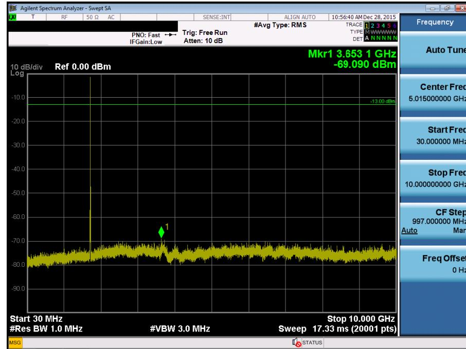
BAND 4. Conducted Spurious Plot\_2 (20175ch\_5MHz\_QPSK\_RB 1\_0)
