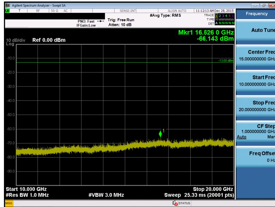
BAND 4. Conducted Spurious Plot\_1 (20375ch\_5MHz\_QPSK\_RB 1\_0)
