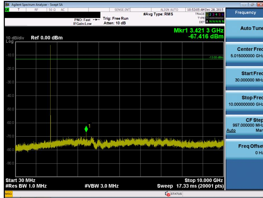
BAND 4. Conducted Spurious Plot\_2 (19957ch\_1.4MHz\_QPSK\_RB 1\_0)
