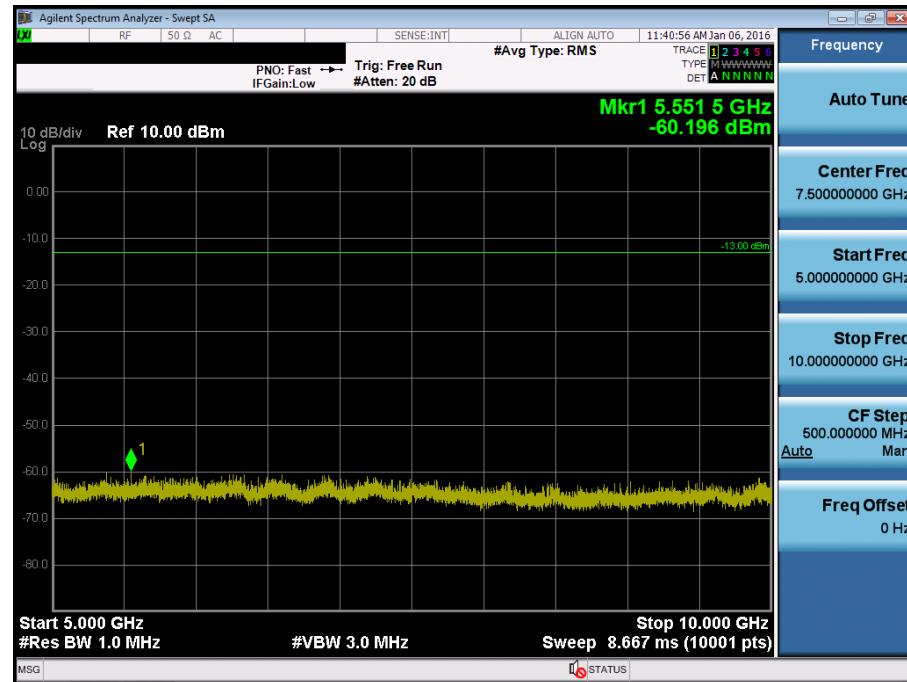
BAND 17. Conducted Spurious Plot\_1 (23780ch\_10MHz\_QPSK\_RB 1\_0)
