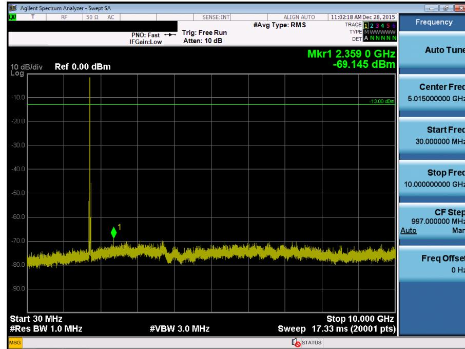
BAND 4. Conducted Spurious Plot\_2 (20175ch\_15MHz\_QPSK\_RB 1\_0)
