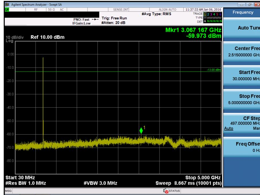
BAND 17. Conducted Spurious Plot\_2 (23790ch\_10MHz\_QPSK\_RB 1\_0)
