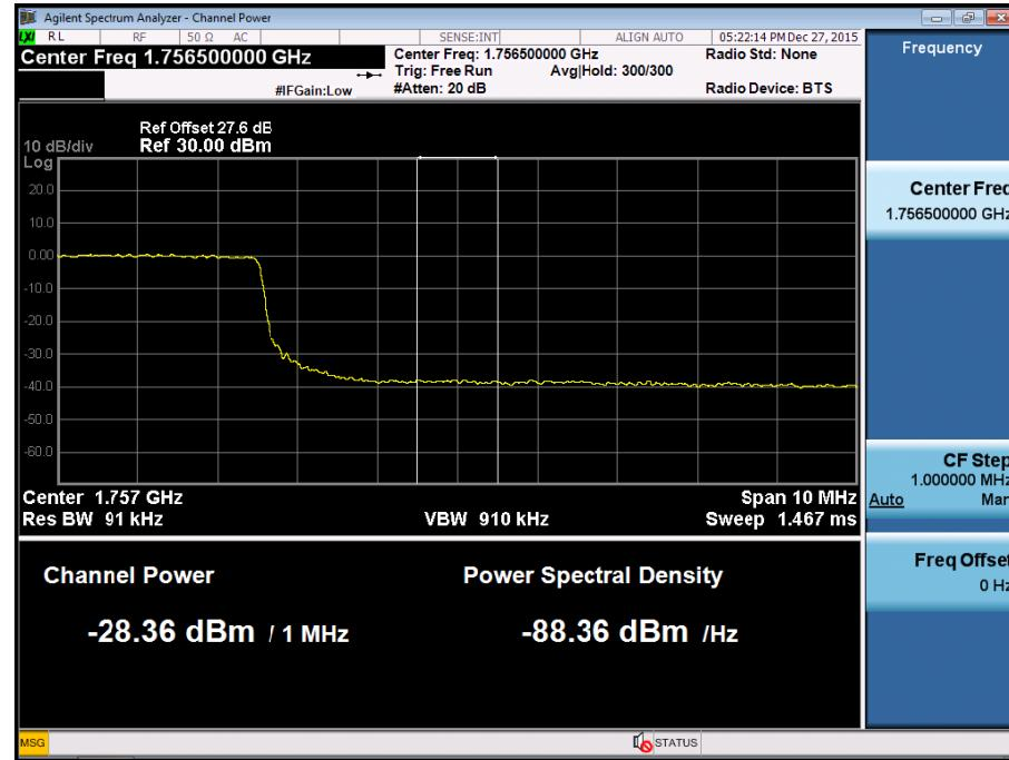
BAND 17. Conducted Spurious Plot\_1 (23755ch\_5MHz\_QPSK\_RB 1\_0)
