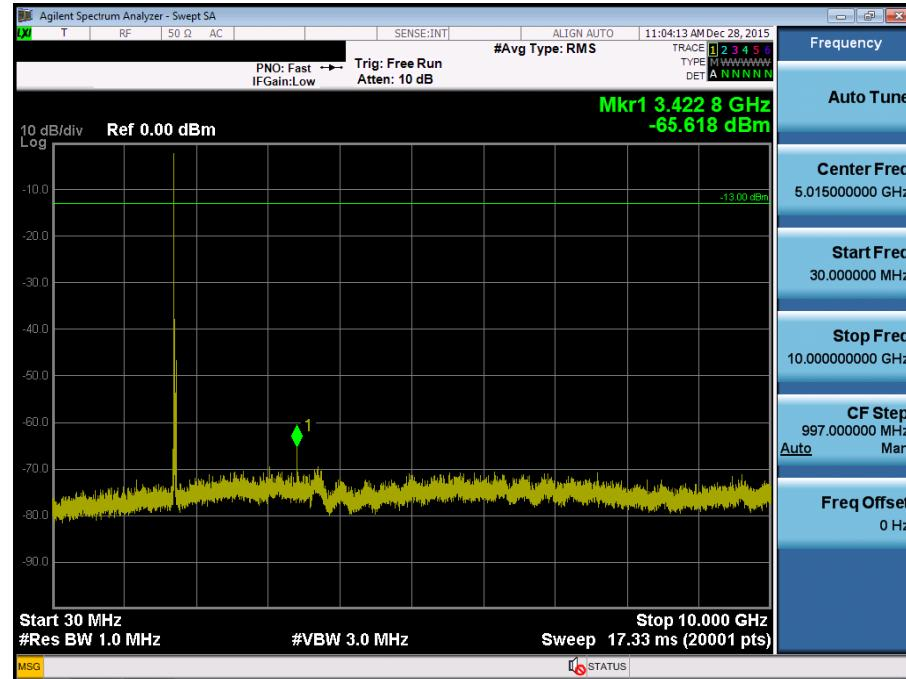
BAND 4. Conducted Spurious Plot\_2 (20050ch\_20MHz\_QPSK\_RB 1\_0)
