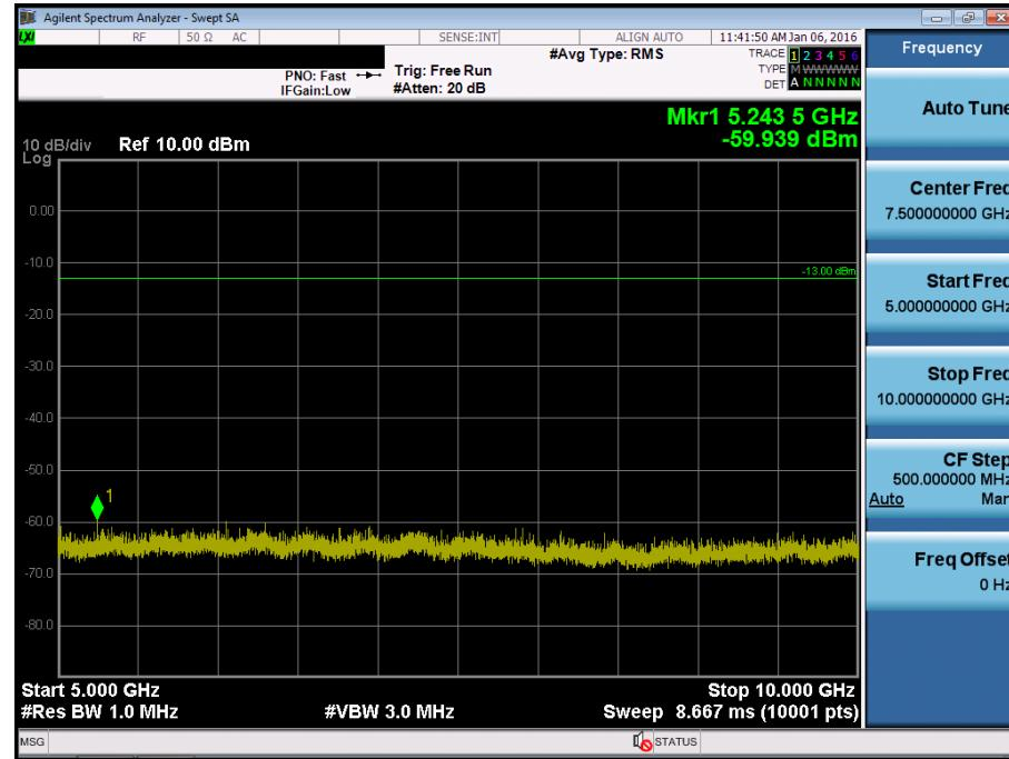
BAND 17. Conducted Spurious Plot\_1 (23790ch\_5MHz\_QPSK\_RB 1\_0)
