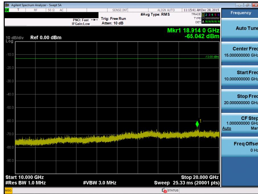
BAND 4. Conducted Spurious Plot\_1 (19965ch\_3MHz\_QPSK\_RB 1\_0)
