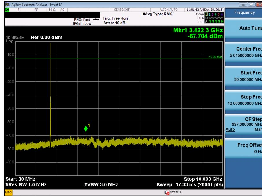
BAND 4. Conducted Spurious Plot\_2 (20025ch\_15MHz\_QPSK\_RB 1\_0)
