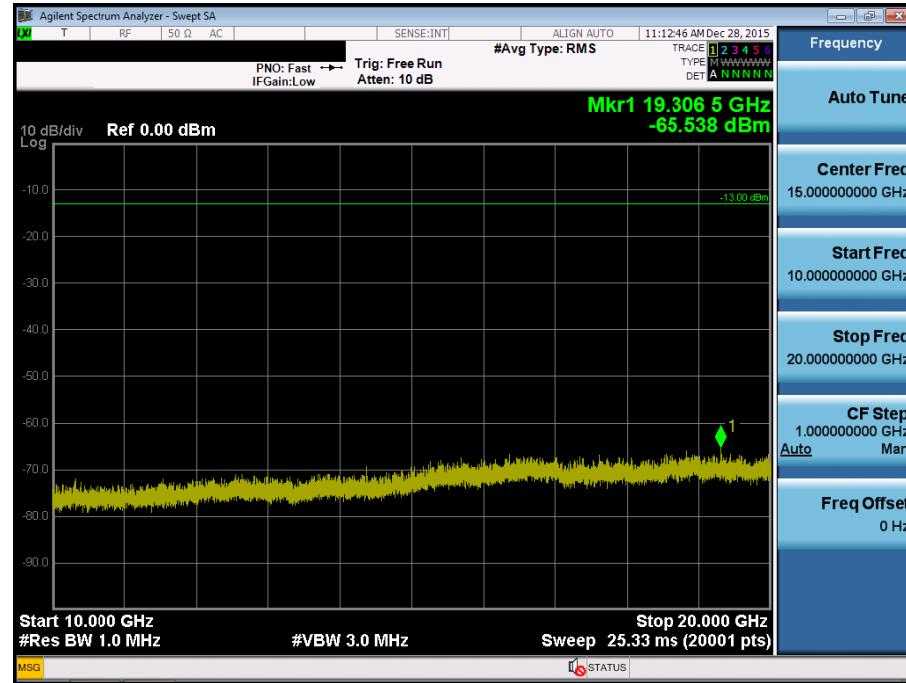
BAND 4. Conducted Spurious Plot\_1 (20175ch\_5MHz\_QPSK\_RB 1\_0)
