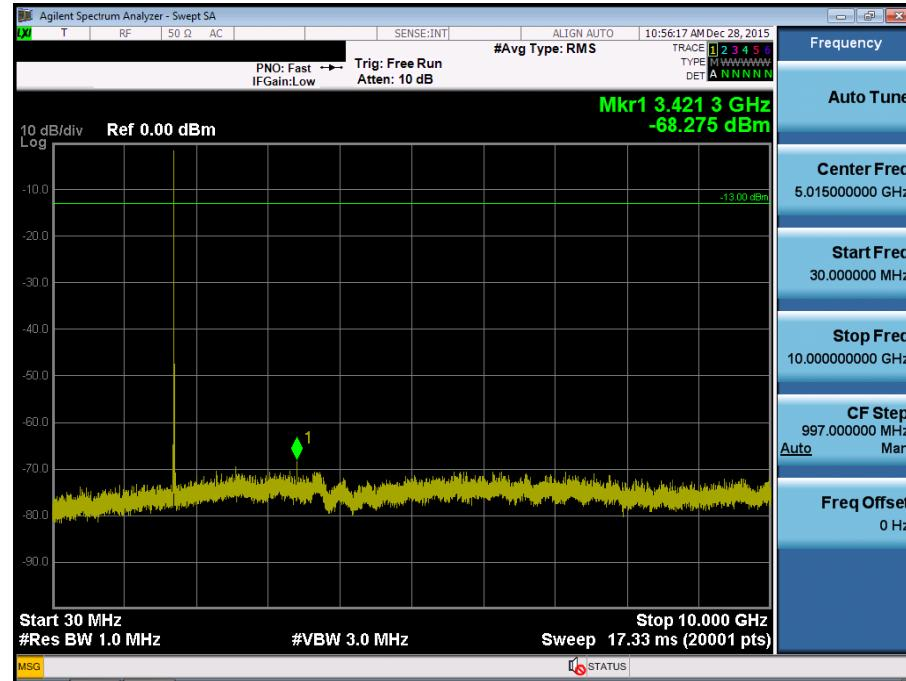
BAND 4. Conducted Spurious Plot\_2 (19975ch\_5MHz\_QPSK\_RB 1\_0)
