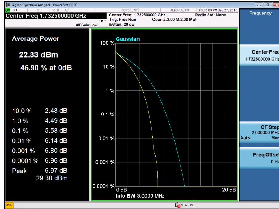
BAND 4. PAR Plot (3M BW\_Ch.20175\_16QAM\_RB15\_0)
