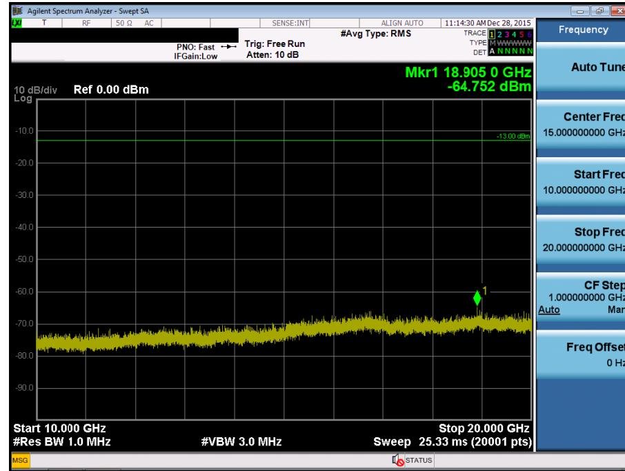
BAND 4. Conducted Spurious Plot\_1 (20385ch\_3MHz\_QPSK\_RB 1\_0)
