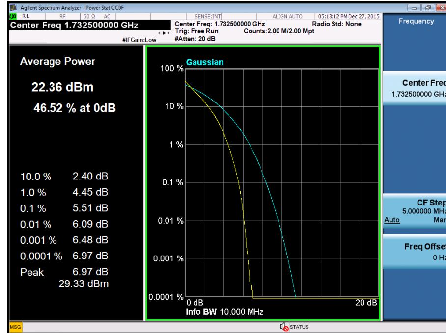
BAND 4. PAR Plot (10M BW\_Ch.20175\_16QAM\_RB50\_0)
