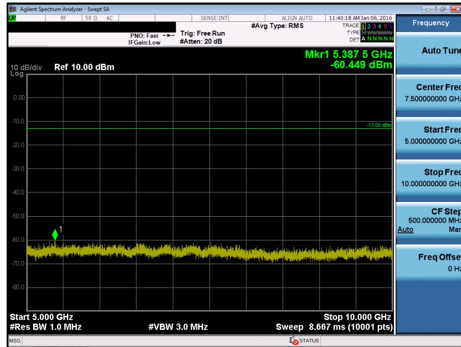
BAND 17. Conducted Spurious Plot\_1 (23790ch\_10MHz\_QPSK\_RB 1\_0)
