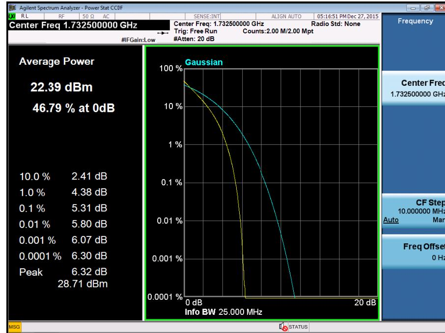
BAND 4. PAR Plot (15M BW\_Ch.20175\_16QAM\_RB75\_0)
