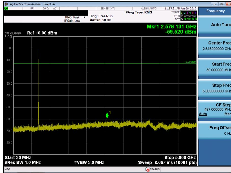
BAND 17. Conducted Spurious Plot\_2 (23755ch\_5MHz\_QPSK\_RB 1\_0)
