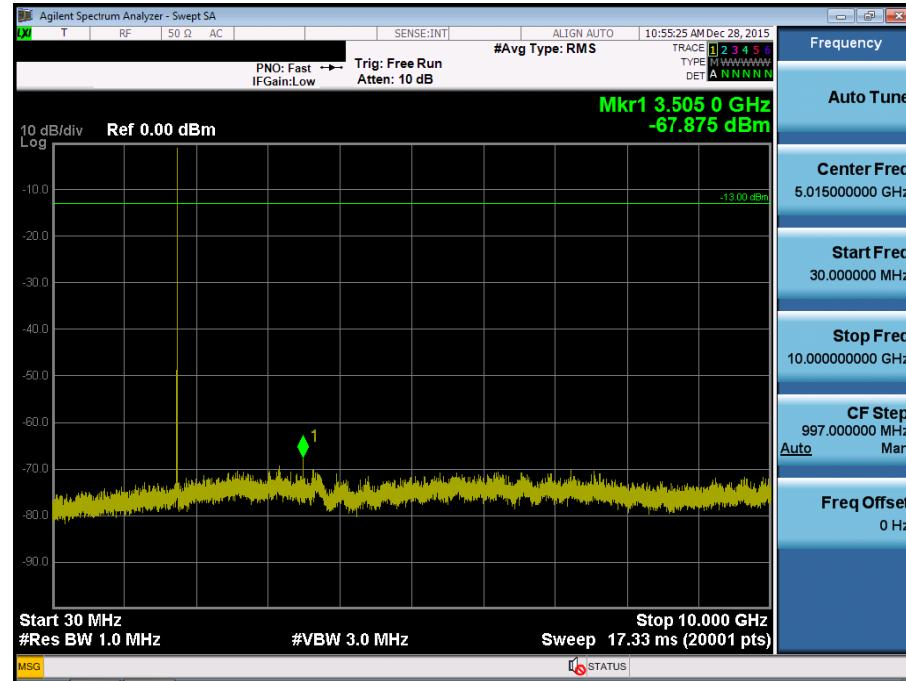
BAND 4. Conducted Spurious Plot\_2 (20385ch\_3MHz\_QPSK\_RB 1\_0)
