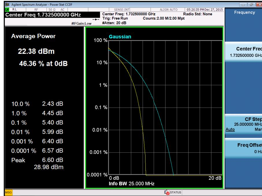
BAND 4. PAR Plot (20M BW\_Ch.20175\_16QAM\_RB100\_0)
