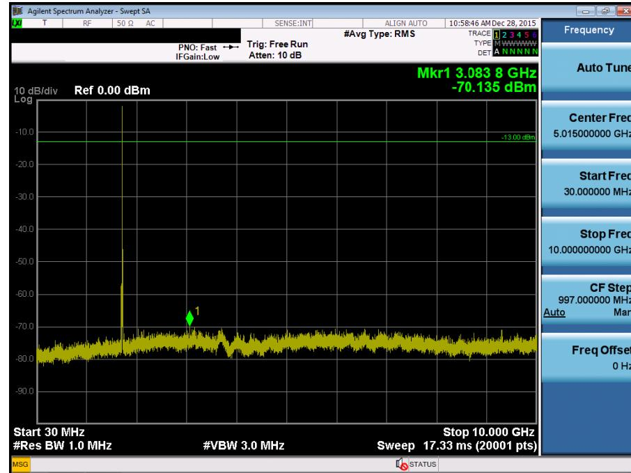
BAND 4. Conducted Spurious Plot\_2 (20175ch\_10MHz\_QPSK\_RB 1\_0)
