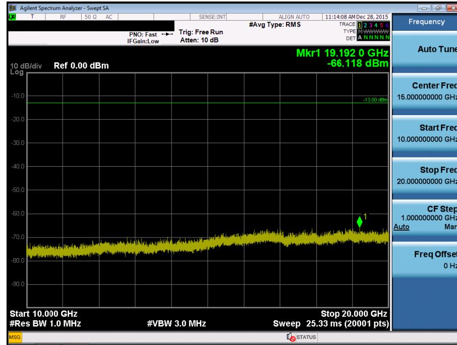
BAND 4. Conducted Spurious Plot\_1 (19975ch\_5MHz\_QPSK\_RB 1\_0)
