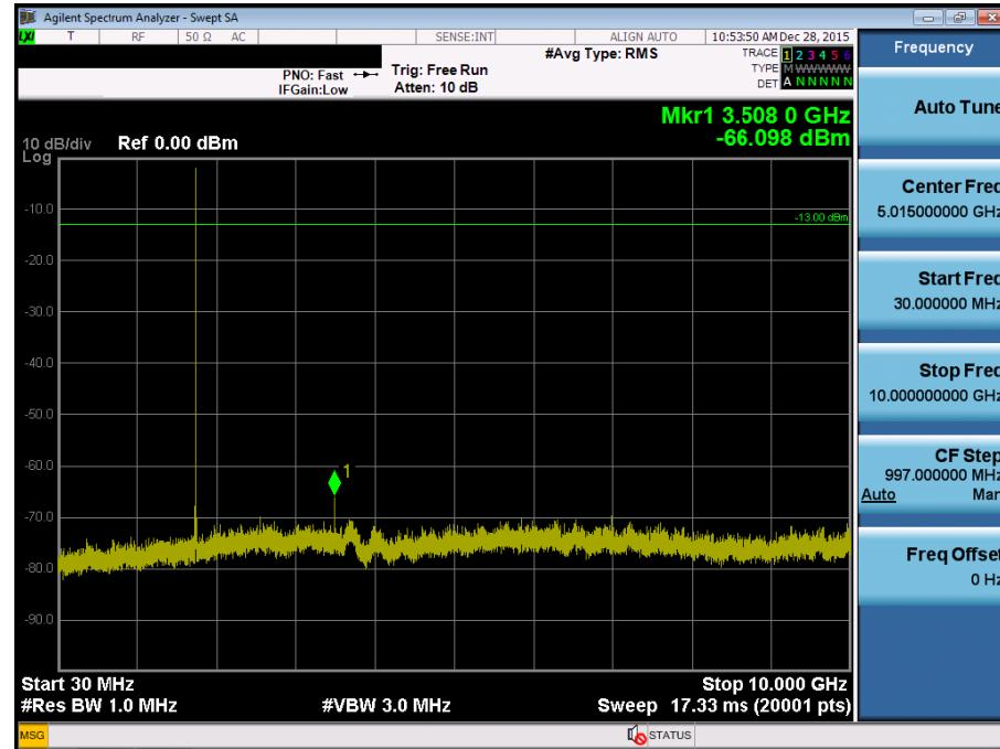
BAND 4. Conducted Spurious Plot\_2 (20393ch\_1.4MHz\_QPSK\_RB 1\_0)
