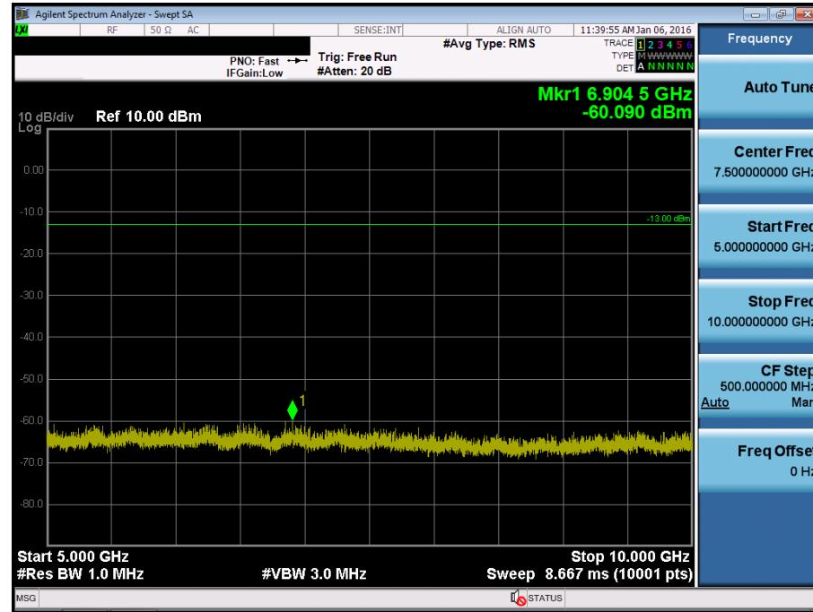
BAND 17. Conducted Spurious Plot\_1 (23800ch\_10MHz\_QPSK\_RB 1\_0)
