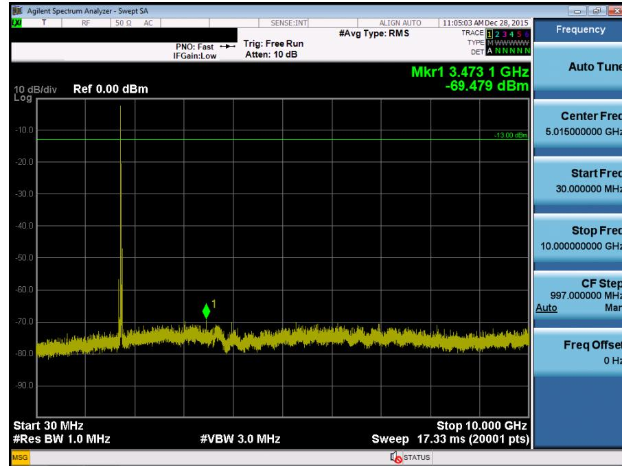
BAND 4. Conducted Spurious Plot\_2 (20300ch\_20MHz\_QPSK\_RB 1\_0)
