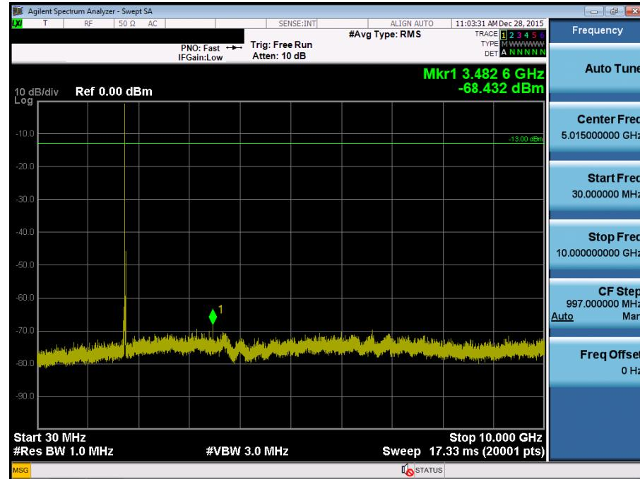
BAND 4. Conducted Spurious Plot\_2 (20325ch\_15MHz\_QPSK\_RB 1\_0)
