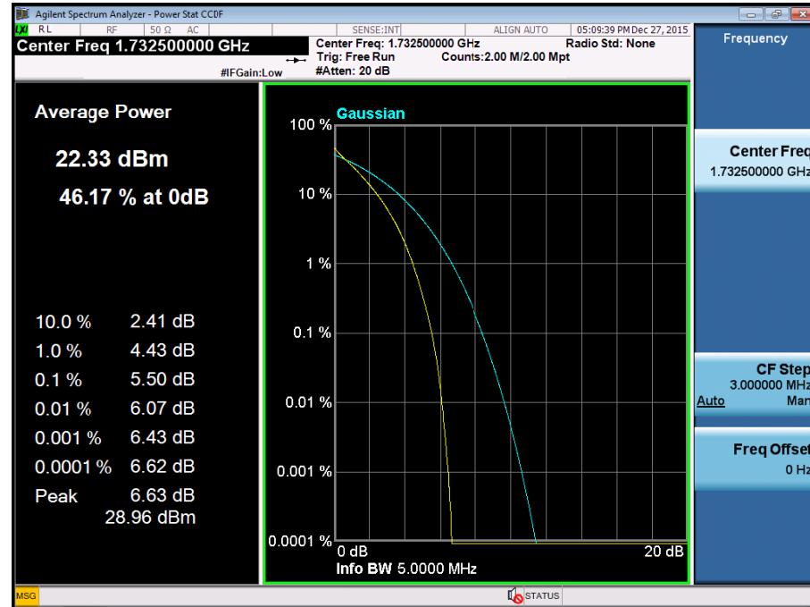
BAND 4. PAR Plot (5M BW\_Ch.20175\_16QAM\_RB25\_0)
