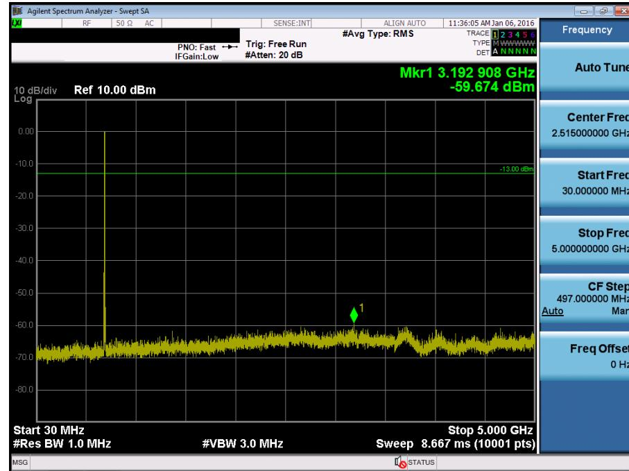
BAND 17. Conducted Spurious Plot\_2 (23825ch\_5MHz\_QPSK\_RB 1\_0)
