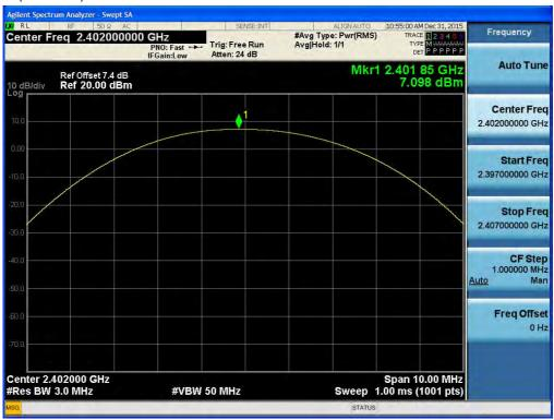
Test Plots (GFSK) Peak Power (Mid-CH)
