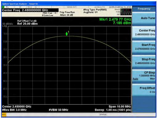
Test Plots (8DPSK) Peak Power (Low-CH)
