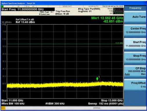
Test Plots (GFSK)- 13 GHz - 15 GHz Spurious Emission (High-CH)
