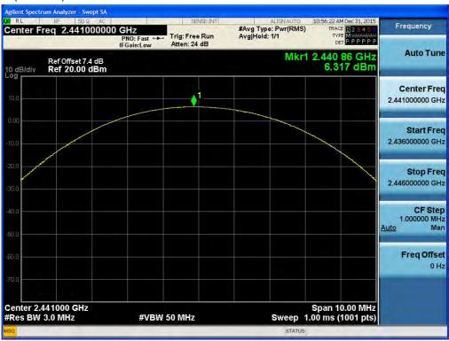
Test Plots (8DPSK) Peak Power (High-CH)
