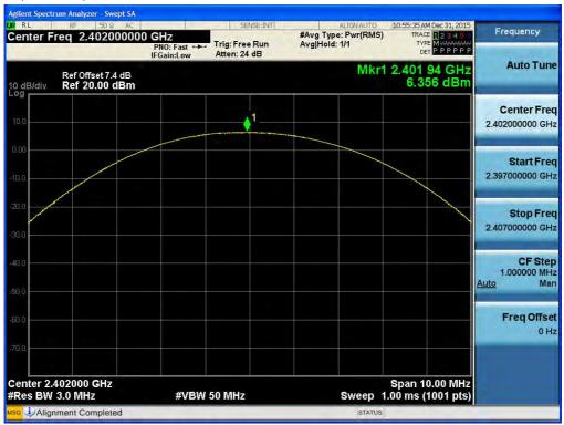
Test Plots (π/4DQPSK) Peak Power (Mid-CH)
