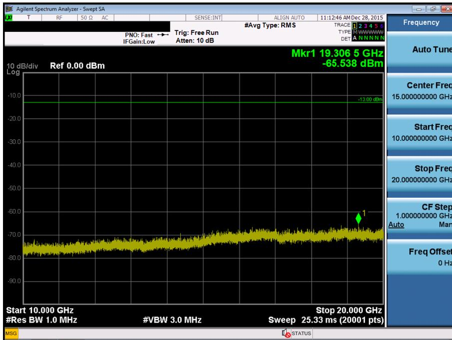
BAND 4. Conducted Spurious Plot\_1 (20175ch\_5MHz\_QPSK\_RB 1\_0)
