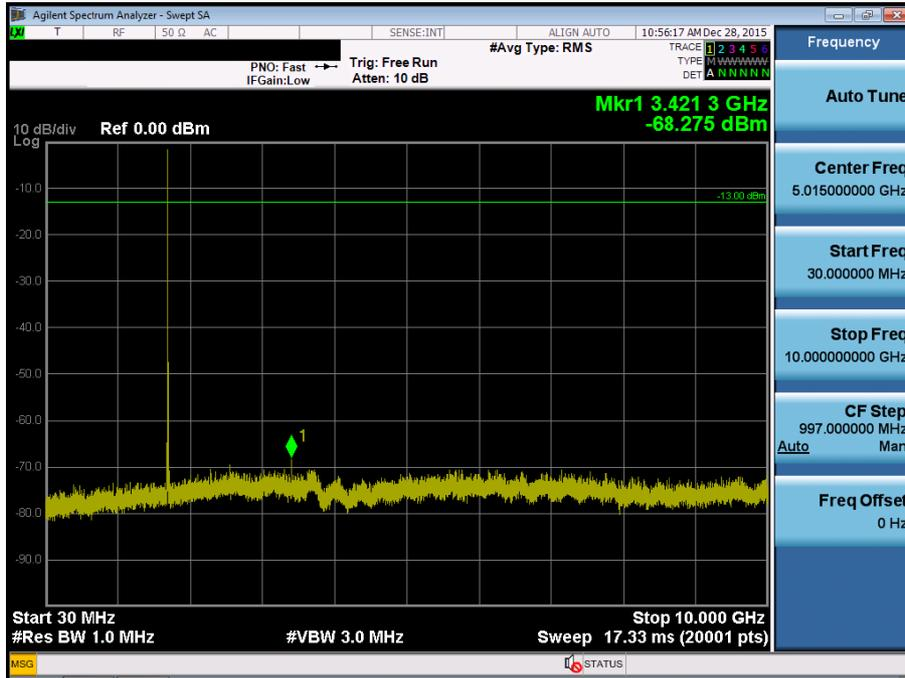
BAND 4. Conducted Spurious Plot\_2 (19975ch\_5MHz\_QPSK\_RB 1\_0)
