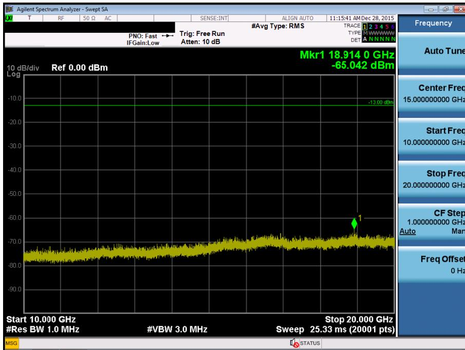
BAND 4. Conducted Spurious Plot\_1 (19965ch\_3MHz\_QPSK\_RB 1\_0)
