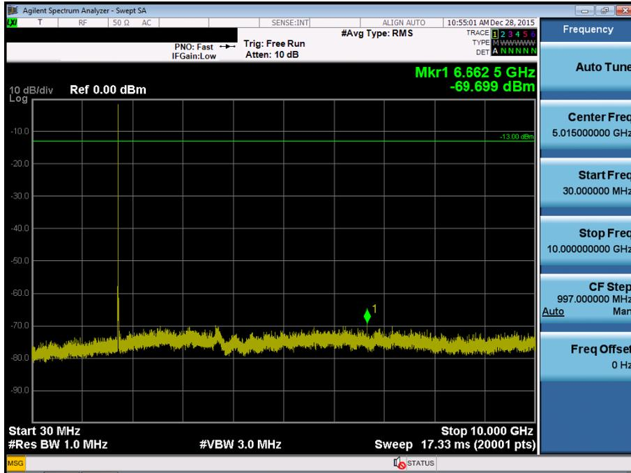
BAND 4. Conducted Spurious Plot\_2 (20175ch\_3MHz\_QPSK\_RB 1\_0)
