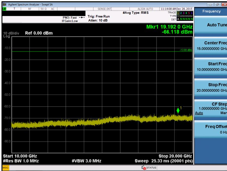
BAND 4. Conducted Spurious Plot\_1 (19975ch\_5MHz\_QPSK\_RB 1\_0)
