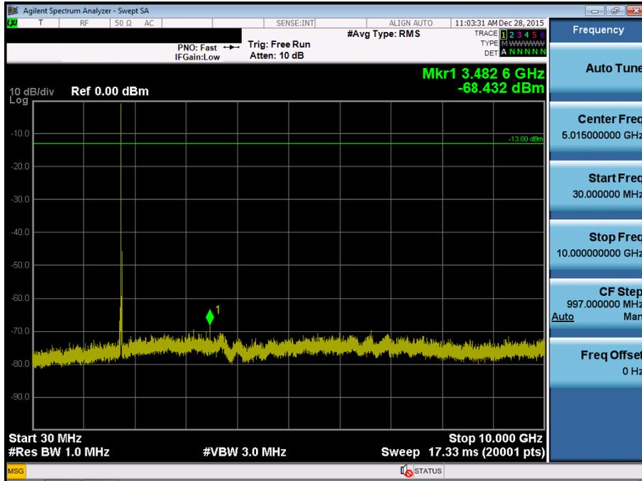
BAND 4. Conducted Spurious Plot\_2 (20325ch\_15MHz\_QPSK\_RB 1\_0)
