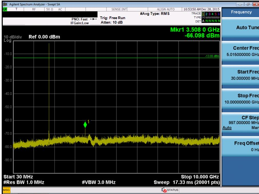
BAND 4. Conducted Spurious Plot\_2 (20393ch\_1.4MHz\_QPSK\_RB 1\_0)
