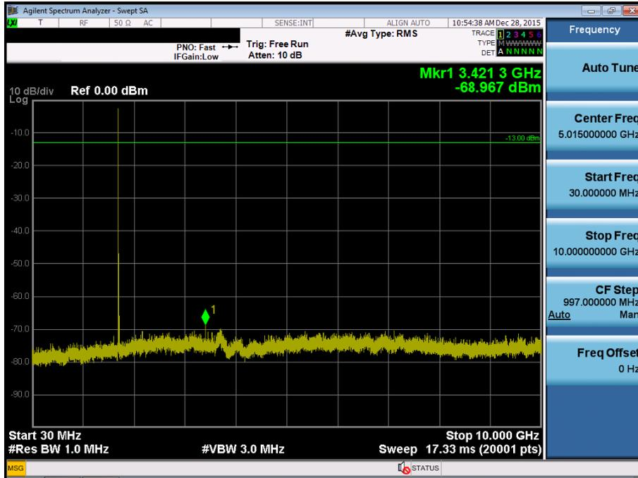
BAND 4. Conducted Spurious Plot\_2 (19965ch\_3MHz\_QPSK\_RB 1\_0)
