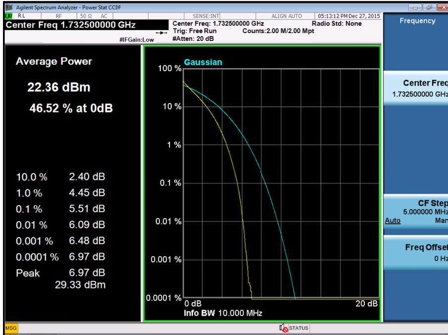
BAND 4. PAR Plot (10M BW\_Ch.20175\_16QAM\_RB50\_0)
