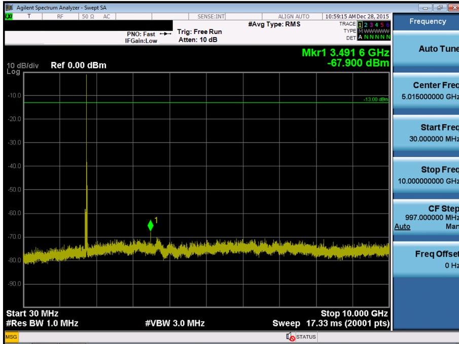
BAND 4. Conducted Spurious Plot\_2 (20350ch\_10MHz\_QPSK\_RB 1\_0)
