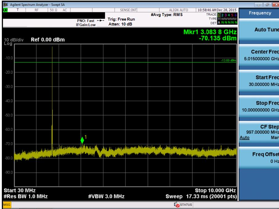
BAND 4. Conducted Spurious Plot\_2 (20175ch\_10MHz\_QPSK\_RB 1\_0)
