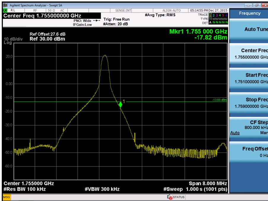
BAND 4. Upper Band Edge Plot (10M BW Ch.20350 QPSK\_RB50) -2
