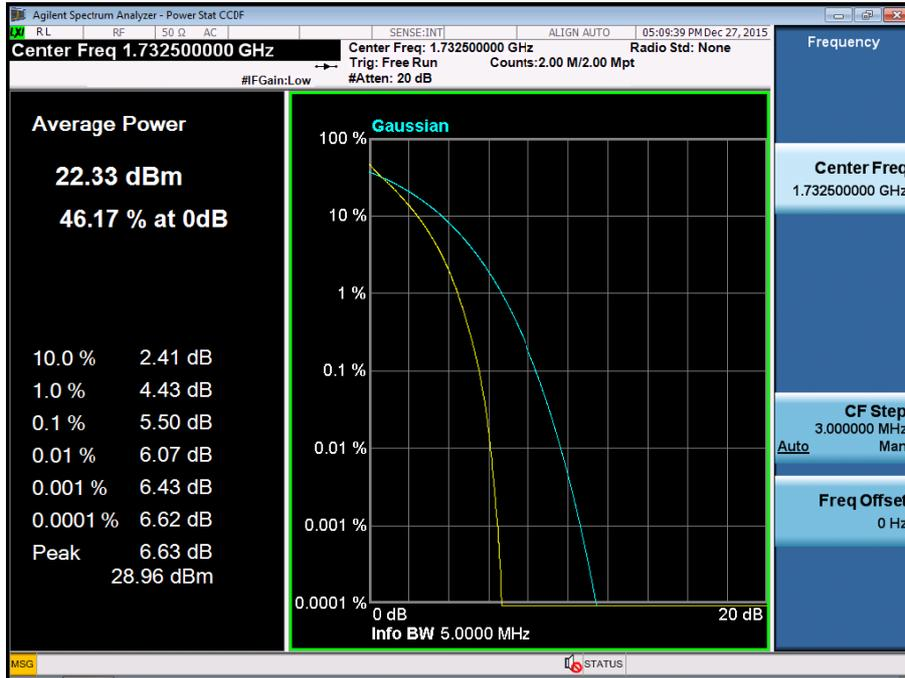
BAND 4. PAR Plot (5M BW\_Ch.20175\_16QAM\_RB25\_0)
