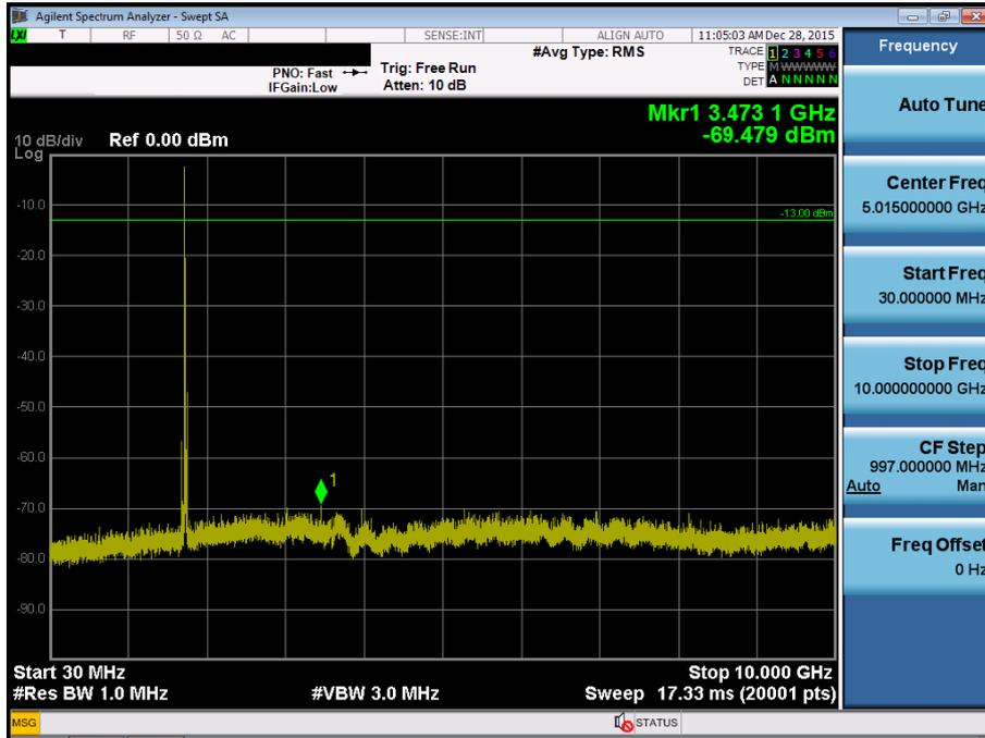
BAND 4. Conducted Spurious Plot\_2 (20300ch\_20MHz\_QPSK\_RB 1\_0)
