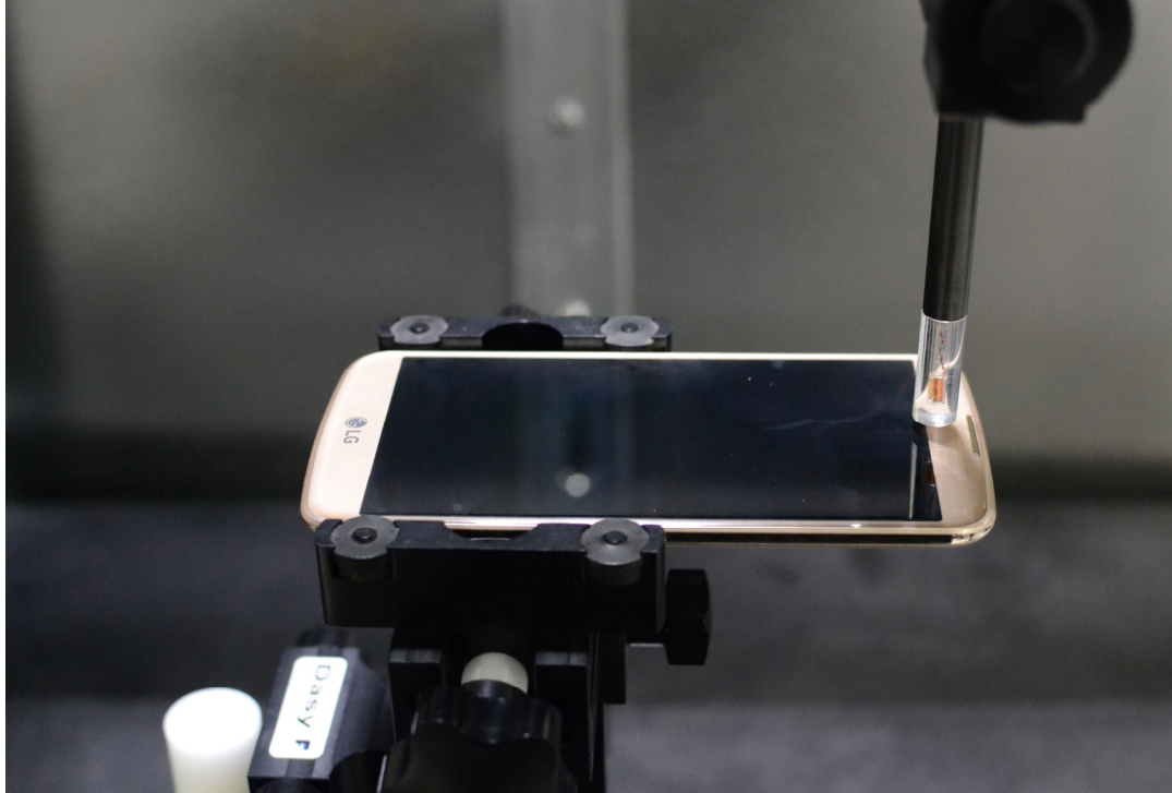
Figure 14-1 Test Setup for Wireless Device
