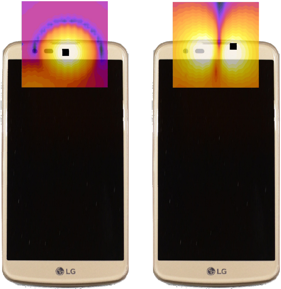
Figure 14-3 T-Coil Scan Overlay Magnetic Field Distributions
