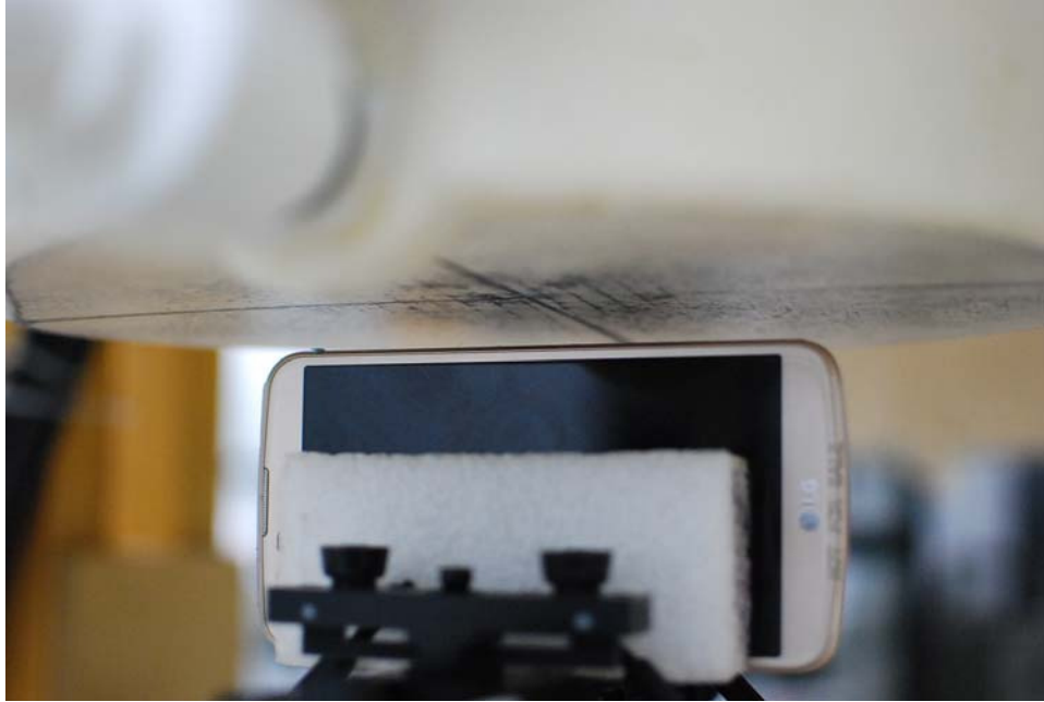
SAR Test Setup Photo 9 – Right Edge (10 mm)
