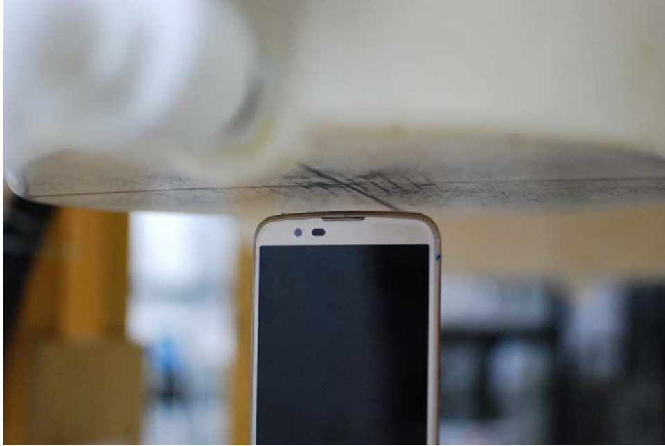
SAR Test Setup Photo 7 – Top Edge (10 mm)
