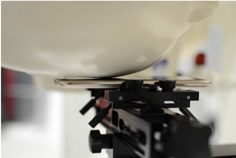
SAR Test Setup Photo 1 – Right Cheek
