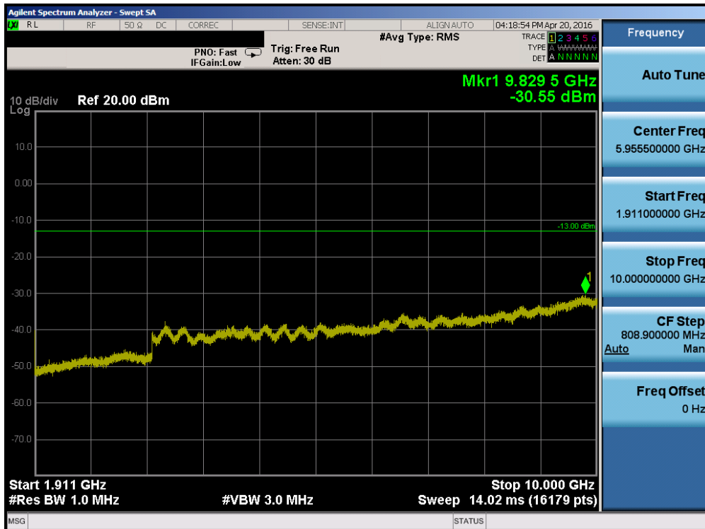
Plot 7-66. Conducted Spurious Plot (Band 2 – 20.0MHz QPSK – RB Size 1, RB Offset 0 – High Channel)
