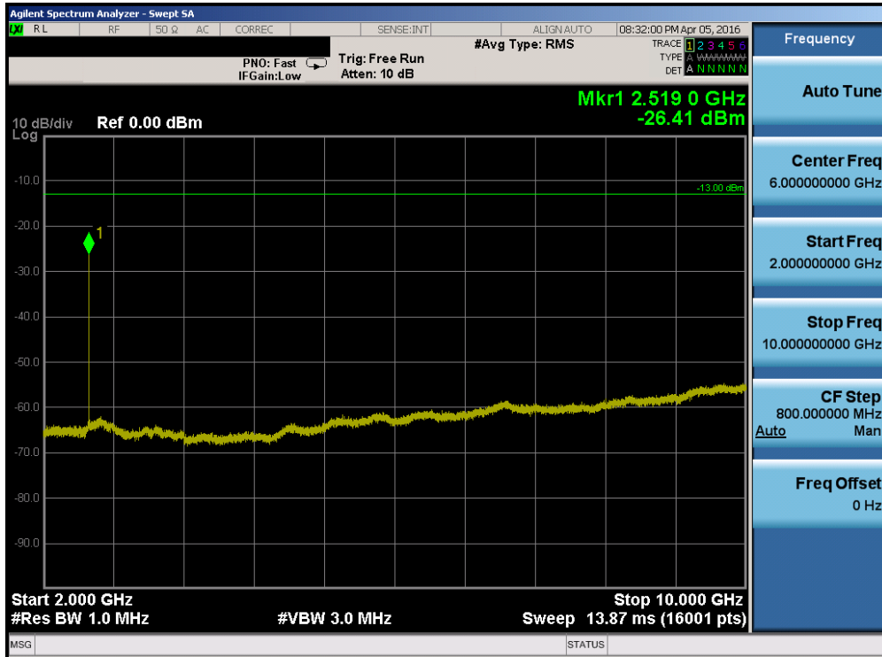
Plot 7-58. Conducted Spurious Plot (Band 5 – 10.0MHz QPSK – RB Size 1, RB Offset 0 – High Channel)
