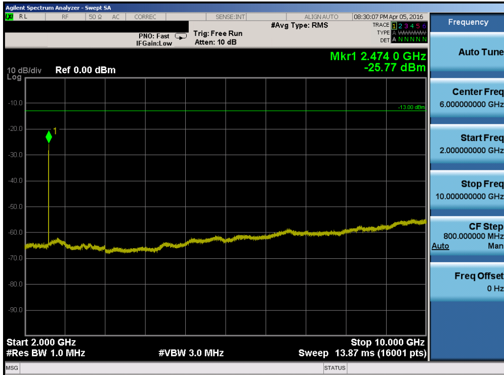
Plot 7-52. Conducted Spurious Plot (Band 5 – 10.0MHz QPSK – RB Size 1, RB Offset 0 – Low Channel)
