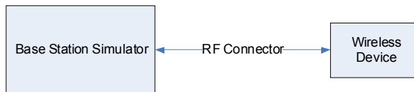
Figure 9-1 Power Measurement Setup
