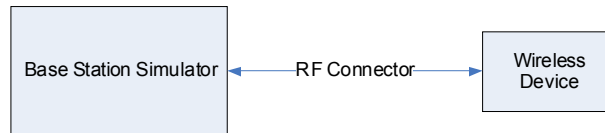
Figure 9-2 Power Measurement Setup
