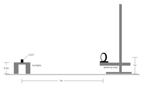
Figure 7-2. Radiated Test Setup < 30Mhz
