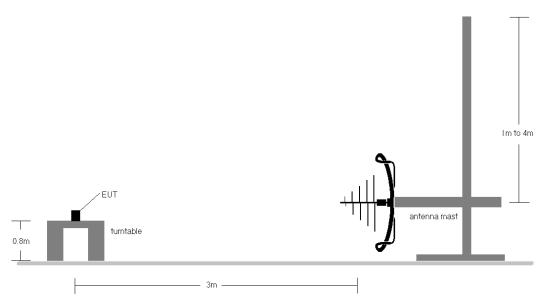
Figure 7-3. Radiated Test Setup < 1GHz
