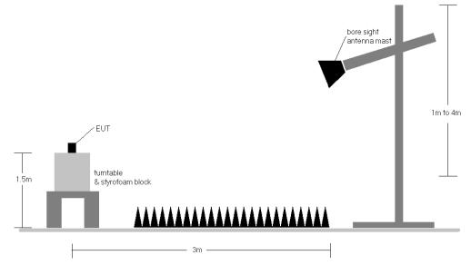
Figure 7-1. Radiated Test Setup >1GHz
