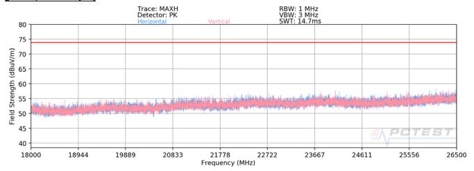
Plot 7-4. Radiated Spurious Plot above 18GHz
