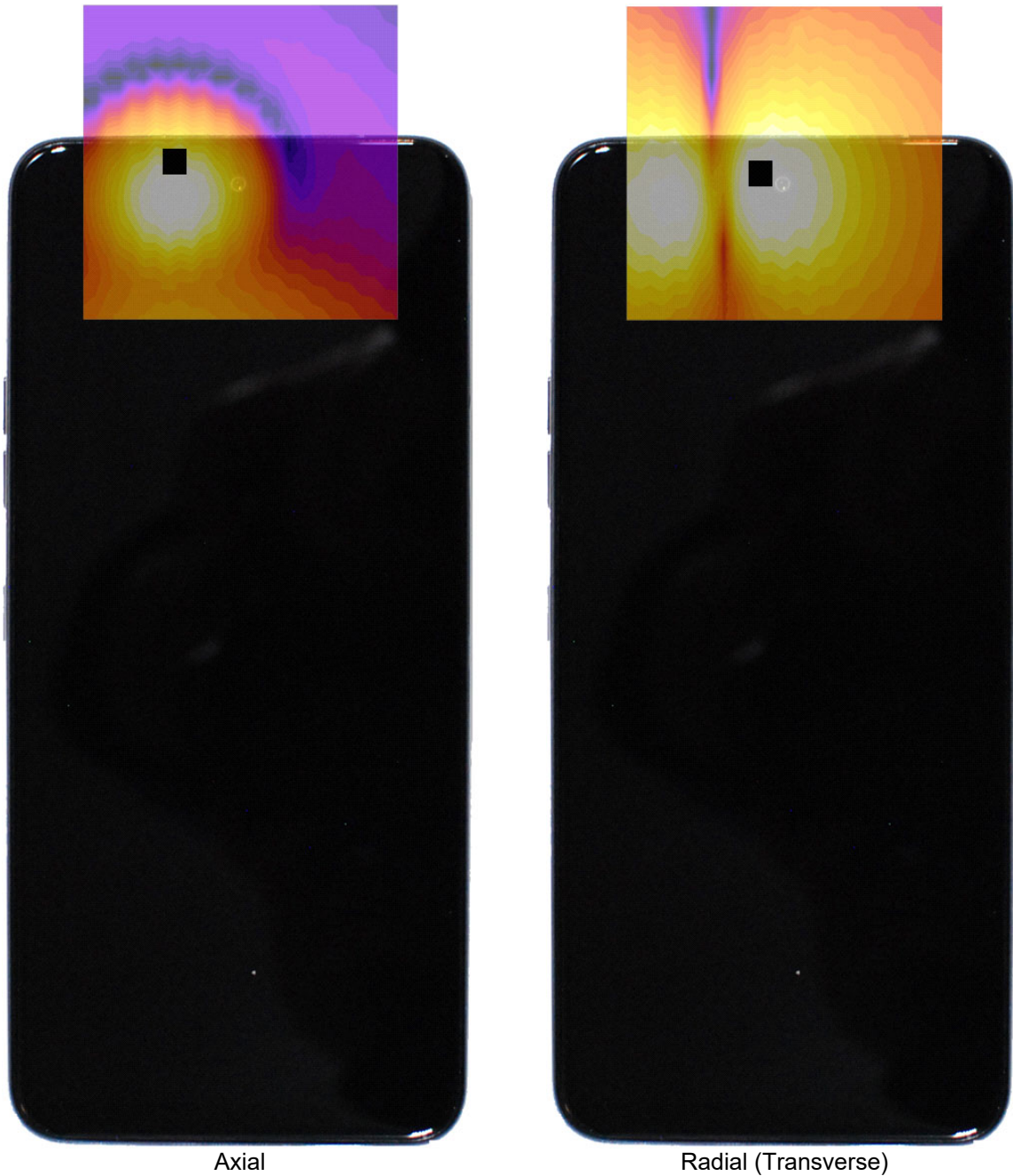
Figure 16-3 T-Coil Scan Overlay Magnetic Field Distributions
