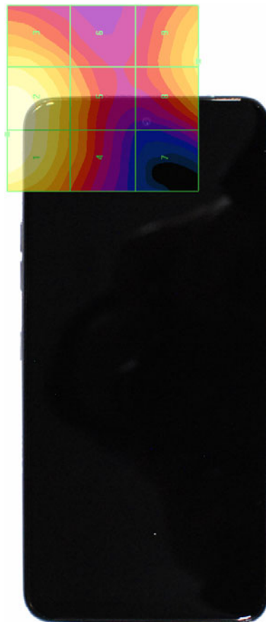
Figure 18-4 E-Field WD Scan overlay (T-Coil Centered scan area pictured)
