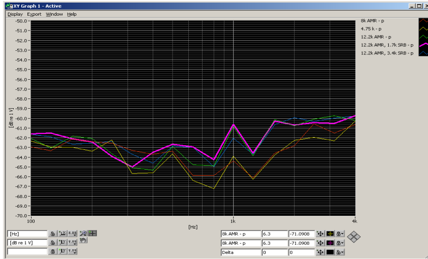
Figure 8-3 UMTS Audio Band Magnetic Noise
