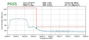
Plot 7-16. Radiated Upper Band Edge Plot (Peak – UNII Band 2A)
