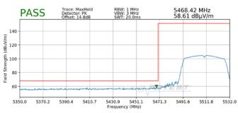
Plot 7-18. Radiated Lower Band Edge Plot (Peak – UNII Band 2C)
