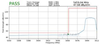
Plot 7-10. Radiated Lower Band Edge Plot (Average – UNII Band 2C)
