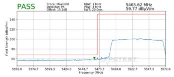
Plot 7-25. Radiated Lower Band Edge Plot (Peak – UNII Band 2C)
