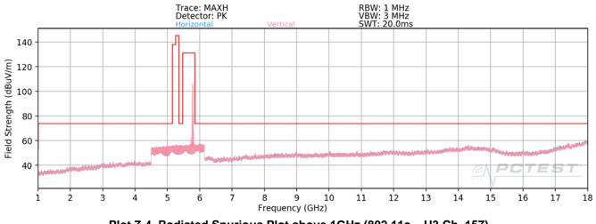
Plot 7-4. Radiated Spurious Plot above 1GHz (802.11a - U3 Ch. 157)
