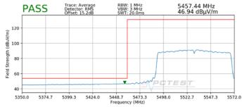
Plot 7-24. Radiated Lower Band Edge Plot (Average – UNII Band 2C)
