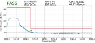
Plot 7-9. Radiated Upper Band Edge Plot (Peak – UNII Band 2A)
