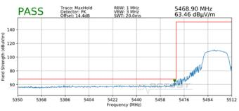
Plot 7-11. Radiated Lower Band Edge Plot (Peak – UNII Band 2C)
