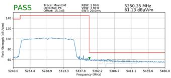
Plot 7-23. Radiated Upper Band Edge Plot (Peak – UNII Band 2A)
