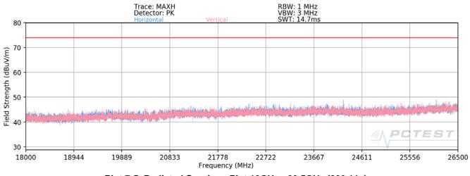
Plot 7-5. Radiated Spurious Plot 18GHz - 26.5GHz (802.11a)
