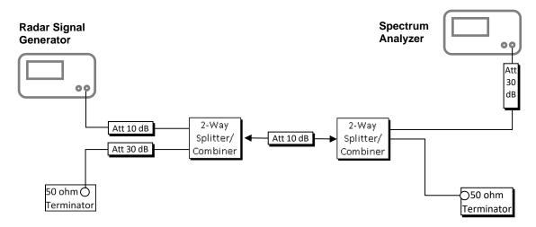
Figure 7-2. Radar Waveform Calibration
