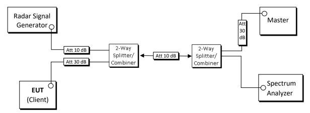
Figure 7-1. Conducted Test Setup for DFS
