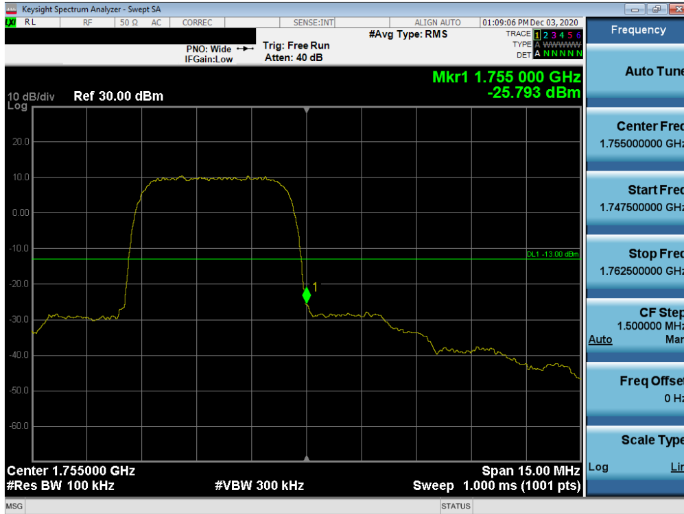
Plot 7-151. Upper Band Edge Plot (WCDMA AWS – Ch. 1513)
