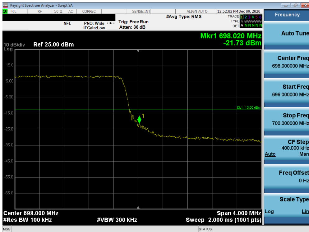
Plot 7-148. Upper Band Edge Plot (LTE Band 71 - 5MHz QPSK – Full RB Configuration)
