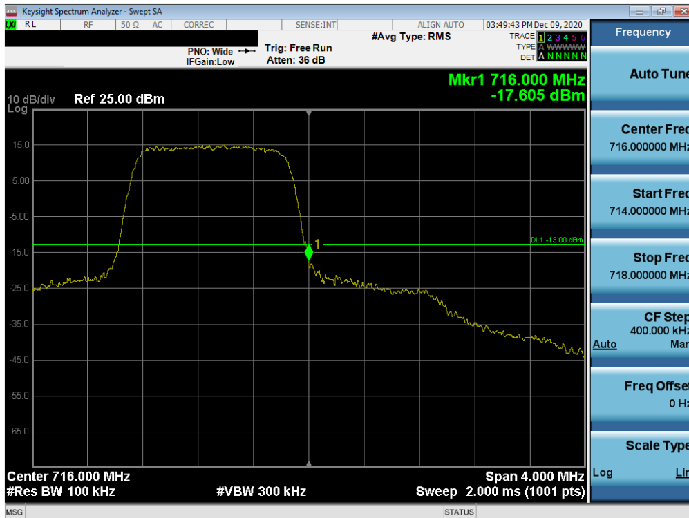
Plot 7-132. Upper Band Edge Plot (LTE Band 12 – 1.4MHz QPSK – Full RB Configuration)
