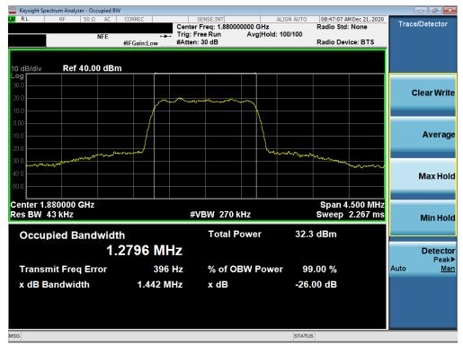
Plot 7-22. Occupied Bandwidth Plot (CDMA, Ch. 600)
