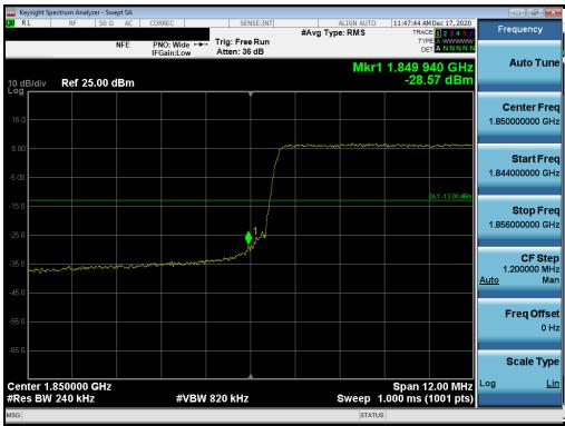
Plot 7-65. Lower Band Edge Plot (LTE Band 25/2 - 15MHz QPSK - Full RB Configuration)
