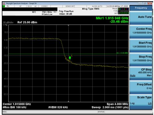
Plot 7-81. Upper Band Edge Plot (LTE Band 25 - 5MHz QPSK - Full RB Configuration)
