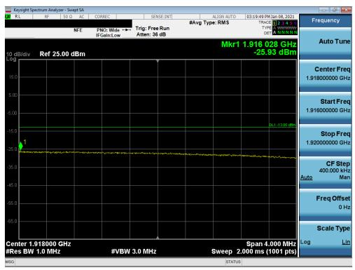
Plot 7-64. Extended Upper Band Edge Plot (LTE Band 25 - 20MHz QPSK - Full RB Configuration)
