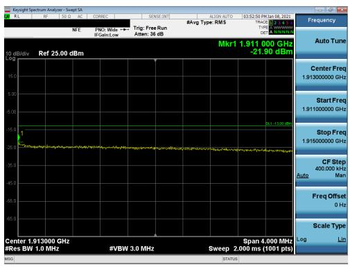
Plot 7-74. Extended Upper Band Edge Plot (LTE Band 2 - 10MHz QPSK - Full RB Configuration)
