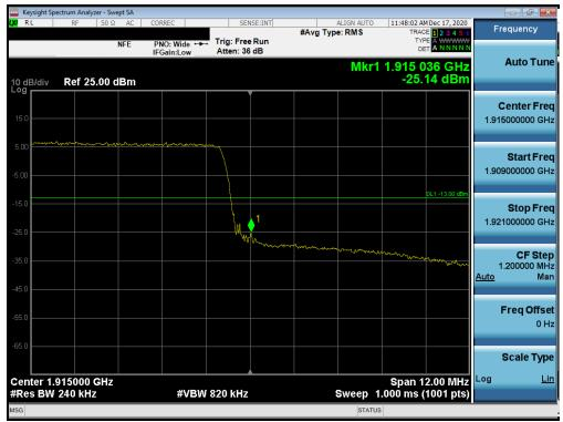
Plot 7-69. Upper Band Edge Plot (LTE Band 25 - 15MHz QPSK - Full RB Configuration)
