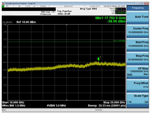
Plot 7-34. Conducted Spurious Plot (GPRS Ch. 512)
