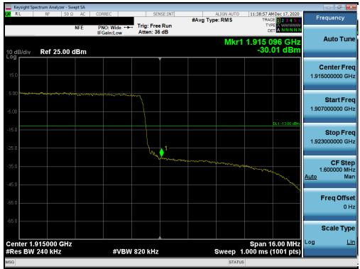
Plot 7-63. Upper Band Edge Plot (LTE Band 25 - 20MHz QPSK - Full RB Configuration)
