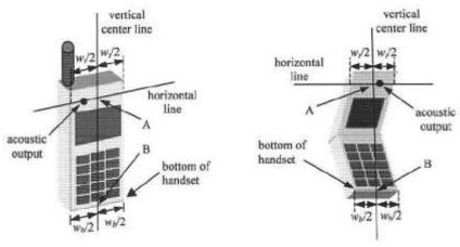
Figure 6-3. Handset vertical and horizontal reference lines
