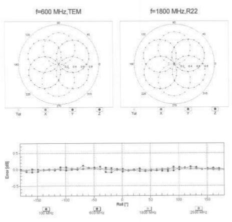
Receiving Pattern ( $\phi$ ),  $\vartheta = 0^{\circ}$
