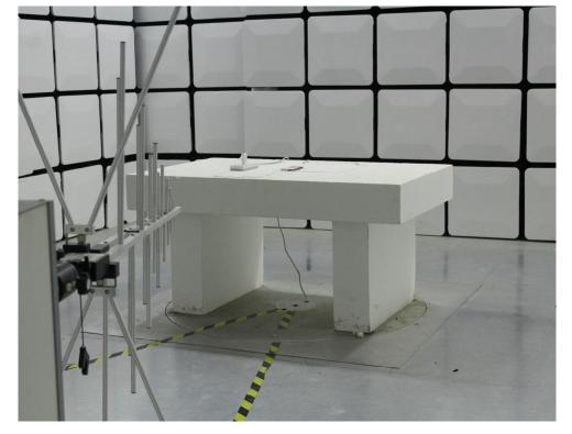
**1.2** Setup for Unwanted Emissions that fall Outside of the Restricted Bands(Radiated) and Unwanted Emissions in the Restricted Bands (Radiated) below 1GHz
