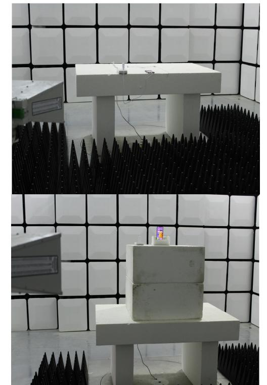
**1.3** Setup for Unwanted Emissions that fall Outside of the Restricted Bands(Radiated) and Unwanted Emissions in the Restricted Bands (Radiated) above 1GHz
